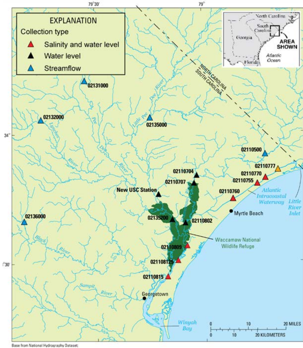
Figure 6. The existing water level, temperature, and salinity stations in PRISM-2 and those that would be used to develop the PRISM-3 Decision Support System and the current acquisition boundary of the Waccamaw National Wildlife Refuge (dark green).
