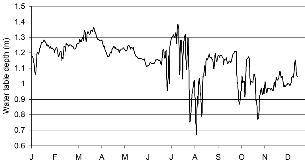
Figure 3.3 – Interpreted water table elevations at Minnow east well used for total soil water evaporation model application (2006).
