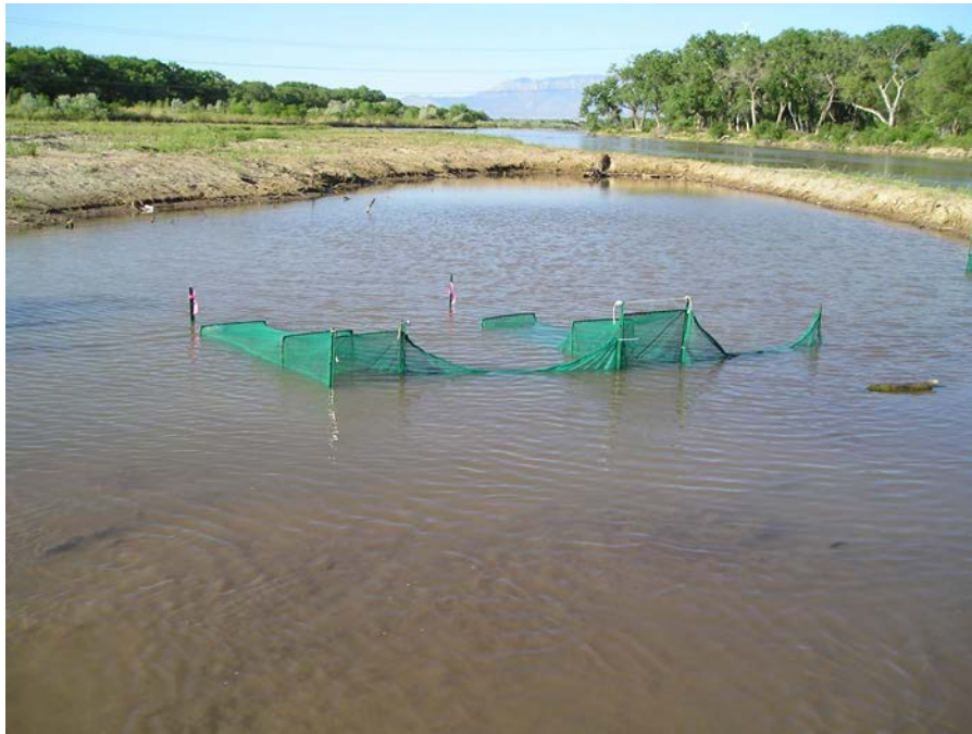
Figure A.4. Westernmost set-up at South Diversion Channel. A medial sandbar has been deposited across the mouth of the embayment, and the water becomes substantially deeper behind the hoop nets.
