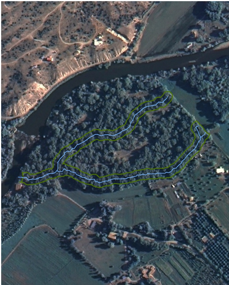
Aerial photograph of channel locations within the proposed Los Luceros restoration site. The total combined channel length is approximately 4,011 feet. The blue lines depict the channel. The green lines represent the widths on either side (50 feet on either side) of the channels where Russian olives would be removed and replaced with dense willow plantings.
