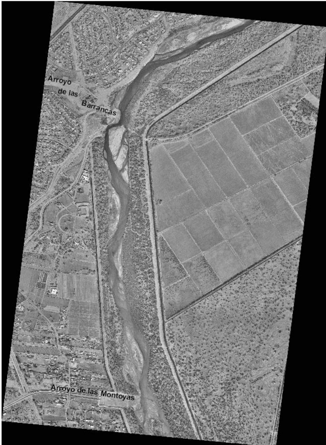
Figure 12. Visible channel planform transition zone from a single-threaded, locally island-braided channel with a deep, fast flowing thalweg (upstream of Barrancas Arroyo) undergoes a transition into a wider, multi-threaded, island and bar-braided channel with shallow, slower-flowing multiple thalwegs (downstream of Montoyas Arroyo).
