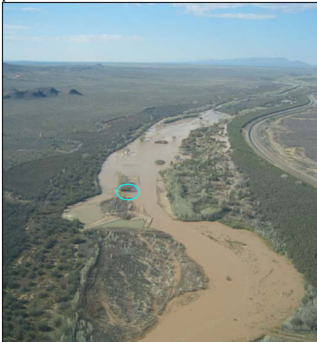
Figure 15. The Bosque del Apache NWR Channel Widening Project area in April 2004 with 2,800 cfs flowing in the Rio Grande. Inlet #1 is circled in red. Photo from River Analysis Archives.
