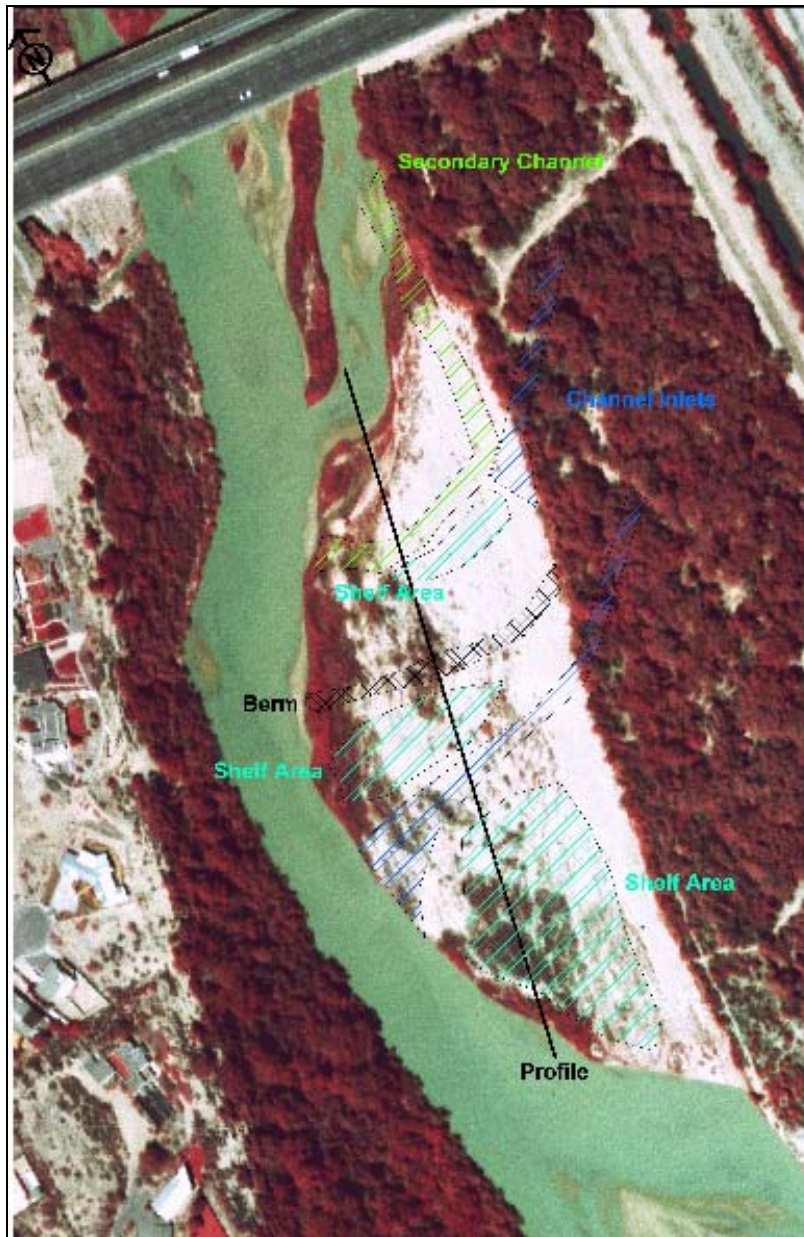
Figure 19. Sketched modifications to a point bar on the Rio Grande immediately downstream of Interstate-40 bridge crossing. The modifications shown include: 1) introduction of a side channel into the bar sediments with connected inlet and shelf area; 2) bar-spanning berm to hinder very high Rio Grande flows that overtop the bar; 3) inlets connected to surface runoff channels; and 4) lower bar elevation to create a directly connected shelf area on the downstream section of the bar.
