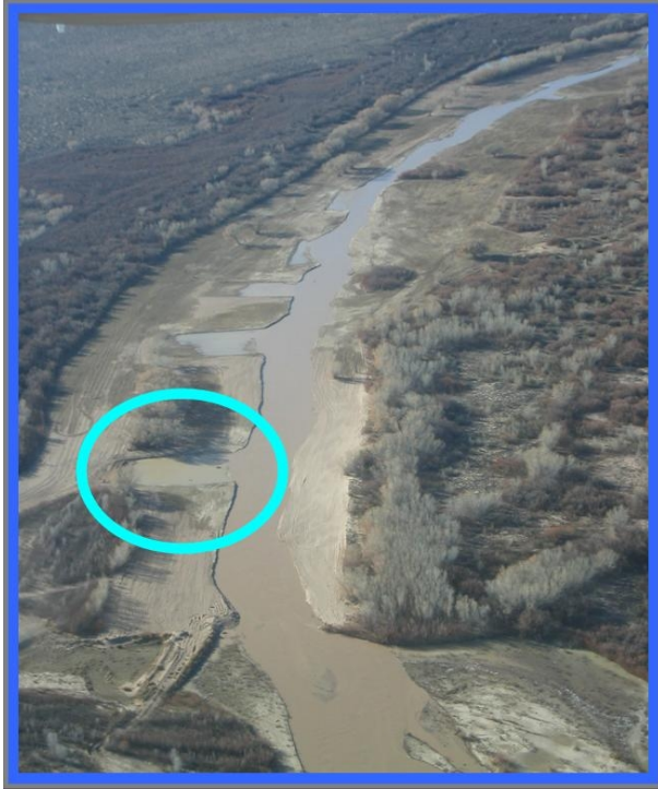
Figure 14. Constructed inlets in the Bosque del Apache NWR Channel Widening Project area in 2003. Inlet #1 is circled in red adjacent to the newly constructed Rio Grande Channel. The previous Rio Grande channel is to the left of the inlets. Photo by R. Doster.
