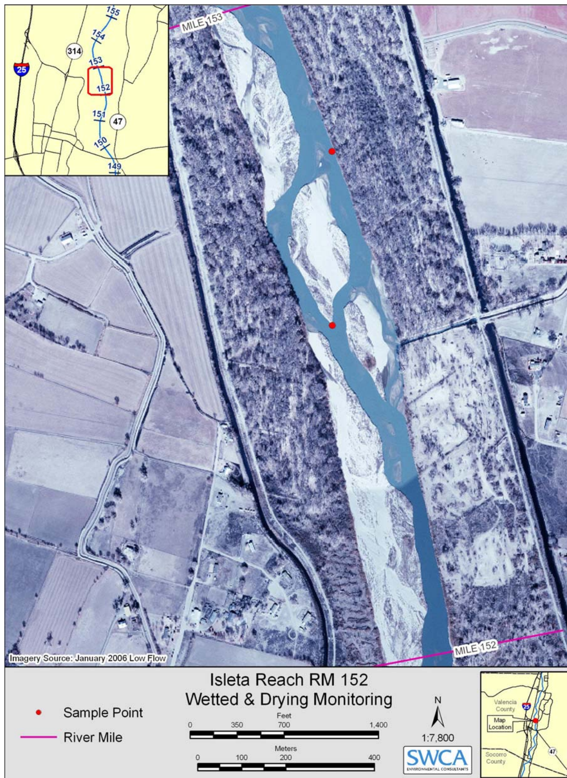
Figure H.1. River mile 152 was the downstream end of drying within the Isleta Reach in 2007. The Peralta Main Canal Wasteway is in the center of the photo and was a significant source of supplemental flow throughout the monitoring period.
