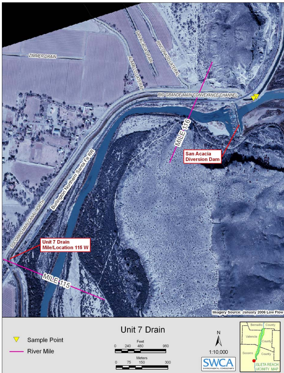
Figure D.10. The Unit 7 Drain sampling site actually lies nearer to the RM 116 than RM 115. The location of the sample points depicted on this map illustrates the location specified by client from which water quality parameters should be monitored.
