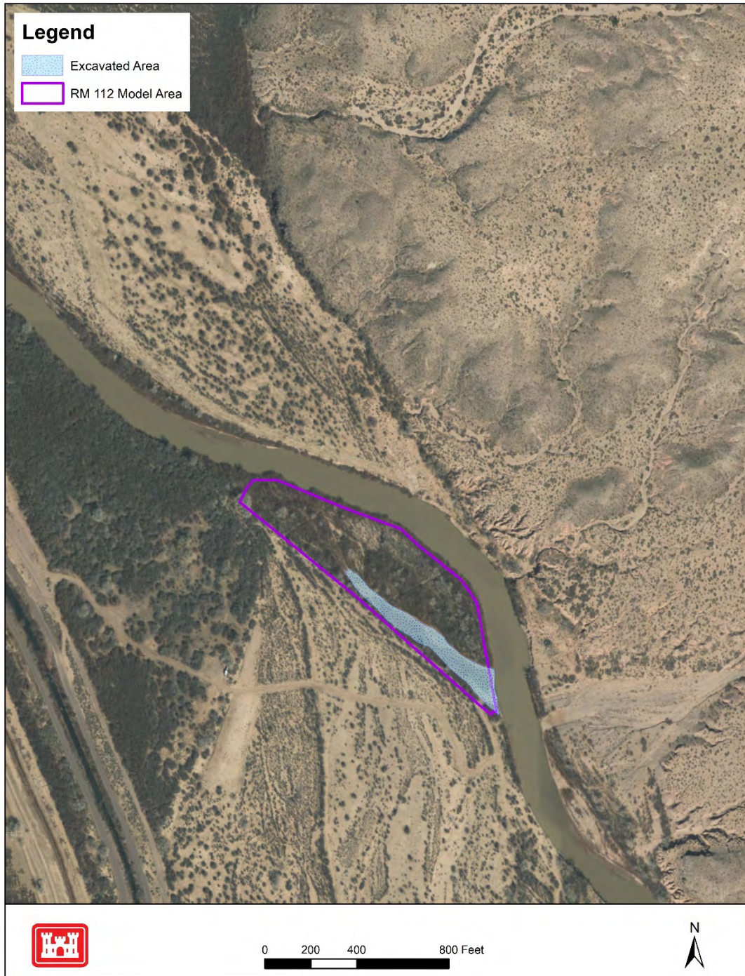
Figure 66. Extents of the 2D model area (evaluated as the adjacent floodplain or “terrace”) and the RM 112 excavated area (HR site).
