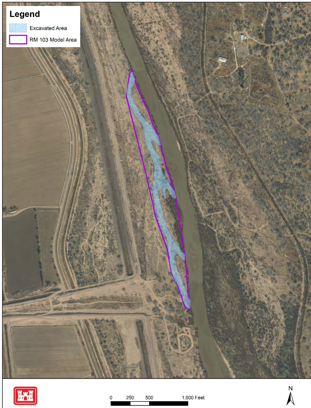
Figure 64. Extents of the 2D model area (evaluated as the adjacent floodplain or “terrace”) and the RM 103 excavated area (HR site).
