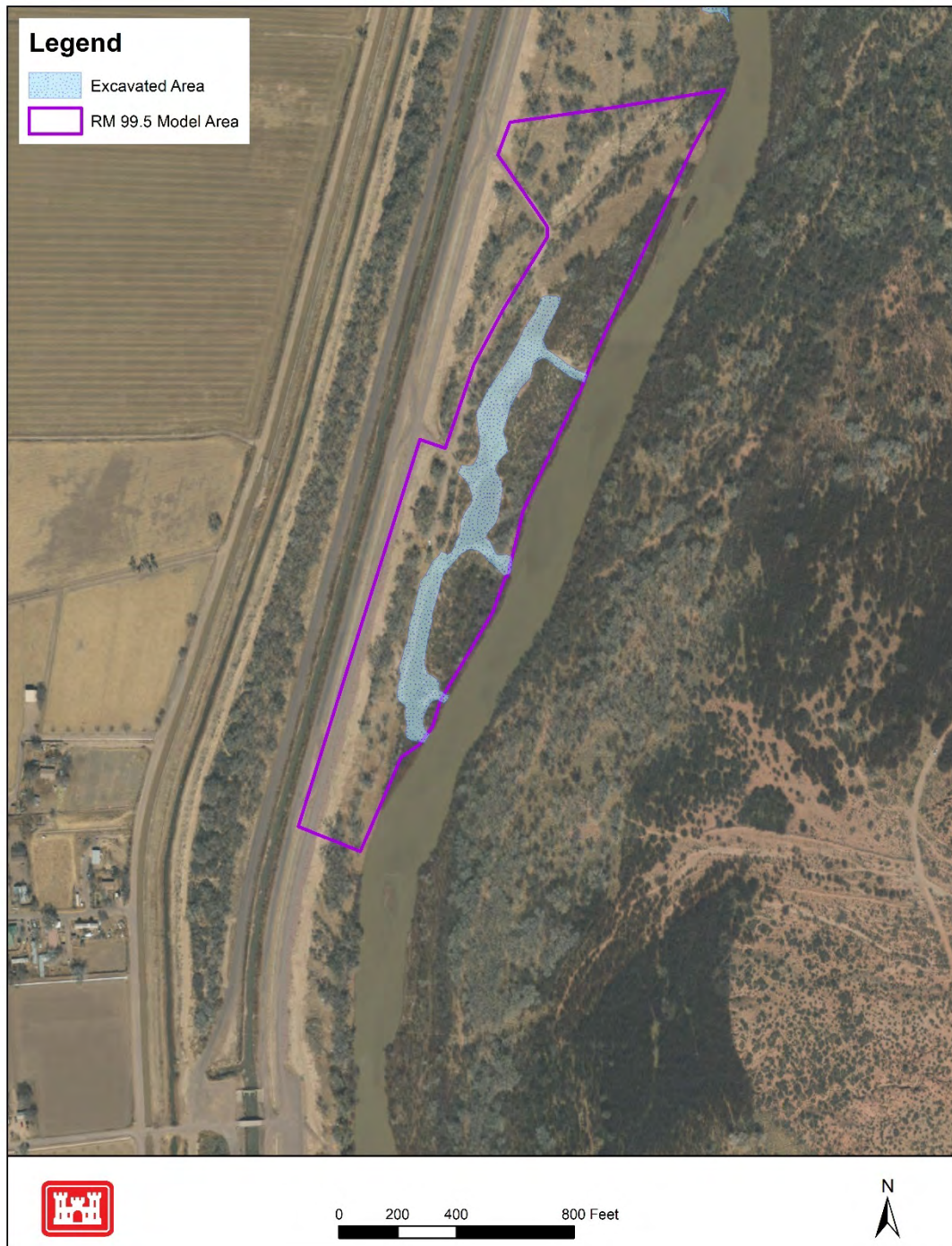
Figure 61. Extents of the 2D model area (evaluated as the adjacent floodplain or “terrace” – geomorphic terrace shown as well) and the RM 99.5 excavated area (HR site).
