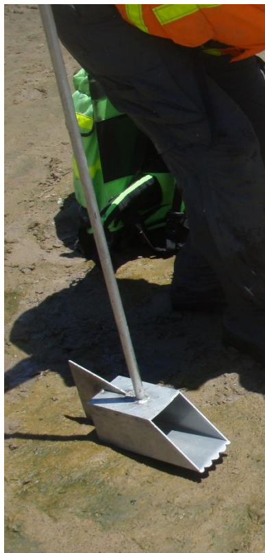
Figure 59. Sediment scoop used for the collection of sediment grab samples in the Cañas study reach (photograph taken by S. Devergie 7/28/2016 on bed material collection south of Belen)
