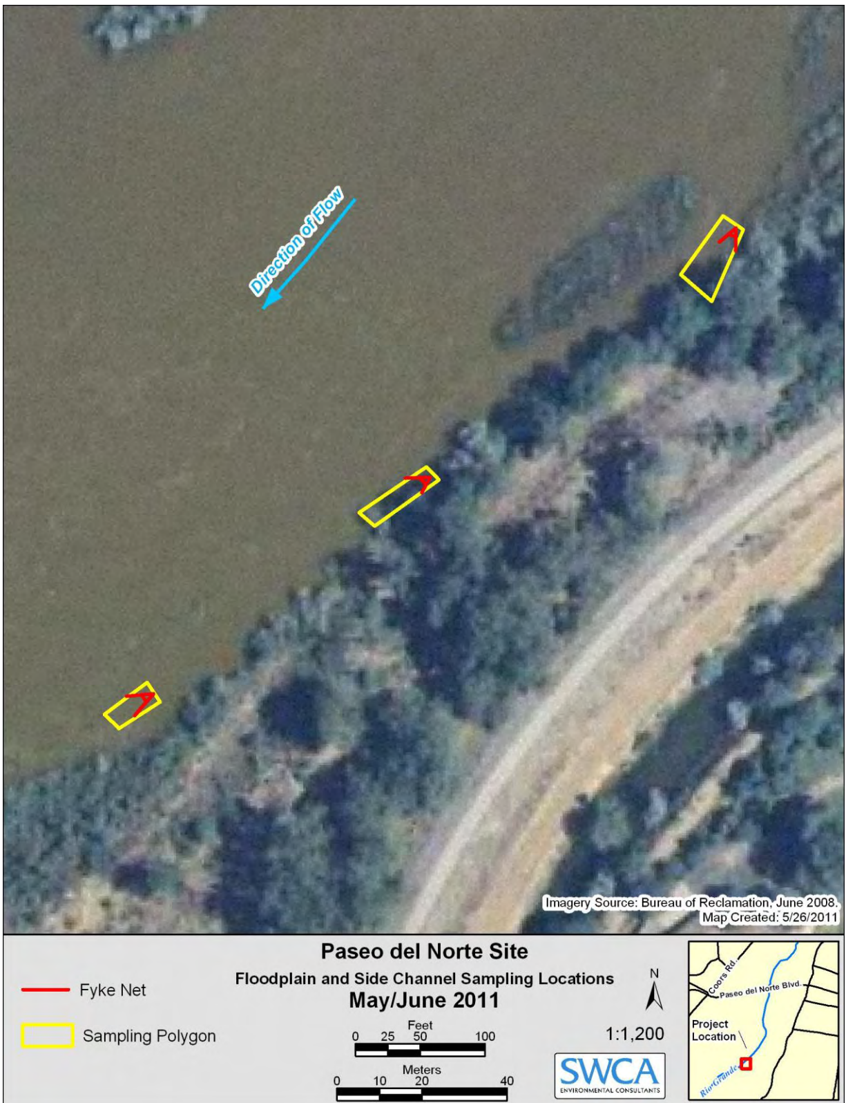
Figure A.2. Paseo Del Norte floodplain and side channel site sampling locations with delineated polygon areas and fyke net placement, May and June 2011. Open area of fyke net triangle depicts fyke wings and sampling direction.
