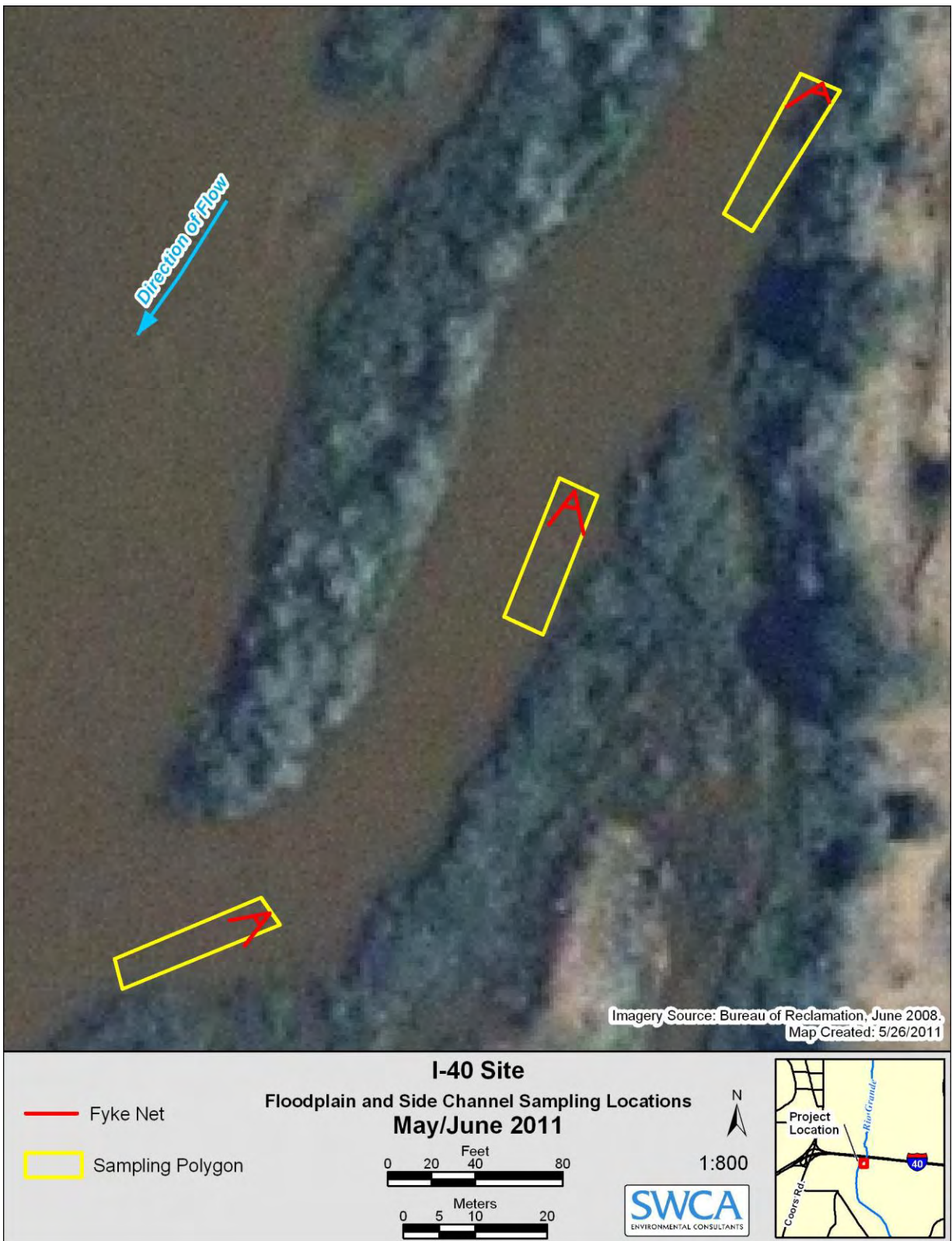
Figure A.4. I-40 site floodplain and side channel sampling locations with delineated polygon areas and fyke net placement, May and June 2011. Open area of fyke net triangle depicts fyke wings and sampling direction.
