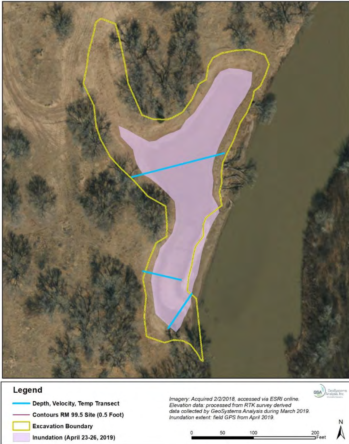
Figure A-8. Inundation extent documented at RM 100 on April 24, 2019. Mean daily discharge at the Escondida gage was 2,740 cfs.
