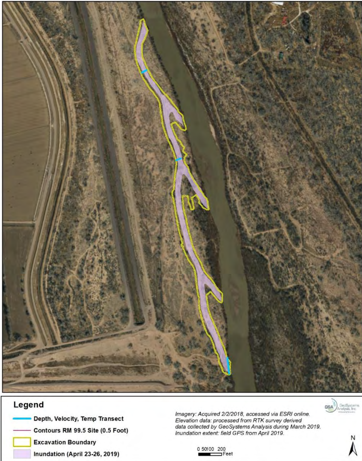
Figure A-12. Inundation extent documented at RM 103 on April 25, 2019. Mean daily discharge at the Escondida gage was 2,830 cfs.
