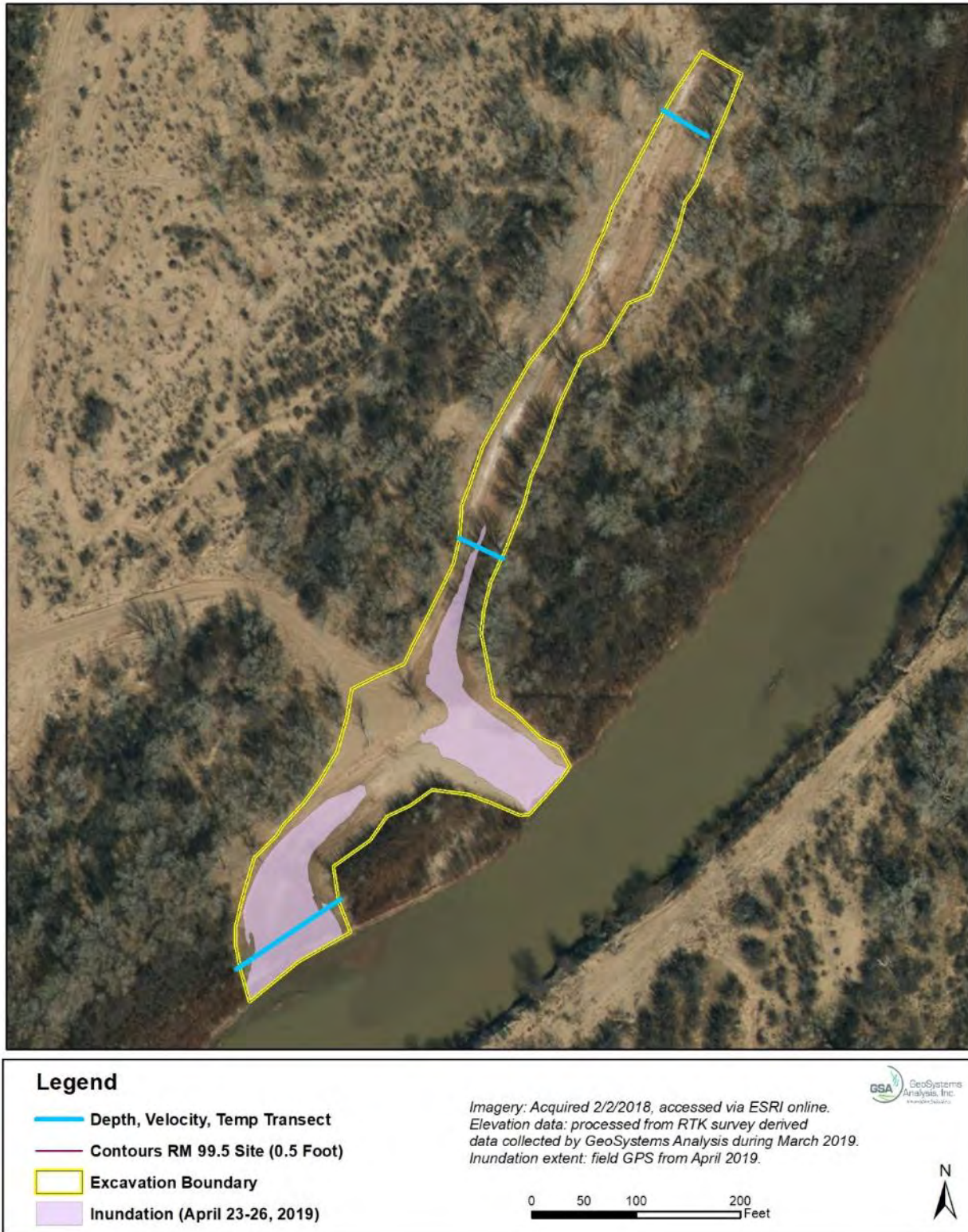
Figure A-2. Inundation extent documented at RM 114 on April 23, 2019. Mean daily discharge at San Acacia gage was 2,530 cfs.
