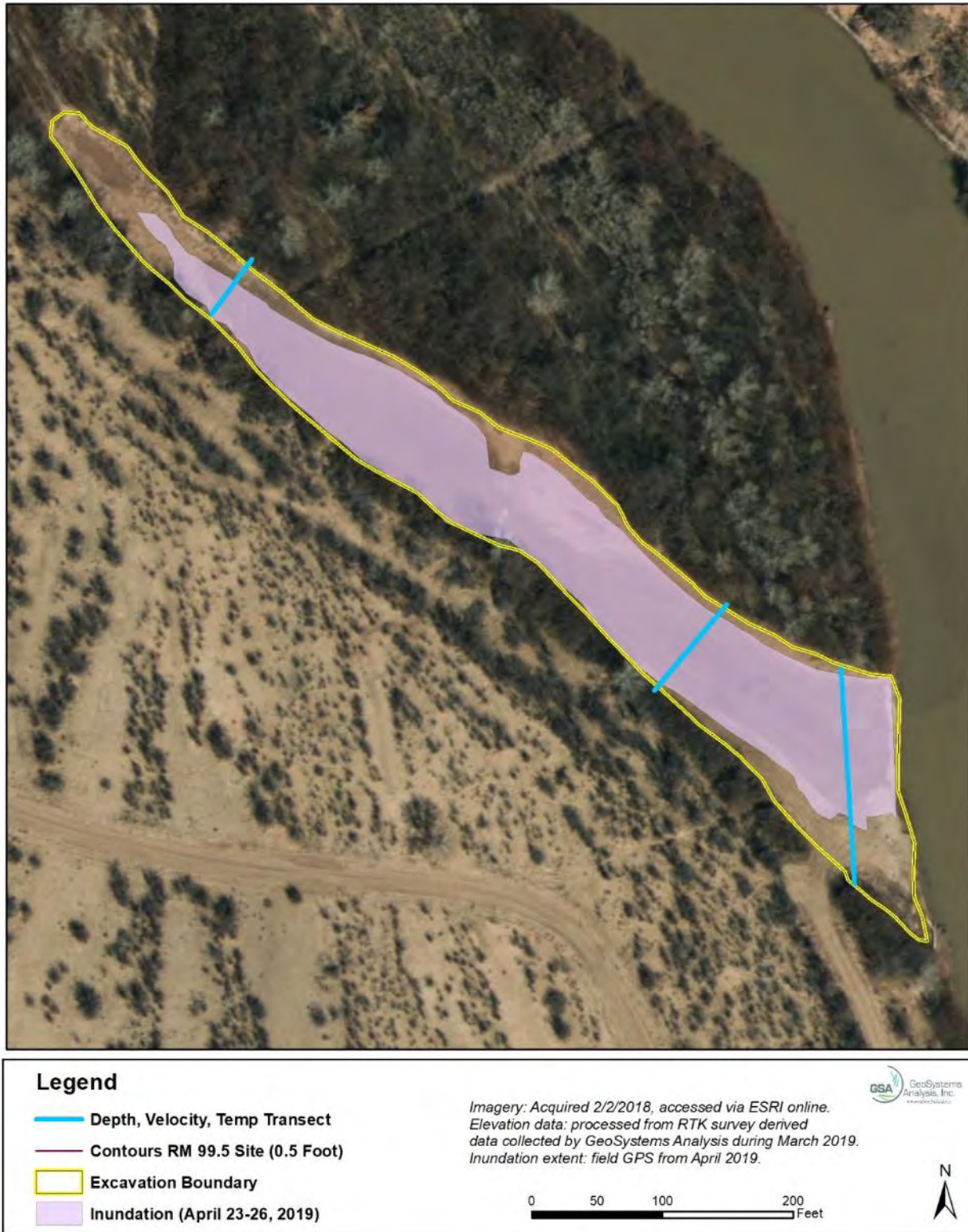
Figure A-4. Inundation extent documented at RM 112 on April 23, 2019. Mean daily discharge at San Acacia gage was 2,530 cfs.
