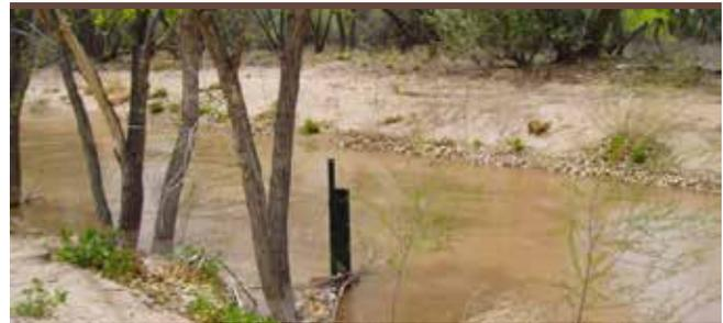
The channel gage at the Rio Grande Nature Center collects data on streamflow through the channel during spring runoff.
