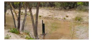
The channel gage at the Rio Grande Nature Center collects data on streamflow through the channel during spring runoff. *Credit: Mick Porter*
