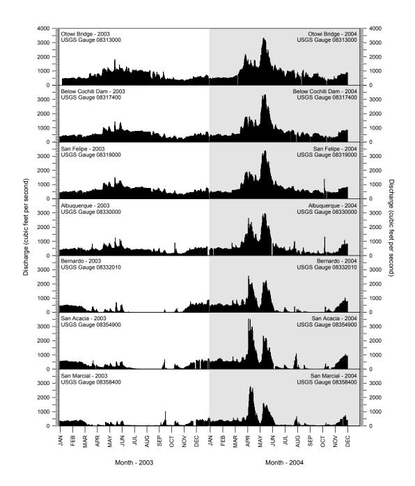
Figure 2. Discharge in the Rio Grande from January 2003 through November 2004 as recorded at seven U. S. Geological Survey (USGS) gauge stations. The Otowi Bridge gauge site is outside of the study area (ca. 25.5 river miles upstream of Cochiti Dam) and provided for reference. Discharge data are provisional and subject to change.
