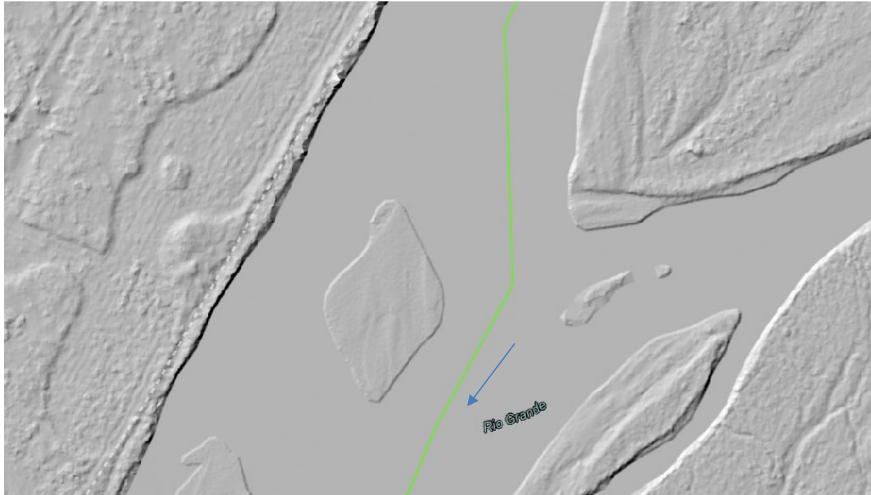
Figure 19. 2022 LiDAR hillshade rendering just upstream of the Alameda Bridge. The centerline was adjusted to avoid the islands visible above the hydroflattened water surface of the 2022 LiDAR hillshade rendering.
