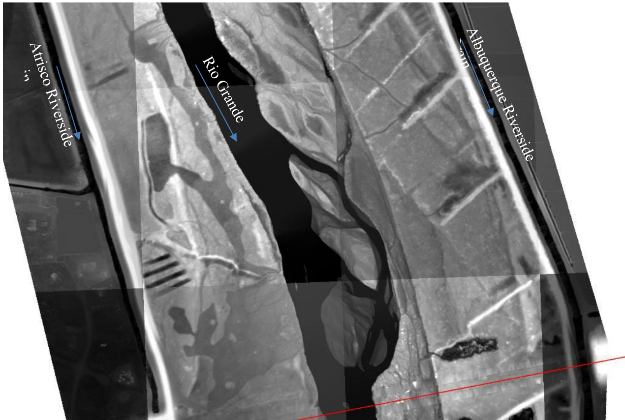
Figure 16. 2022 LiDAR collected for Reclamation. The darkest zones represent the lowest recorded terrain in a given tile. Note there are multiple tiles, so the colors are not always balanced across the sections. These areas clearly delineate the wetted water surface of the Rio Grande and the drains at the time of the LiDAR collection. The flow direction and names of the drains are shown in the figure.
