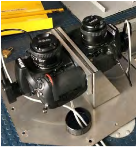
IMAGES: Camera Array with USACE-produced Mount, In-flight Data Collection, and View from Aircraft Sensor Port CREDIT: USACE Staff
