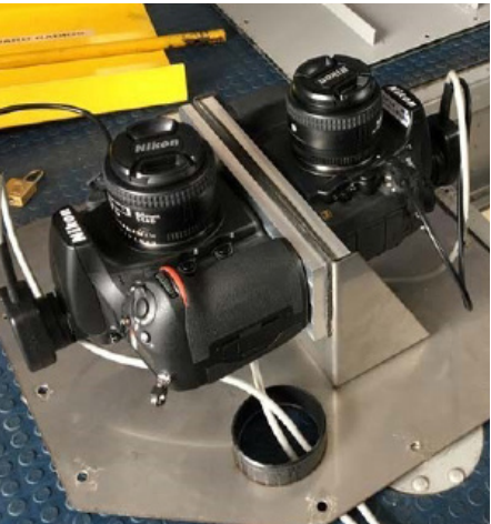
IMAGES: Camera Array with USACE-produced Mount, In-flight Data Collection, and View from Aircraft Sensor Port CREDIT: USACE Staff
