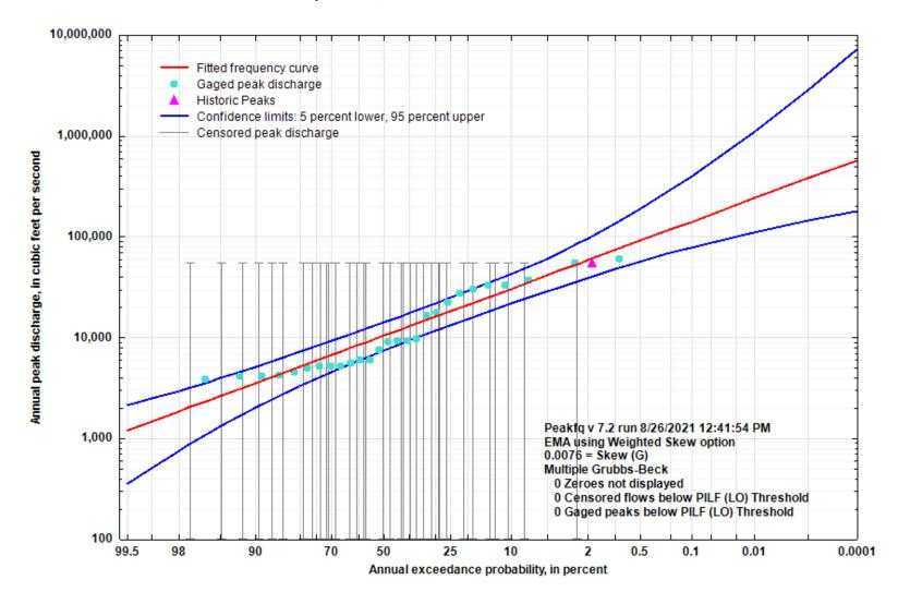
Figure 5-2. Flood Flow Frequency Curve for West Fork White River east of Fayetteville, AR
