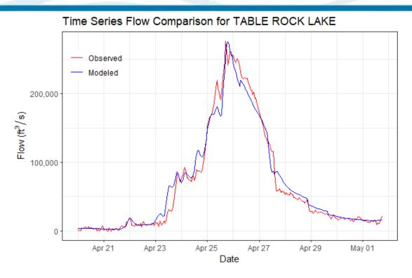
Figure 6-106. Calibration Results for TABLE ROCK LAKE HEC-HMS Junction – Flow at Table Rock Lake (2011 Event)
