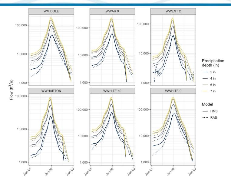
Figure 6-29. Plots showing HEC-RAS 2D and HEC-HMS calibration subbasins within Beaver Lake Watershed
