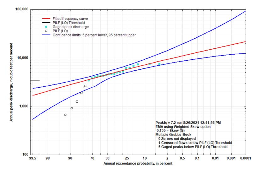
Figure 5-36. Flood Flow Frequency Curve for Bennetts River at Vidette, AR
