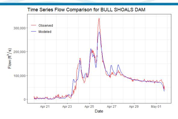
Figure 6-112. Calibration Results for BULL SHOALS DAM HEC-HMS Junction – Flow at Bull Shoals Dam (2011 Event)
