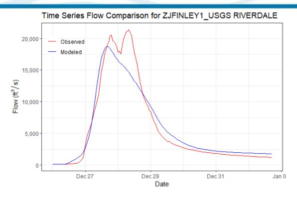
Figure 6-72. Calibration Results for ZJFINLEY1\_USGS RIVERDALE HEC-HMS Junction – Finley Creek below Riverdale, MO Gage (07052345, 2015 Event)
