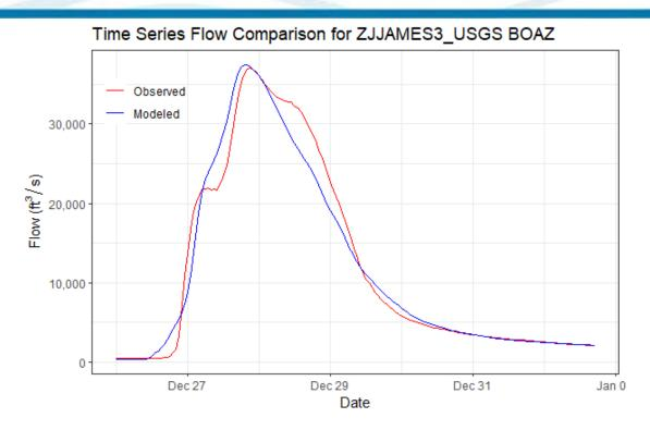
*Figure 6-74. Calibration Results for ZJJAMES3\_USGS BOAZ HEC-HMS Junction – James River* near Boaz, MO Gage (07052250, 2015 Event)
