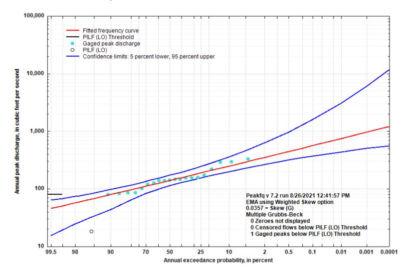
Figure 5-57. Flood Flow Frequency Curve for Fourche River Tributary at Middlebrook, AR
