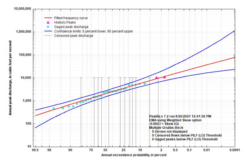
Figure 5-48. Flood Flow Frequency Curve for Big Creek near Yukon, MO
