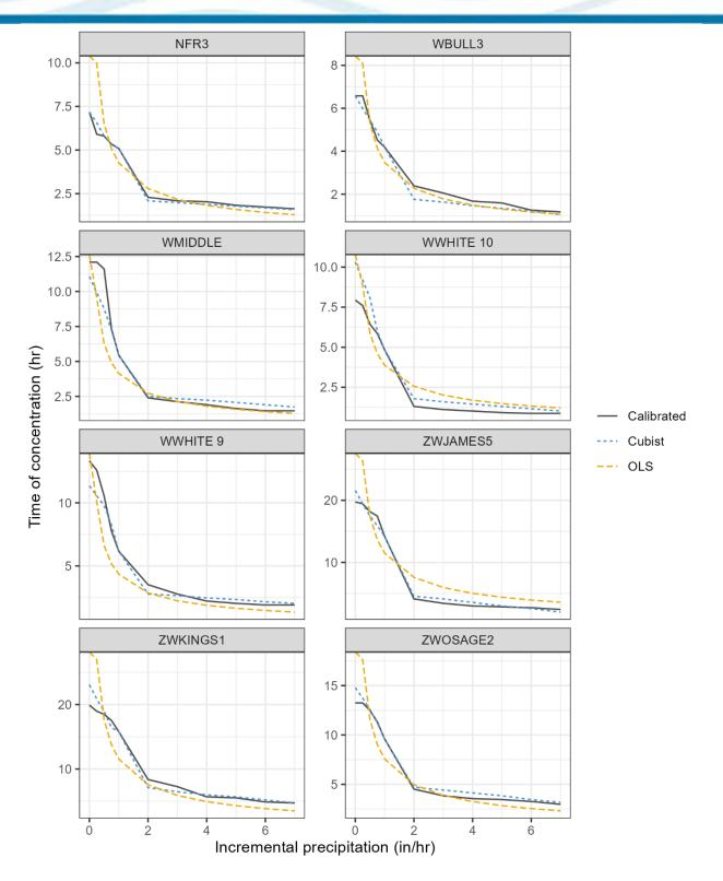
Figure 6-26. Plots showing results, in hours, for LOOCV for Tc
