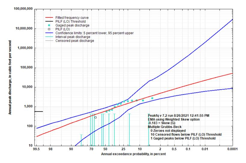
Figure 5-14. Flood Flow Frequency Curve for Dry Crane Creek near Crane, MO
