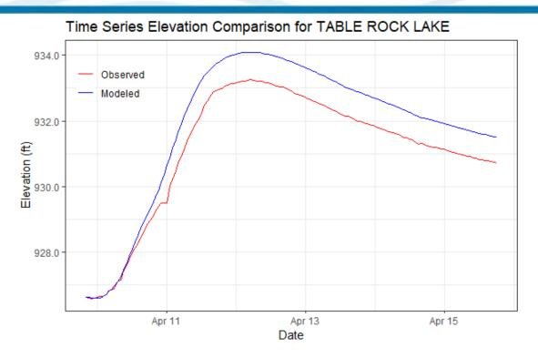
Figure 6-128. Validation Results for TABLE ROCK LAKE HEC-HMS Junction – Elevation at Table Rock Lake (2008 Event)
