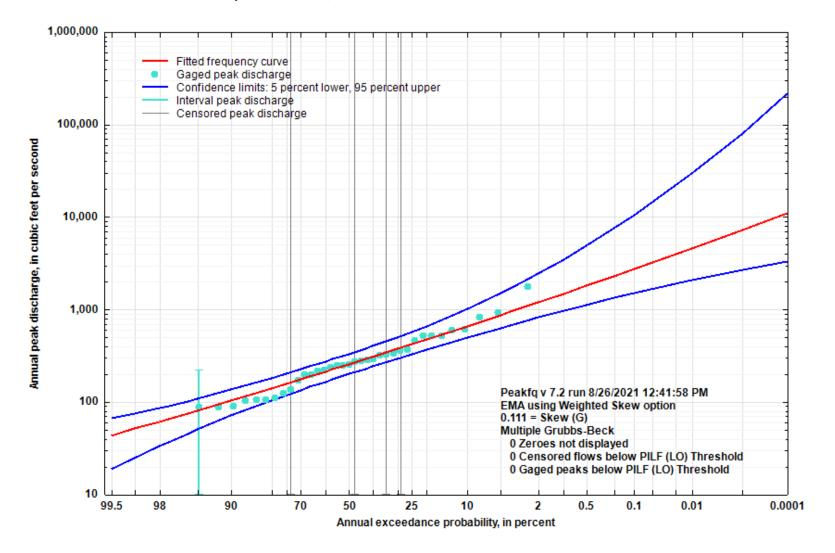
Figure 5-74. Flood Flow Frequency Curve for Choctaw Creek Tributary near Choctaw, AR
