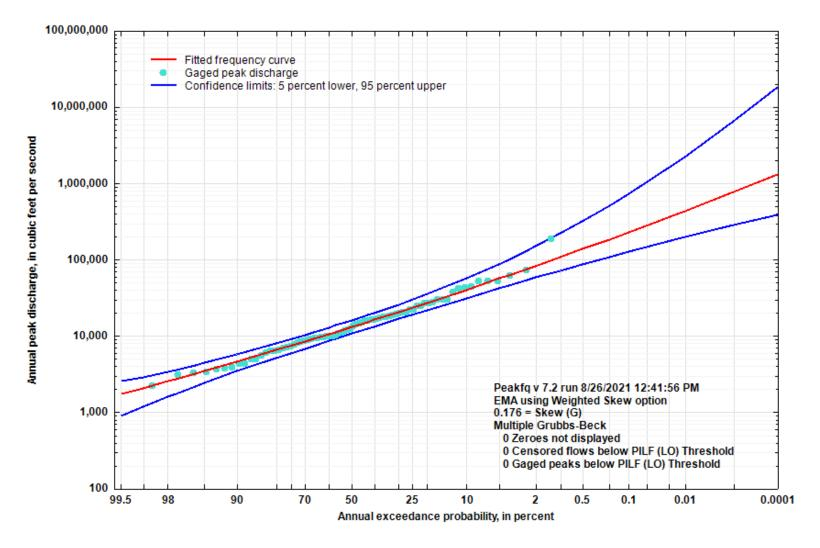
Figure 5-34. Flood Flow Frequency Curve for North Fork River near Tecumseh, MO
