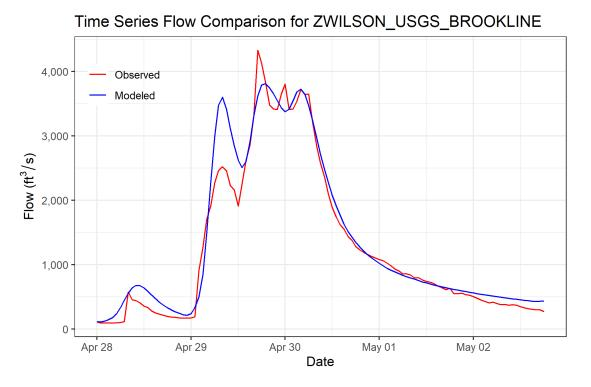
Figure 6-47. Calibration Results for ZWILSON\_USGS\_BROOKLINE HEC-HMS Junction – Wilson Creek near Brookline, MO Gage (07052152, 2017 Event)
