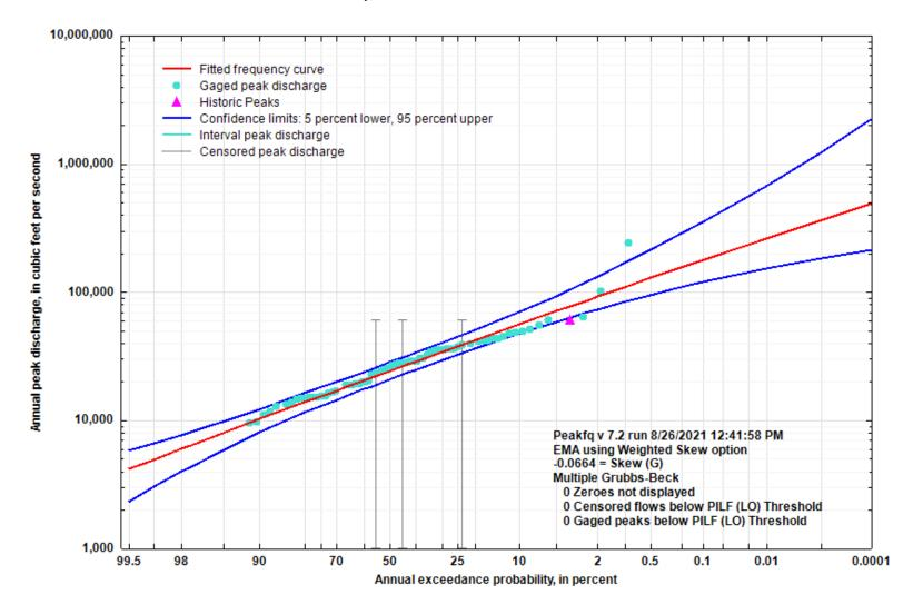
Figure 5-72. Flood Flow Frequency Curve for Middle Fork of Little Red River at Shirley, AR
