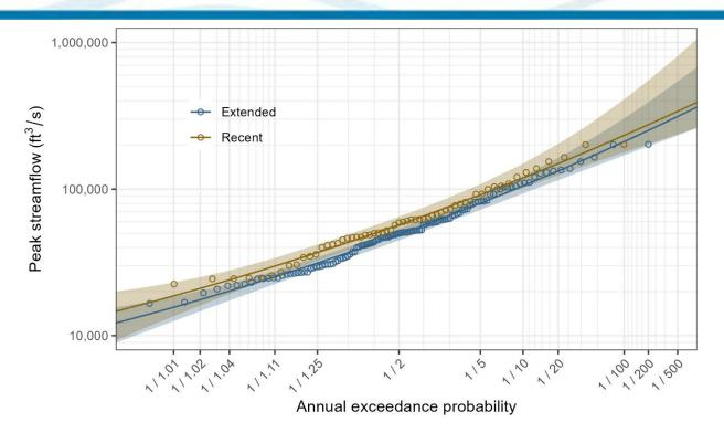
Figure 11-7 Comparison of regulated to extended period of record AEP streamflows for USGS 07060500 White River at Calico Rock AR
