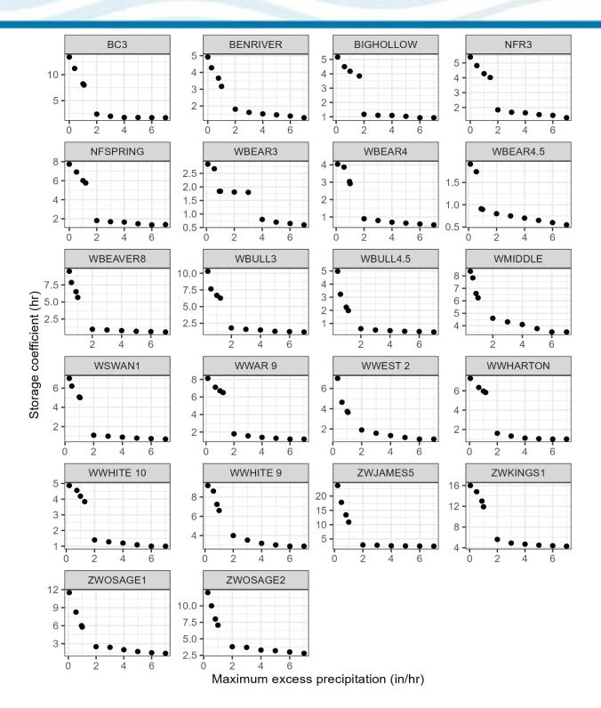
Figure 6-34. Plots showing R and maximum excess precipitation for subbasins used for creating Variable Clark curves
