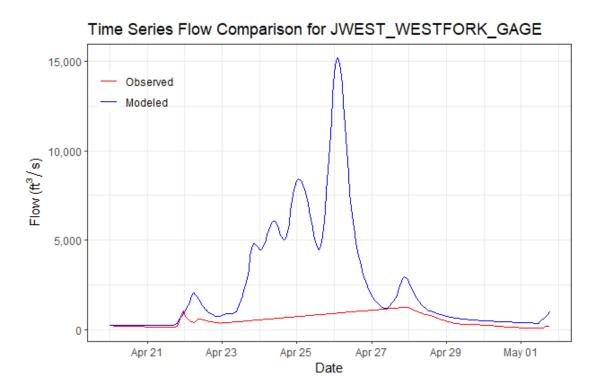
Figure 6-89. Calibration Results for JWEST\_WESTFORK\_GAGE HEC-HMS Junction – West Fork of White River east of Fayetteville Gage (07048550, 2011 Event)
