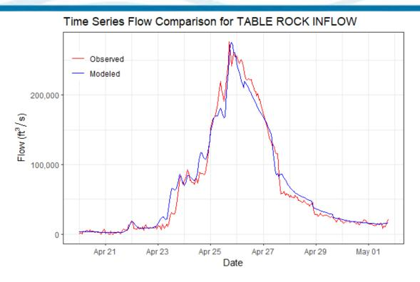
Figure 6-104. Calibration Results for TABLE ROCK INFLOW HEC-HMS Junction – Inflow to Table Rock Lake (2011 Event)
