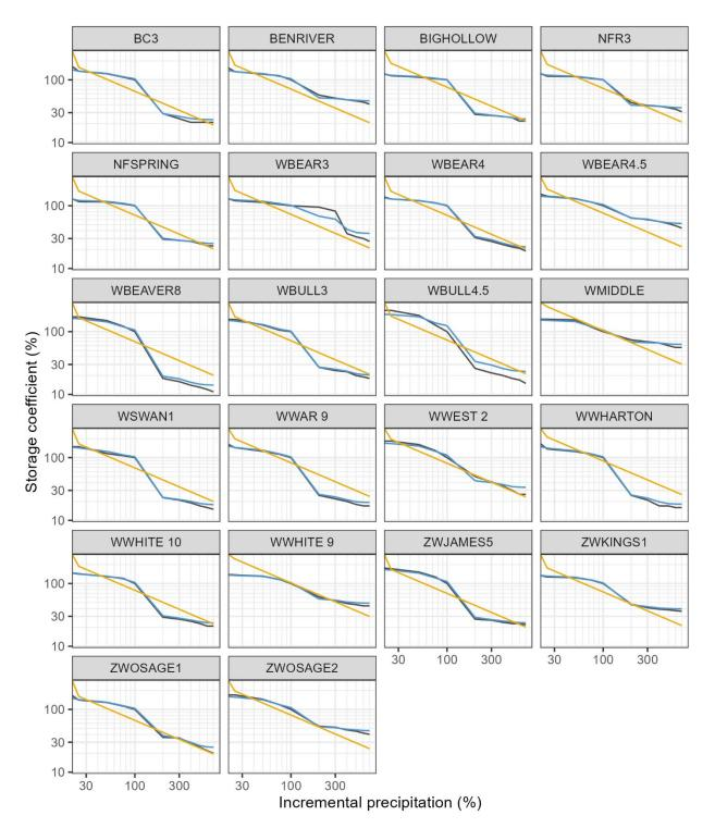
Figure 6-38. Plots showing calibrated R curves and predicted R curves from Cubist and from Ordinary Least Square (OLS) regression.
