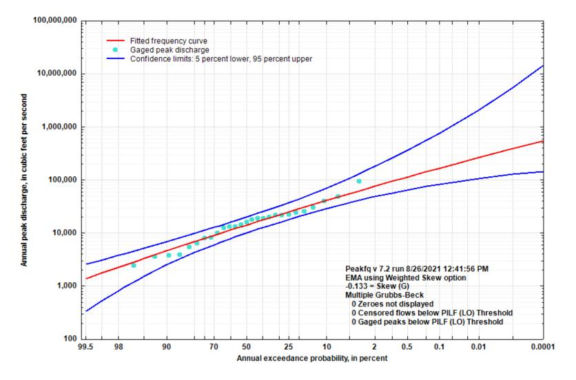
Figure 5-49. Flood Flow Frequency Curve for Jacks Fork at Alley Spring, MO
