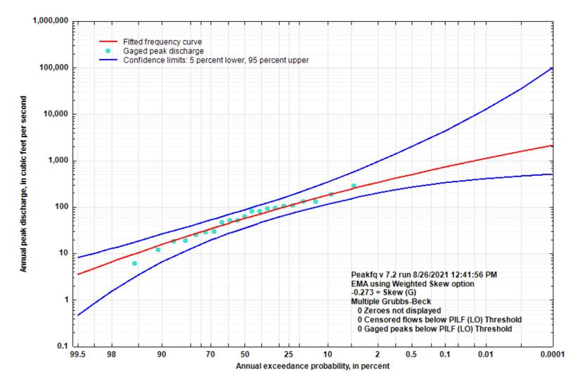
Figure 5-41. Flood Flow Frequency Curve for Wolf Bayou near Drasco, AR
