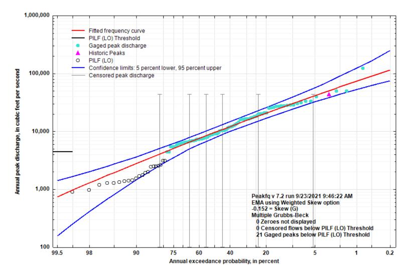
Figure 5-63. Flood Flow Frequency Curve for Eleven Point River near Bardley, MO
