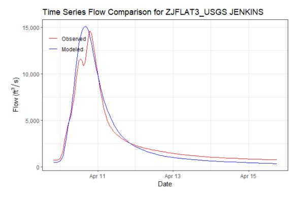
Figure 6-123. Validation Results for ZJFLAT3\_USGS JENKINS HEC-HMS Junction – Flat Creek below Jenkins, MO Gage (2008 Event)
