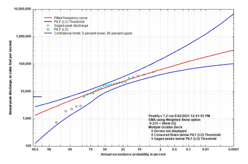
Figure 5-20. Flood Flow Frequency Curve for Beaver Creek at Bradleyville, MO
