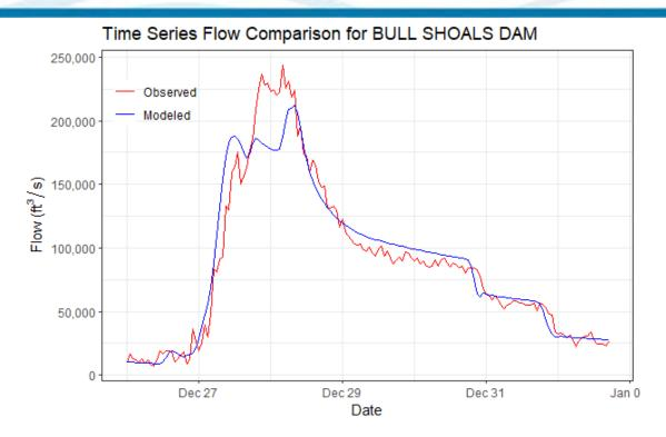
Figure 6-88. Calibration Results for BULL SHOALS DAM HEC-HMS Junction – Flow at Bull Shoals Dam (2015 Event)
