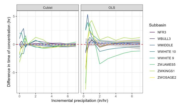
Figure 6-23. Plots showing differences in calibrated Tc values vs Tc values estimated by regression. Blue dotted line with confidence interval is linear regression of all values. Red dashed line is at Y = 0.
