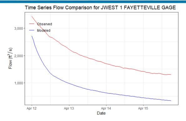
Figure 6-114. Validation Results for JWEST 1 FAYETTEVILLE GAGE HEC-HMS Junction – White River at Fayetteville, AR Gage (2008 Event)
