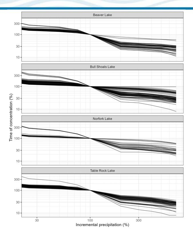
Figure 6-39. Plots showing variable Tc curves for selected HEC-HMS subbasins
