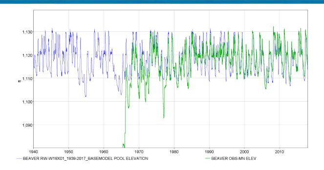
Figure 8-8. Observed and modeled pool elevation for Beaver Dam from 1940-2017.
