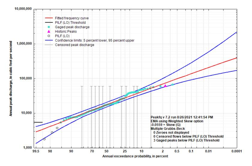
Figure 5-8. Flood Flow Frequency Curve for Kings River near Berryville, AR
