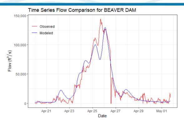
Figure 6-94. Calibration Results for BEAVER DAM HEC-HMS Junction – Flow at Beaver Dam (2011 Event)
