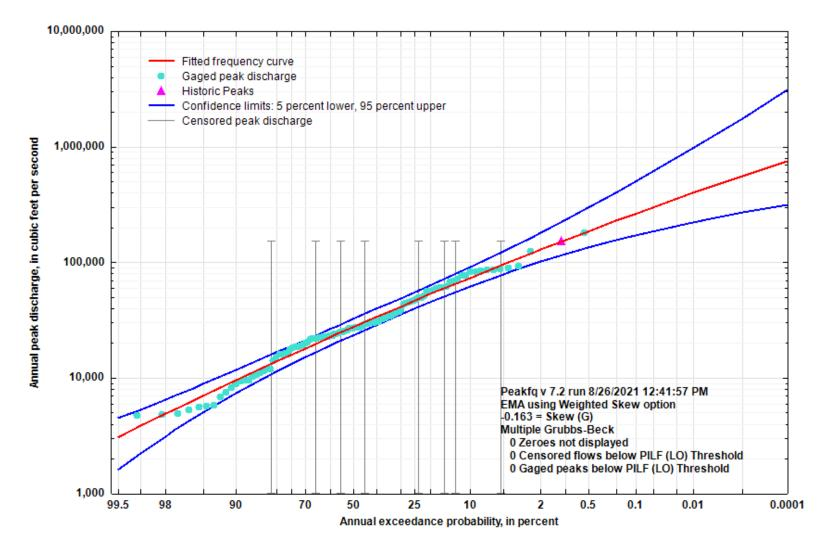
Figure 5-53. Flood Flow Frequency Curve for Current River at Van Buren, MO
