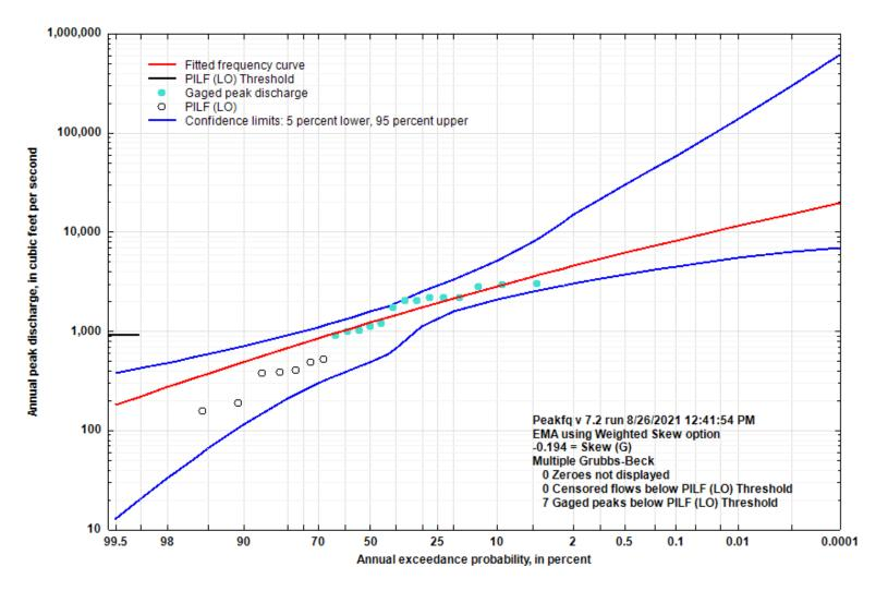
Figure 5-10. Flood Flow Frequency Curve for Pearson Creek near Springfield, MO
