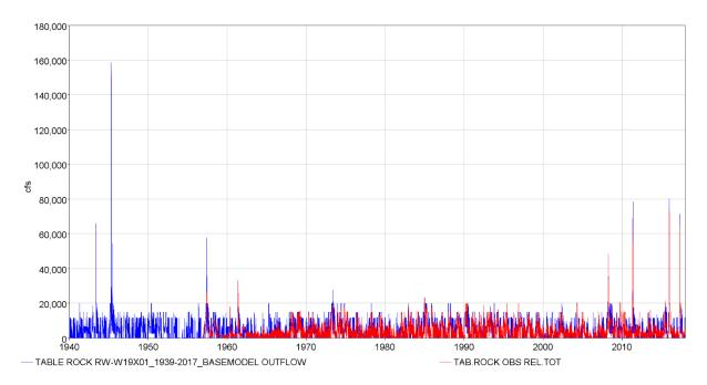
Figure 8-13. Observed and modeled releases for Table Rock Dam from 1940-2017.
