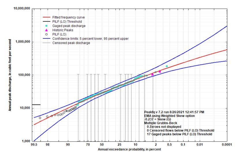
Figure 5-54. Flood Flow Frequency Curve for Current River at Doniphan, MO
