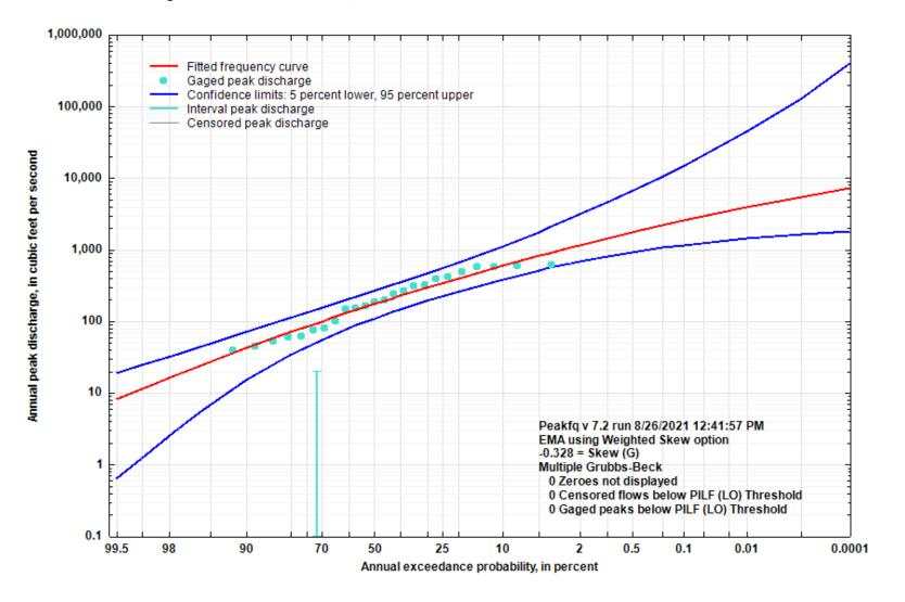
Figure 5-55. Flood Flow Frequency Curve for North Prong Little Black River at Hunter, MO
