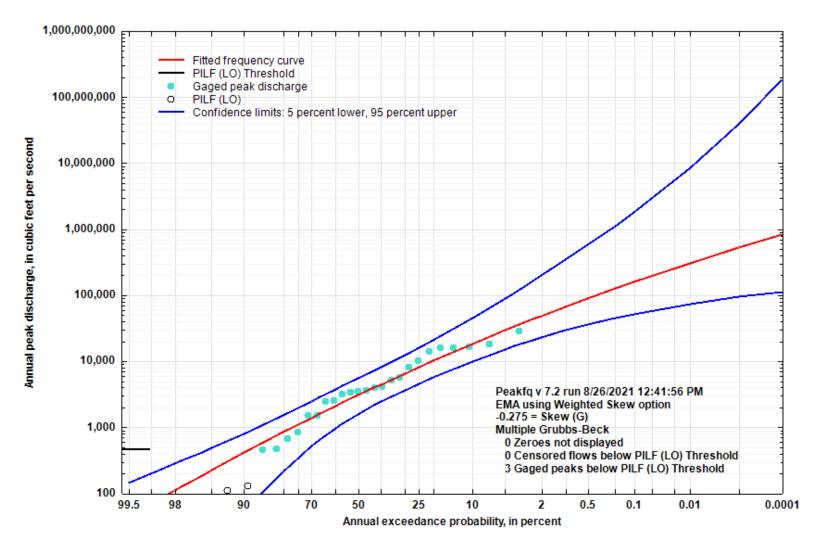
Figure 5-45. Flood Flow Frequency Curve for Logan Creek at Ellington, MO
