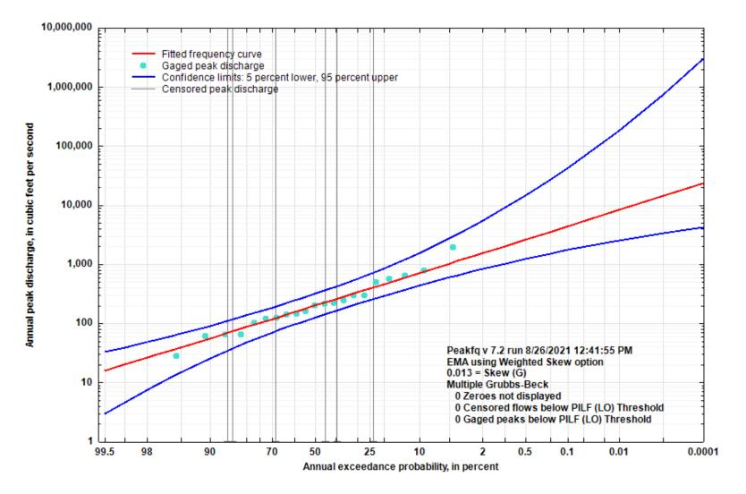
Figure 5-12. Flood Flow Frequency Curve for Maple Grove Branch near Ozark, MO
