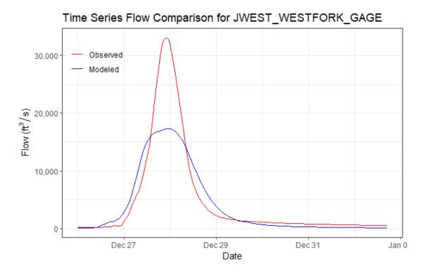
Figure 6-65. Calibration Results for JWEST\_WESTFORK\_GAGE HEC-HMS Junction – West Fork of White River east of Fayetteville, AR Gage (07048550, 2015 Event)
