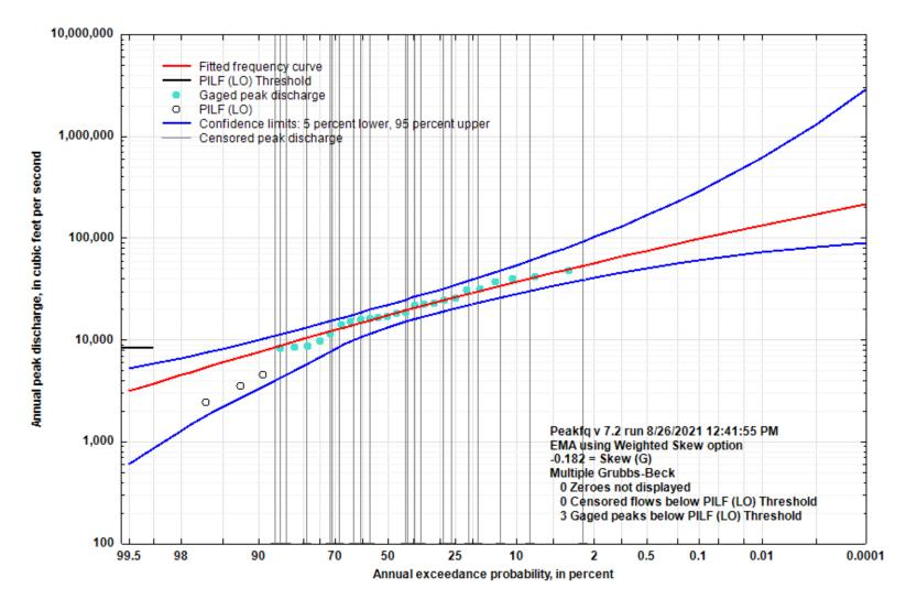
Figure 5-13. Flood Flow Frequency Curve for James River near Boaz, MO
