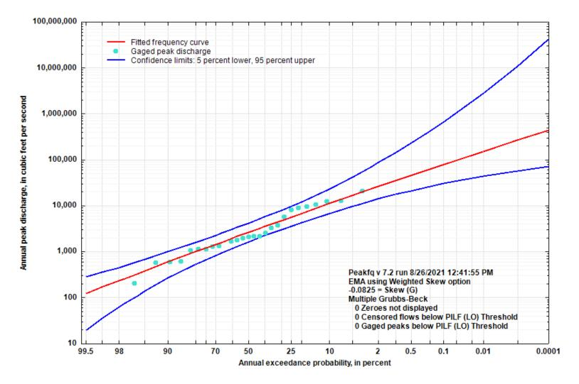
Figure 5-17. Flood Flow Frequency Curve for Yocum Creek near Oak Grove, AR
