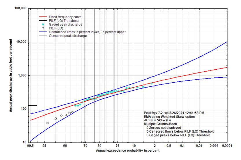
Figure 5-76. Flood Flow Frequency Curve for Key Branch near Searcy, AR
