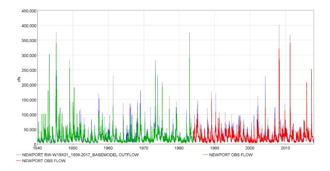
Figure 8-23. Observed and modeled flow at Newport from 1940-2017.
