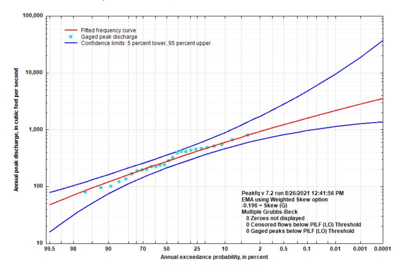
Figure 5-33. Flood Flow Frequency Curve for Dodd Creek Tributary near Mountain Home, AR
