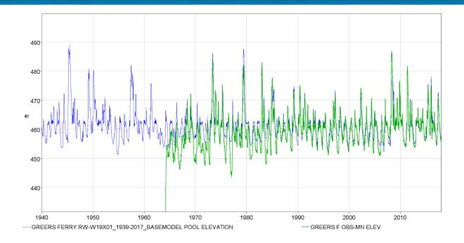
*Figure 8-20. Observed and modeled pool elevation for Greers Ferry Dam from 1940-2017.*
