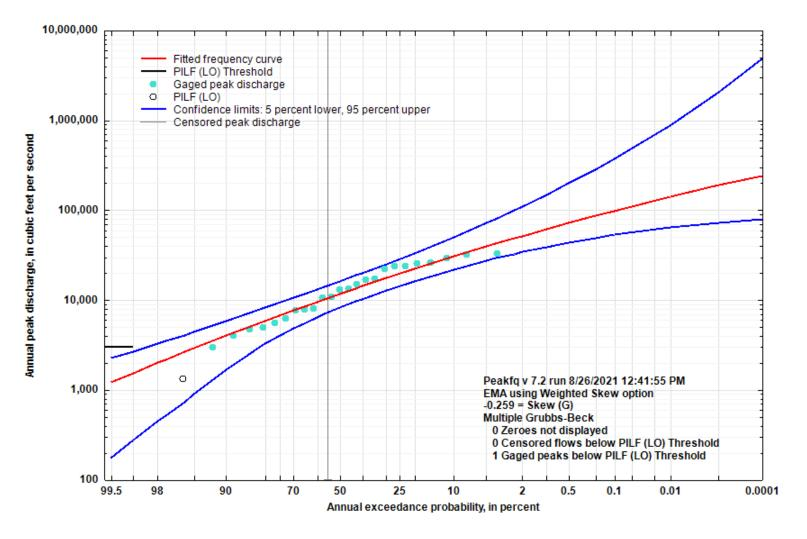
Figure 5-18. Flood Flow Frequency Curve for Bull Creek near Walnut Shade, MO
