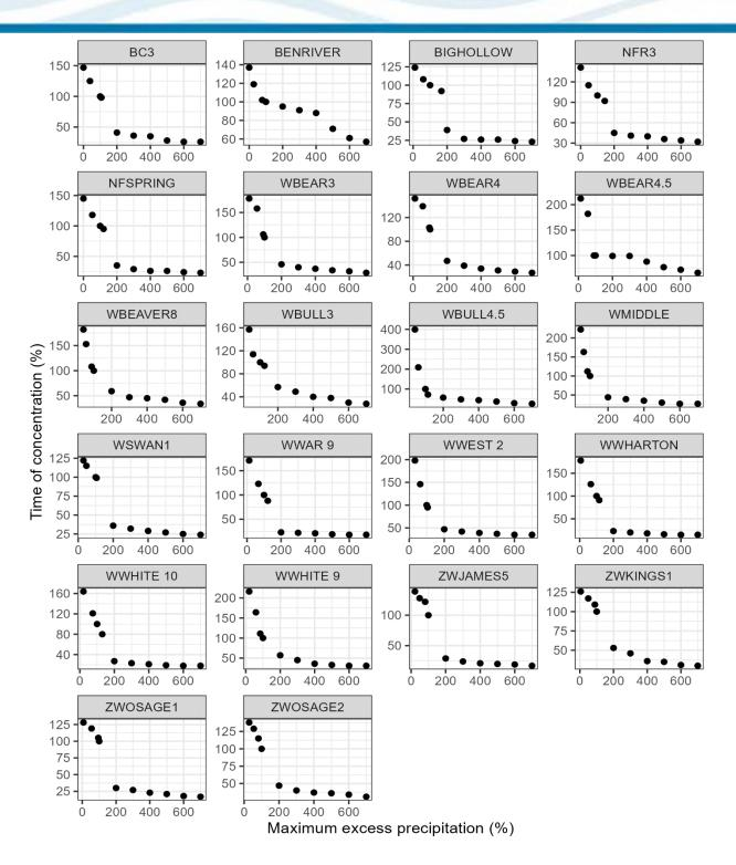
Figure 6-35. Plots showing Tc percentage and maximum excess precipitation percentage for subbasins used for creating Variable Clark curves
