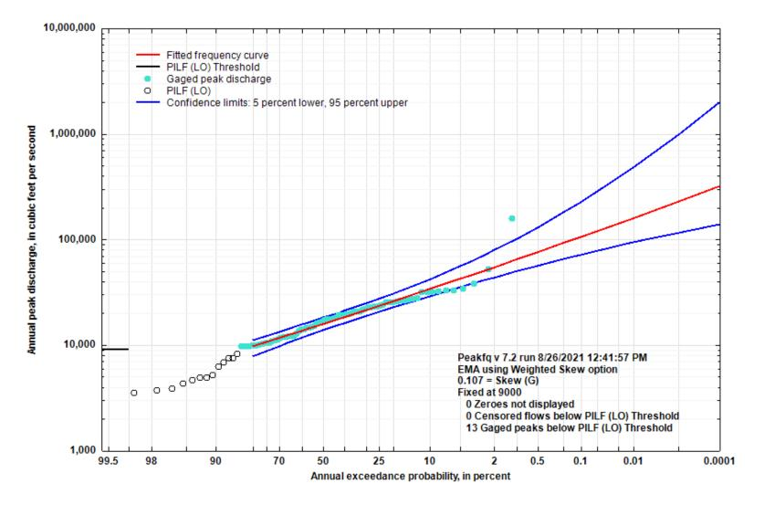
Figure 5-67. Flood Flow Frequency Curve for Strawberry River near Poughkeepsie, AR
