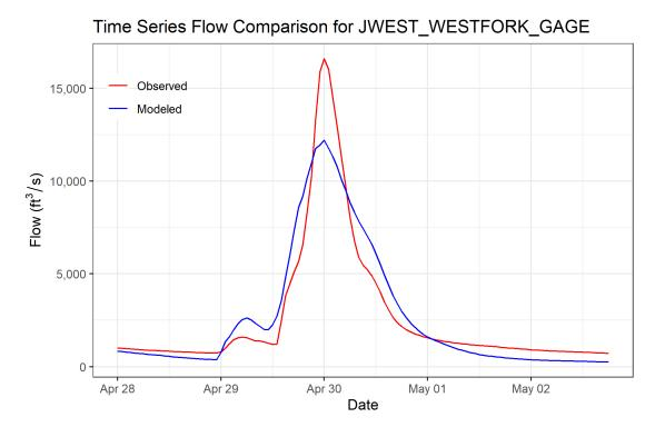
Figure 6-41. Calibration Results for JWEST\_WESTFORK\_GAGE HEC-HMS Junction – West Fork of White River east of Fayetteville, AR Gage (07048550, 2017 Event)
