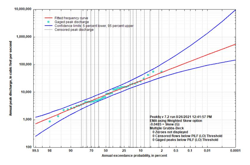
Figure 5-56. Flood Flow Frequency Curve for Little Black River below Fairdealing, MO
