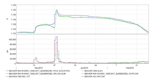
Figure 8-2. Observed and modeled pool elevation for Beaver Dam for Dec 2015 storm event.
