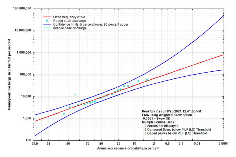
Figure 5-24. Flood Flow Frequency Curve for Bear Creek near Omaha, AR
