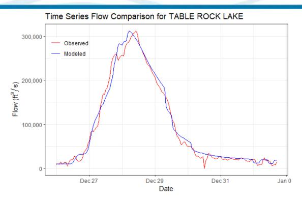
Figure 6-82. Calibration Results for TABLE ROCK LAKE HEC-HMS Junction – Flow at Table Rock Lake (2015 Event)
