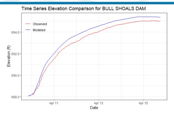
Figure 6-134. Validation Results for BULL SHOALS DAM HEC-HMS Junction – Elevation at Bull Shoals Lake (2008 Event)
