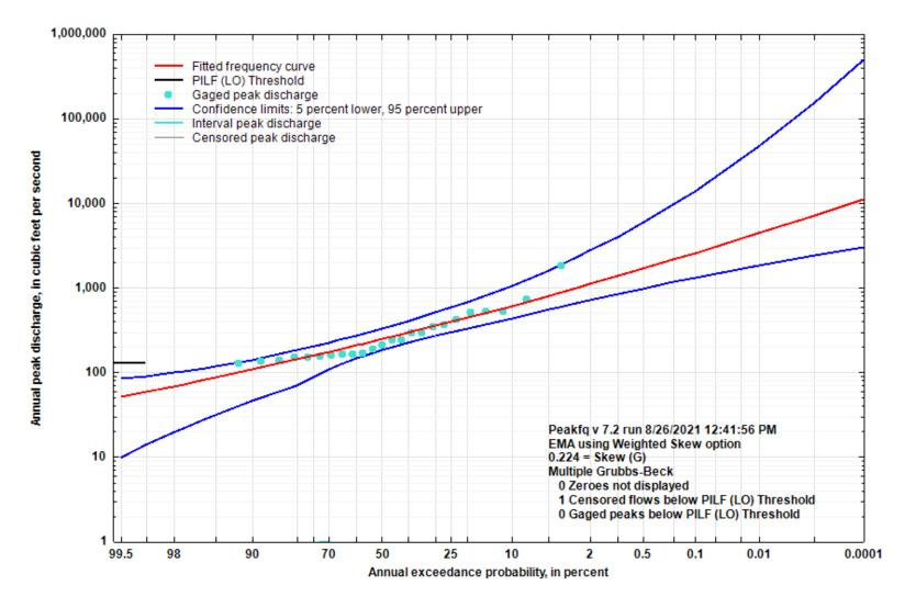
Figure 5-38. Flood Flow Frequency Curve for Band Mill Creek near Brockwell, AR
