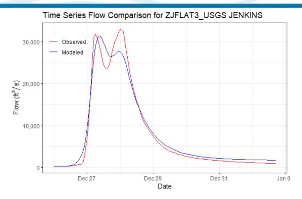
Figure 6-76. Calibration Results for ZJFLAT3\_USGS JENKINS HEC-HMS Junction – Flat Creek below Jenkins, MO Gage (07052820, 2015 Event)
