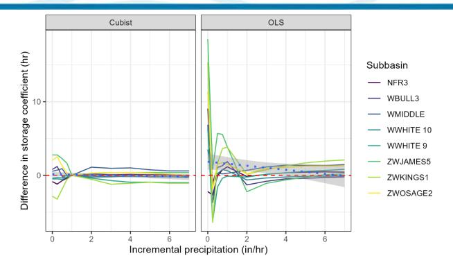
Figure 6-24. Plots showing differences in calibrated R values vs R values estimated by regression. Blue dotted line with confidence interval is linear regression of all values. Red dashed line is at Y = 0.
