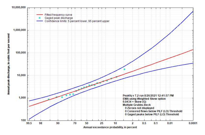
Figure 5-69. Flood Flow Frequency Curve for Reeds Creek near Strawberry
