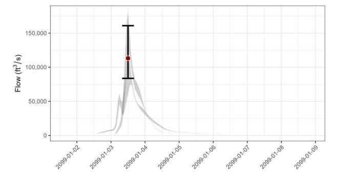
Figure 10-4 Results from stochastic precipitation frequency for USGS 07049000
