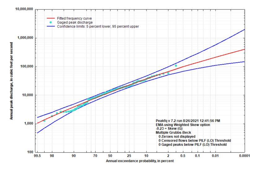
Figure 5-50. Flood Flow Frequency Curve for Jacks Fork at Eminence, MO
