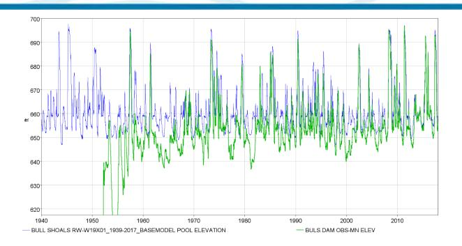
Figure 8-14. Observed and modeled pool elevation for Bull Shoals Dam from 1940-2017.
