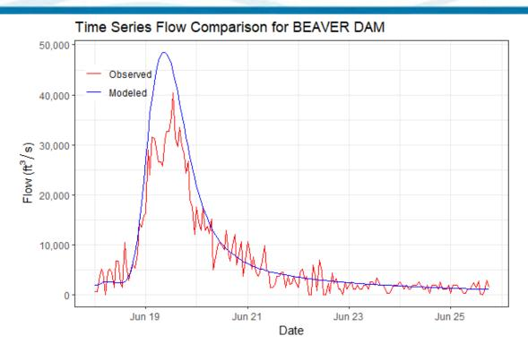
Figure 6-141. Validation Results for BEAVER DAM HEC-HMS Junction – Flow at Beaver Dam (2015 Event)
