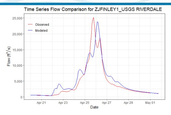
Figure 6-96. Calibration Results for ZJFINLEY1\_USGS RIVERDALE HEC-HMS Junction – Finley Creek below Riverdale, MO Gage (07052345, 2011 Event)
