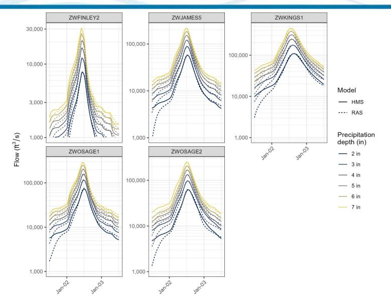
Figure 6-30. Plots showing HEC-RAS 2D and HEC-HMS calibration subbasins within Table Rock Lake Watershed
