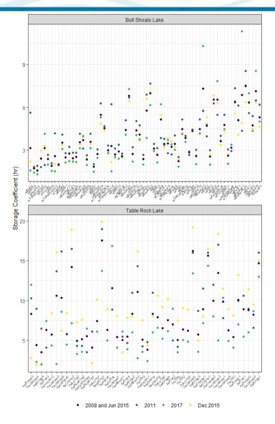
Figure 6-12. Storage Coefficient – Bull Shoals and Table Rock Lakes Subbasins
