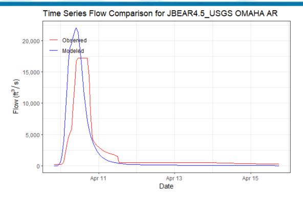
Figure 6-132. Validation Results for JBEAR4.5\_USGS OMAHA HEC-HMS Junction – Bear Creek near Omaha, AR Gage (2008 Event)
