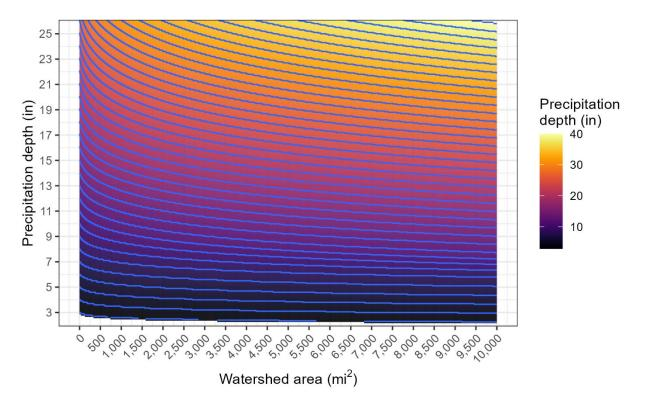
*Figure 7-5. Plot showing results of depth-area-reduction analysis based on all sites used in the analysis.*
