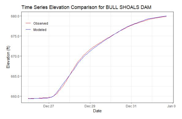
Figure 6-87. Calibration Results for BULL SHOALS DAM HEC-HMS Junction – Elevation at Bull Shoals Lake (2015 Event)
