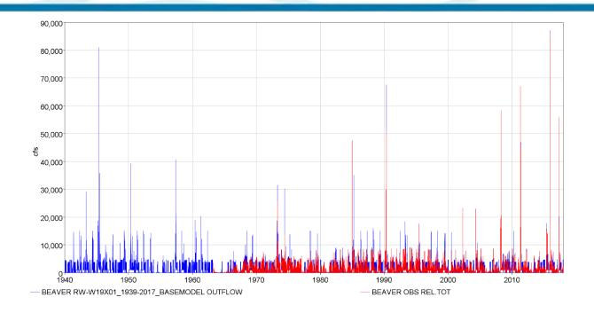
*Figure 8-10. Observed and modeled releases for Beaver Dam from 1940-2017.*
