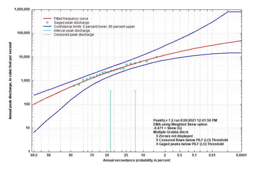
Figure 5-43. Flood Flow Frequency Curve for East Fork Black River near Ironton, MO
