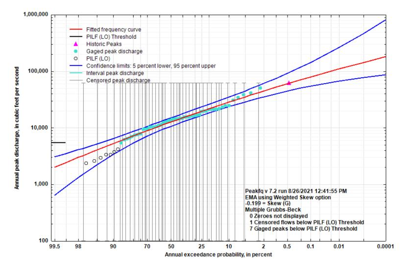
Figure 5-11. Flood Flow Frequency Curve for James River near Springfield, MO
