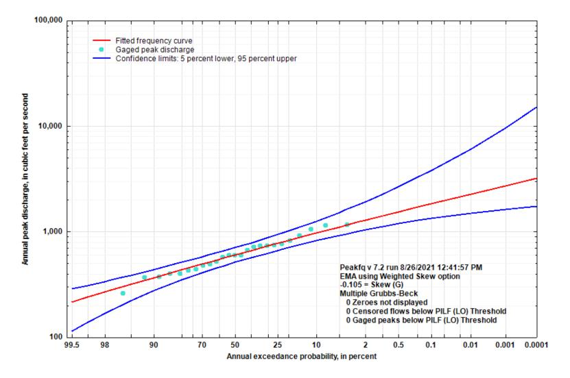
Figure 5-65. Flood Flow Frequency Curve for Hubble Creek near Pocahontas, AR
