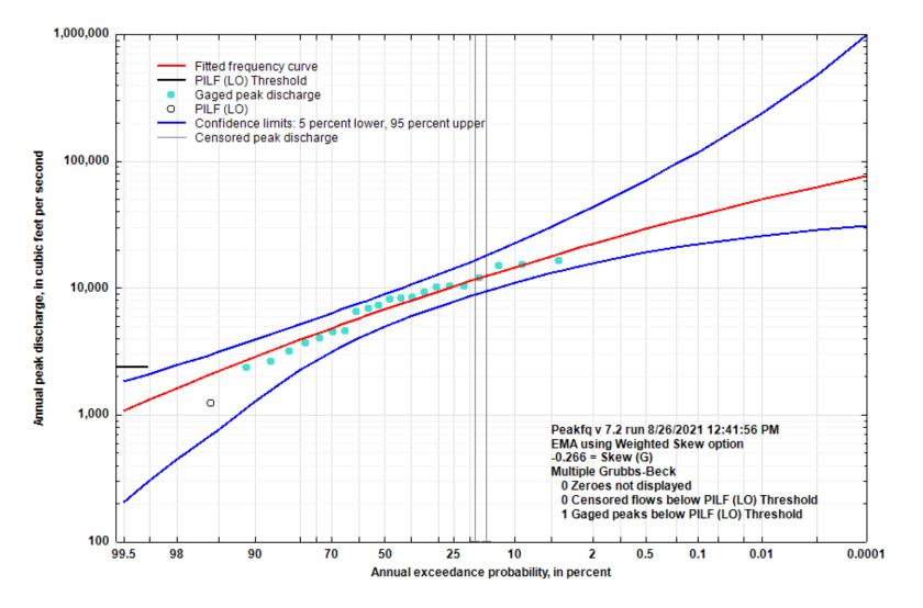
Figure 5-46. Flood Flow Frequency Curve for Tenmile Creek near Poplar Bluff, MO
