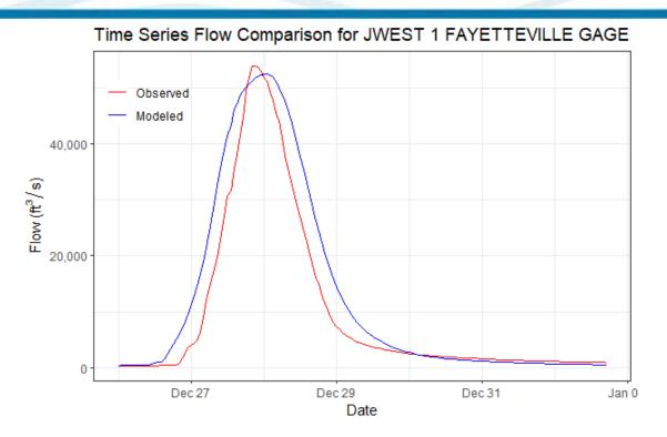
Figure 6-66. Calibration Results for JWEST 1 FAYETTEVILE GAGE HEC-HMS Junction – White River at Fayetteville, AR Gage (07048600, 2015 Event)
