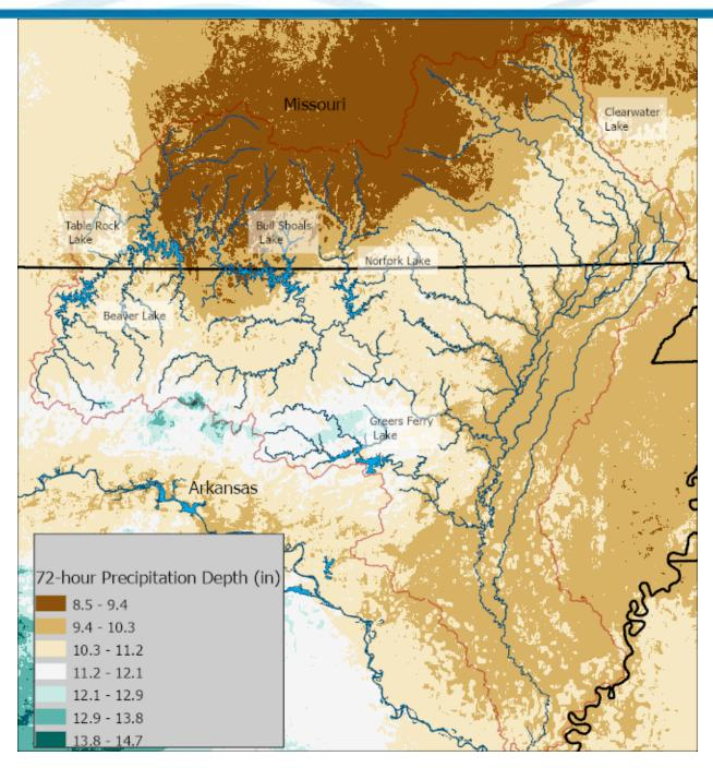
Figure 11-2 1/100 AEP, 72-hour precipitation depth isopluvial map from SWL precipitation frequency study
