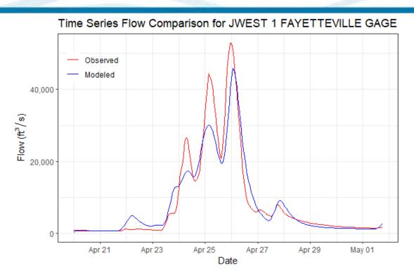
Figure 6-90. Calibration Results for JWEST 1 FAYETTEVILLE GAGE HEC-HMS Junction – White River at Fayetteville, AR Gage (07048600, 2011 Event)
