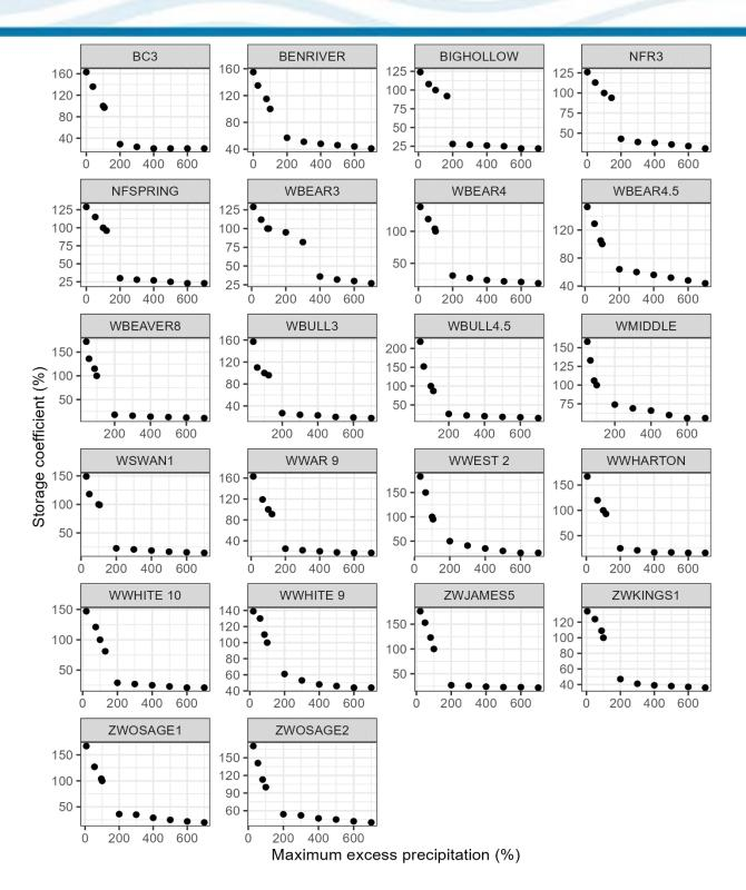
Figure 6-36. Plots showing R percentage and maximum excess precipitation percentage for subbasins used for creating Variable Clark curves.
