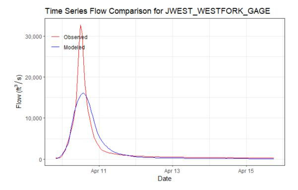
Figure 6-113. Validation Results for JWEST\_WESTFORK\_GAGE HEC-HMS Junction – West Fork of White River east of Fayetteville, AR Gage (2008 Event)
