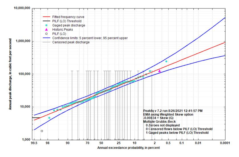
Figure 5-61. Flood Flow Frequency Curve for Spring River at Imboden, AR
