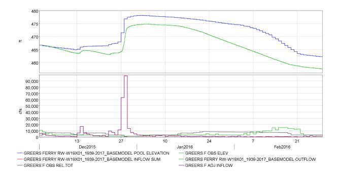
*Figure 8-6. Observed and modeled pool elevation for Greers Ferry Dam for Dec 2015 storm event.*
