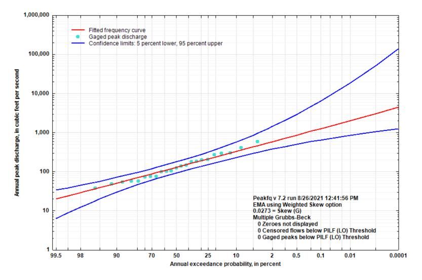
Figure 5-47. Flood Flow Frequency Curve for Fudge Hollow near Licking, MO
