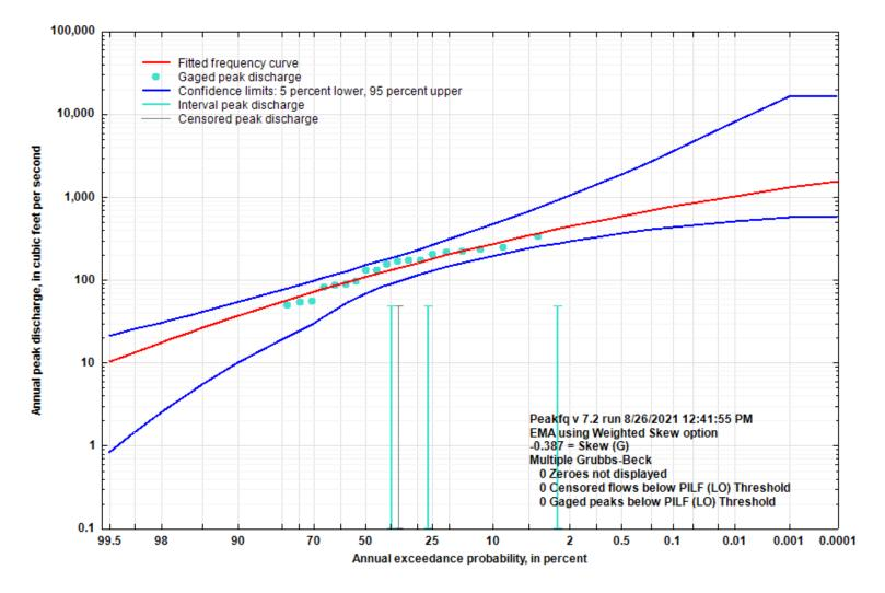
Figure 5-22. Flood Flow Frequency Curve for Gray Branch at Lutie, MO
