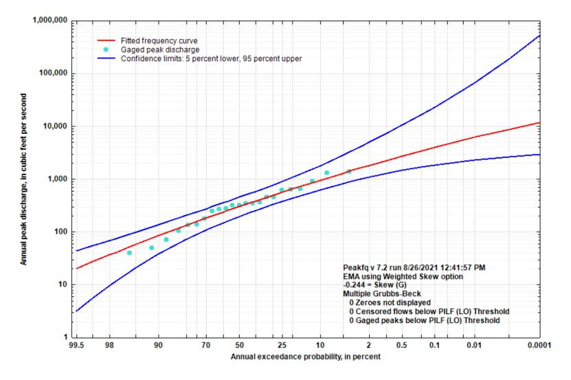
Figure 5-71. Flood Flow Frequency Curve for Tick Creek near Leslie, AR
