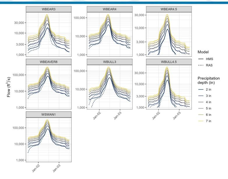
Figure 6-31. Plots showing HEC-RAS 2D and HEC-HMS calibration subbasins within Bull Shoals Lake Watershed
