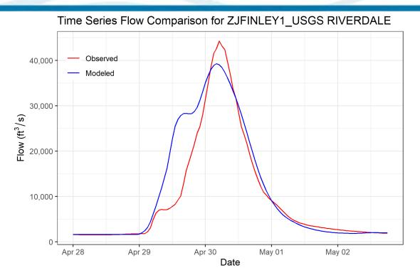
Figure 6-48. Calibration Results for ZJFINLEY1\_USGS RIVERDALE HEC-HMS Junction – Finley Creek below Riverdale, MO Gage (07052345, 2017 Event)
