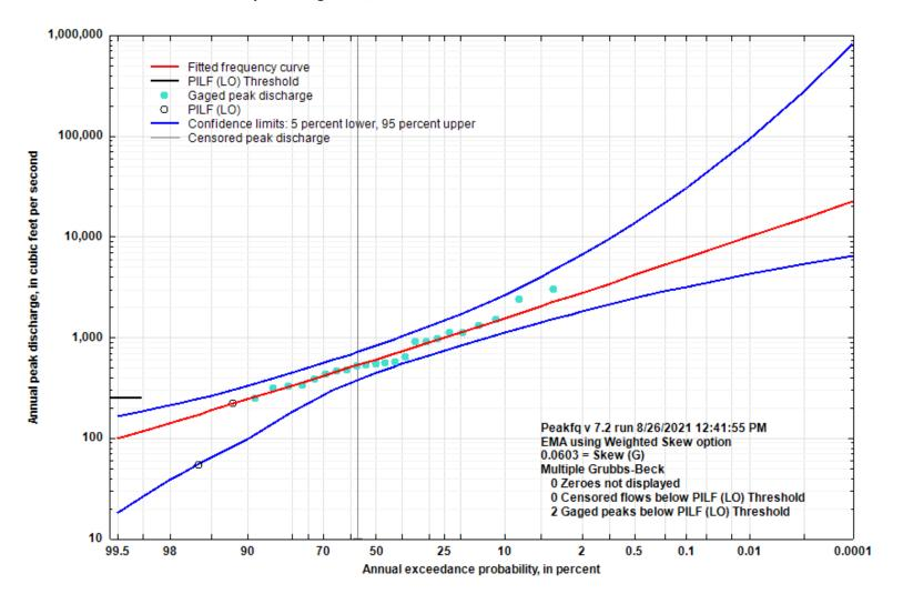
Figure 5-25. Flood Flow Frequency Curve for Crooked Creek Tributary near Dog Patch, AR
