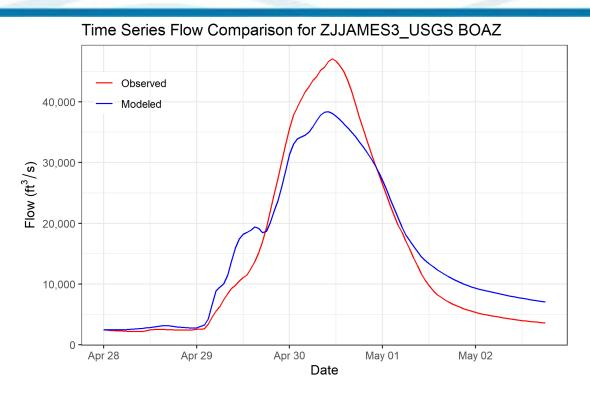
Figure 6-50. Calibration Results for ZJAMES3\_USGS BOAZ HEC-HMS Junction – James River near Boaz, MO Gage (07052250, 2017 Event)
