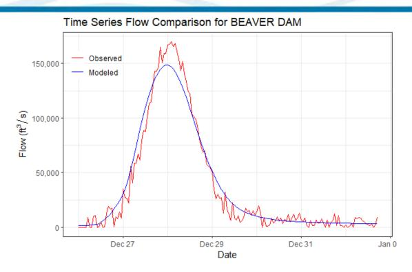
Figure 6-70. Calibration Results for BEAVER DAM HEC-HMS Junction – Flow at Beaver Dam (2015 Event)
