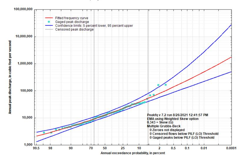
Figure 5-64. Flood Flow Frequency Curve for Eleven Point River near Ravenden Springs, AR
