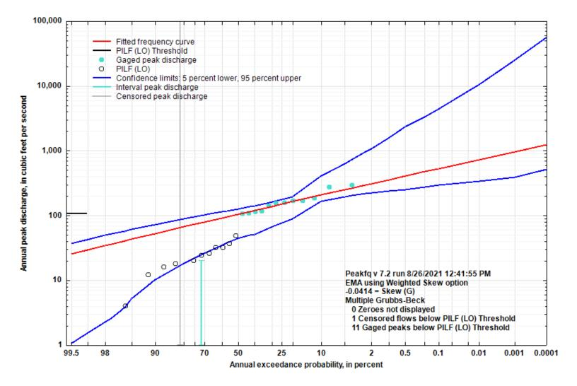
Figure 5-21. Flood Flow Frequency Curve for Yanell Branch near Kirbyville, MO
