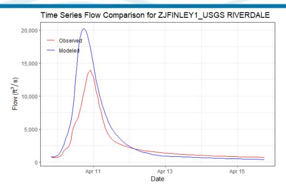
Figure 6-120. Validation Results for ZJFINLEY1\_USGS RIVERDALE HEC-HMS Junction – Finley Creek below Riverdale, MO Gage (2008 Event)
