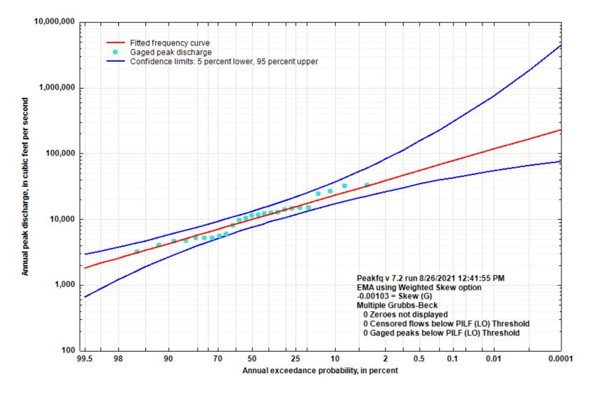
Figure 5-30. Flood Flow Frequency Curve for Richland Creek near Witts Spring, AR
