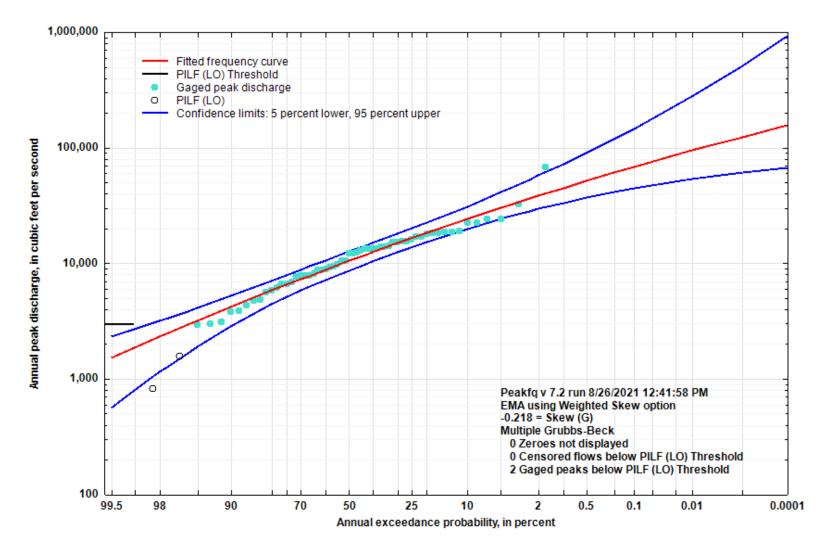
Figure 5-73. Flood Flow Frequency Curve for South Fork of Little Red River at Clinton, AR
