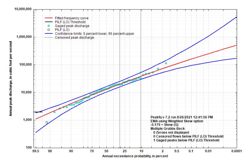
Figure 5-35. Flood Flow Frequency Curve for Bryant Creek near Tecumseh, MO
