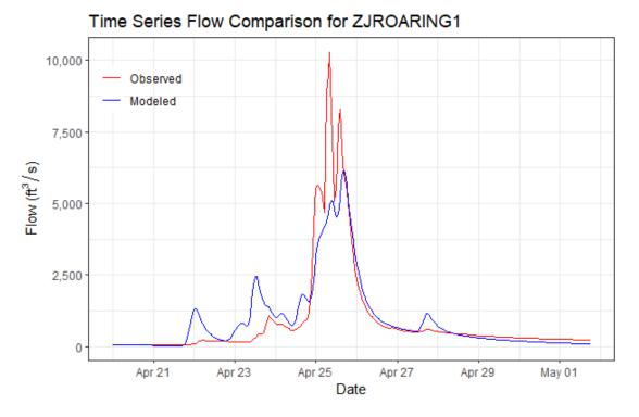
Figure 6-101. Calibration Results for ZJROARING1 HEC-HMS Junction – Roaring River at Roaring River State Park Gage (07050152, 2011 Event)
