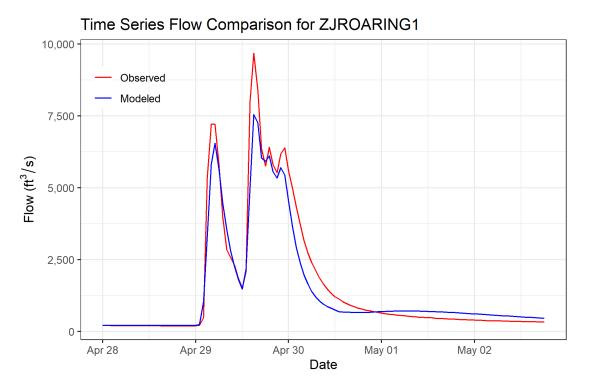
Figure 6-53. Calibration Results for ZJROARING1 HEC-HMS Junction – Roaring River at Roaring River State Park Gage (07050152, 2017 Event)
