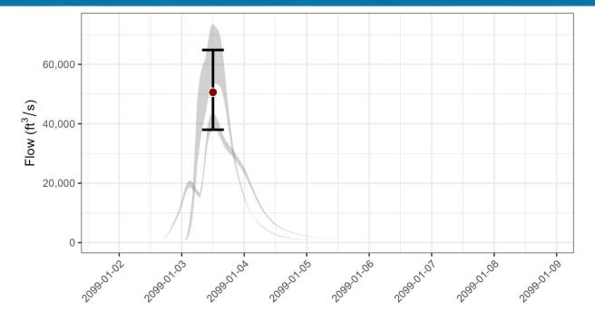
*Figure 10-11 Results from stochastic precipitation frequency for USGS 07053810*
