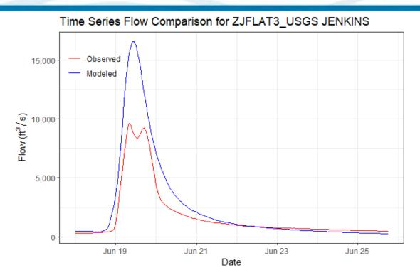
Figure 6-147. Validation Results for ZJFLAT3\_USGS JENKINS HEC-HMS Junction – Flat Creek below Jenkins, MO Gage (2015 Event)
