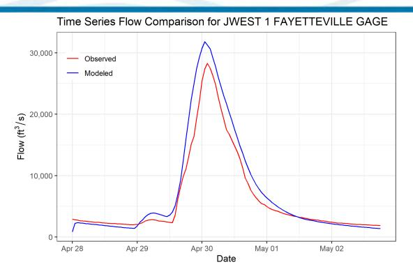
Figure 6-42. Calibration Results for JWEST 1 FAYETTEVILE GAGE HEC-HMS Junction – White River at Fayetteville, AR Gage (07048600, 2017 Event)
