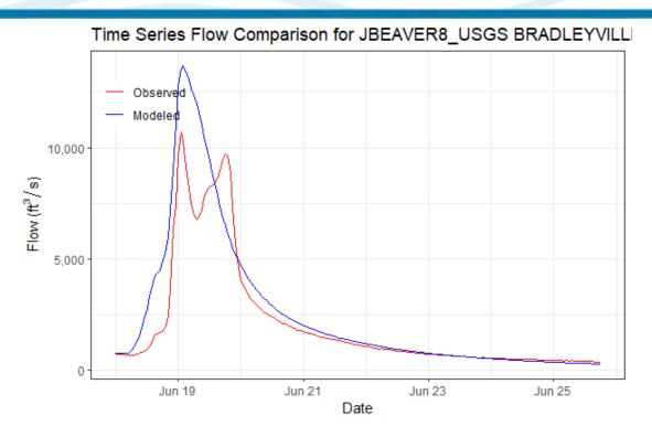
Figure 6-155. Validation Results for JBEAVER8 USGS BRADLEYVILLE HEC-HMS Junction -Beaver Creek at Bradleyville, MO Gage (2015 Event)
