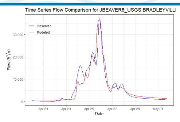
Figure 6-108. Calibration Results for JBEAVER8\_USGS BRADLEYVILLE HEC-HMS Junction – Beaver Creek at Bradleyville, MO Gage (07054080, 2011 Event)
