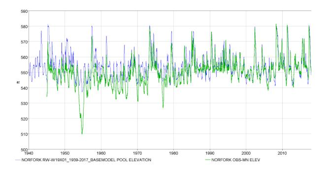
Figure 8-17. Observed and modeled pool elevation for Norfork Dam from 1940-2017.
