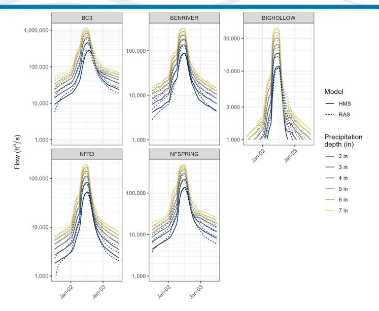
Figure 6-32. Plots showing HEC-RAS 2D and HEC-HMS calibration subbasins within Norfork Lake Watershed
