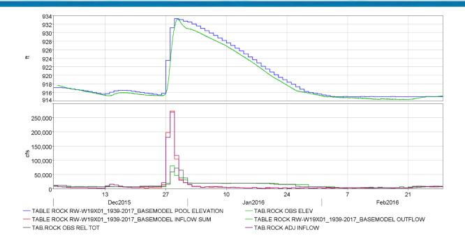
*Figure 8-3. Observed and modeled pool elevation for Table Rock Dam for Dec 2015 storm event.*
