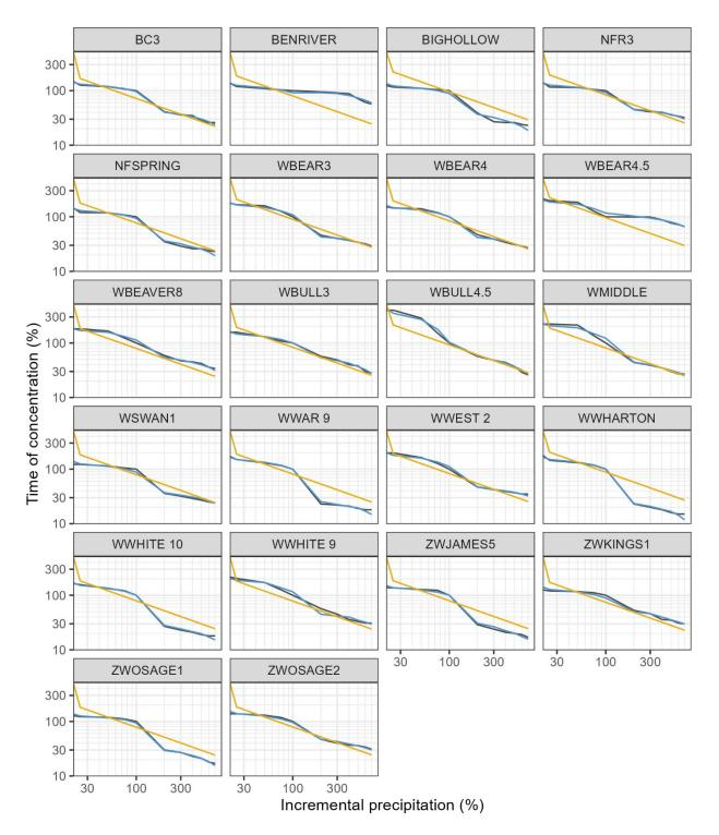
Figure 6-37. Plots showing calibrated Tc curves and predicted Tc curves from Cubist and from Ordinary Least Square (OLS) regression.
