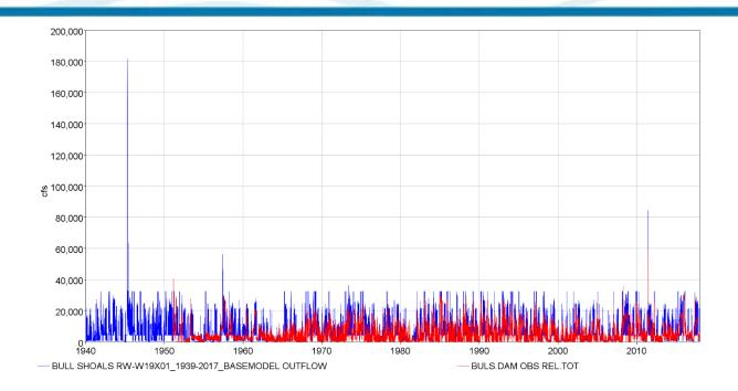
Figure 8-16. Observed and modeled outflow for Bull Shoals Dam from 1940-2017.
