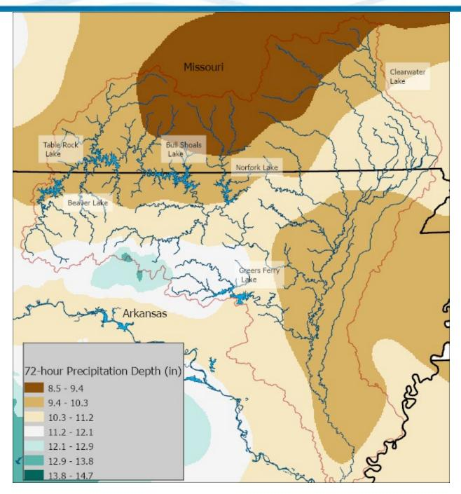
Figure 11-3 1/100 AEP, 72-hour precipitation depth isopluvial map from NOAA Atlas 14 Vol 8 and Vol 9
