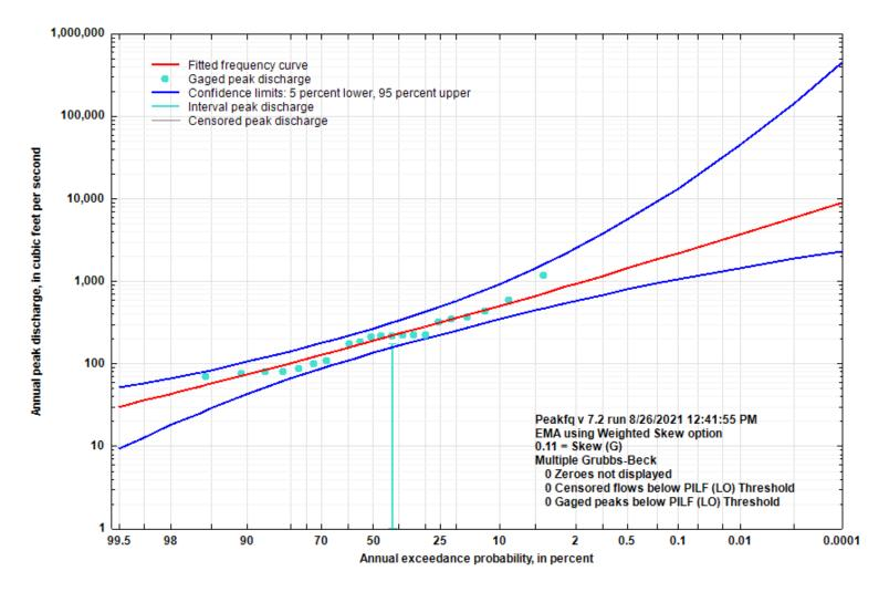
Figure 5-19. Flood Flow Frequency Curve for Ingenthron Hollow near Forsyth, MO
