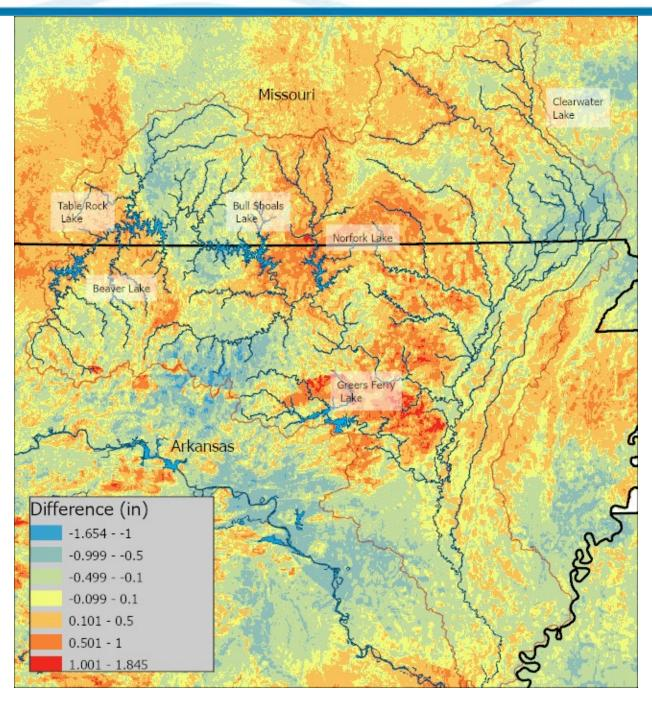
Figure 11-4. Difference between 72-hour SWL 1/100 AEP precipitation frequency depths and NOAA Atlas 14 1/100 AEP precipitation frequency depths
