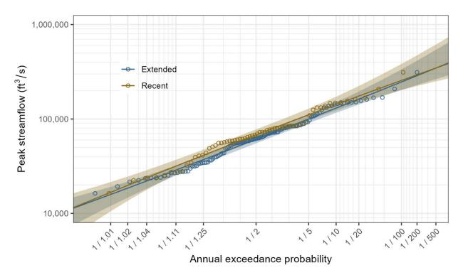
Figure 11-6 Comparison of regulated to extended period of record AEP streamflows for USGS 07061000 White River at Batesville AR
