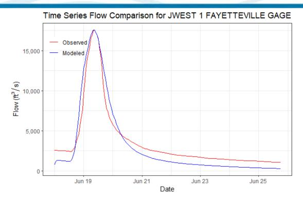
Figure 6-137. Validation Results for JWEST 1 FAYETTEVILLE GAGE HEC-HMS Junction – White River at Fayetteville, AR Gage (2015 Event)
