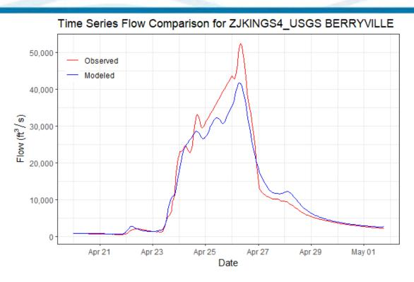
Figure 6-102. Calibration Results for ZJKINGS4 USGS BERRYVILLE HEC-HMS Junction – Kings River near Berryville, AR Gage (07050500, 2011 Event)
