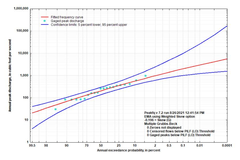
Figure 5-1. Flood Flow Frequency Curve for Dog Branch at St. Paul, AR
