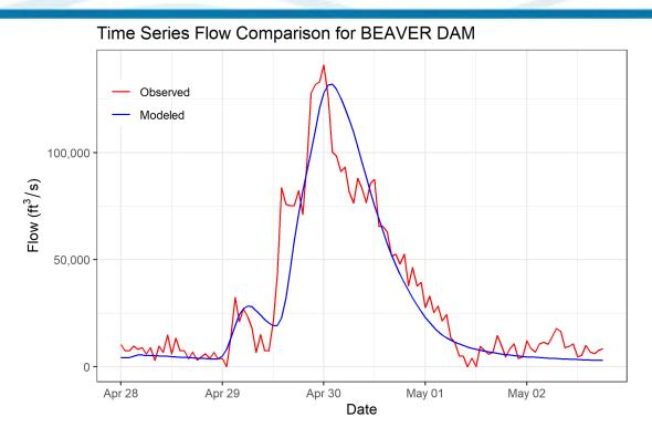
Figure 6-46. Calibration Results for BEAVER DAM HEC-HMS Junction – Flow at Beaver Dam (2017 Event)
