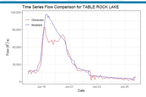
Figure 6-153. Validation Results for TABLE ROCK LAKE HEC-HMS Junction – Flow at Table Rock Lake (2015 Event)
