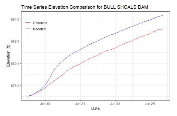
Figure 6-158. Validation Results for BULL SHOALS DAM HEC-HMS Junction – Elevation at Bull Shoals Lake Gage (2015 Event)
