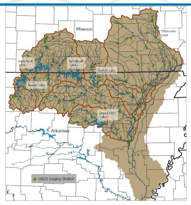
Figure 4-1. Map showing USGS streamflow gaging stations used for HEC-HMS model calibrations and HEC-HMS basin model boundaries and subbasins
