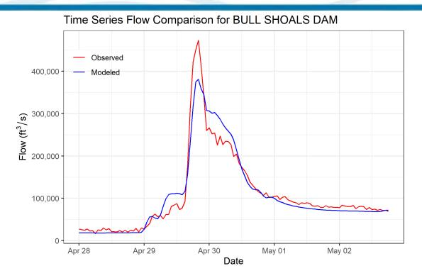
Figure 6-64. Calibration Results for BULL SHOALS DAM HEC-HMS Junction – Flow at Bull Shoals Dam (2017 Event)
