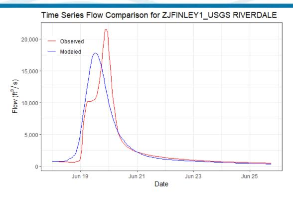
Figure 6-143. Validation Results for ZJFINLEY1\_USGS RIVERDALE HEC-HMS Junction – Finley Creek below Riverdale, MO Gage (2015 Event)
