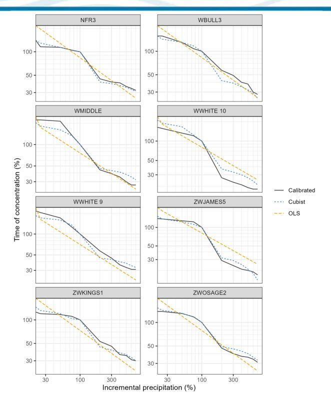
Figure 6-25. Plots showing results, in percentages, for LOOCV for Tc
