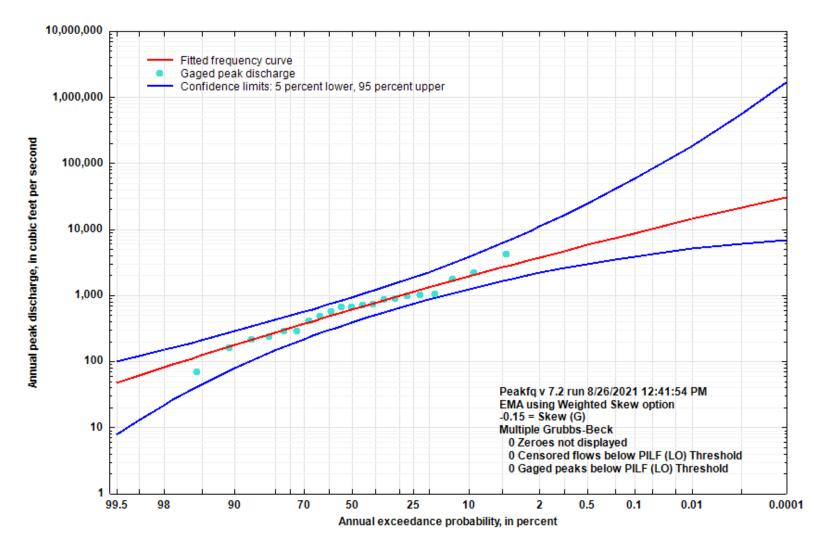
Figure 5-6. Flood Flow Frequency Curve for Maxwell Creek at Kingston, AR
