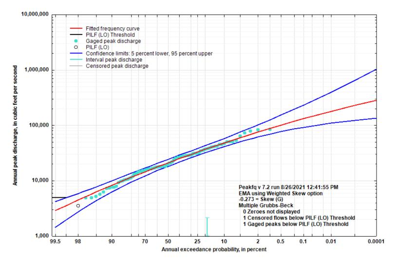
Figure 5-15. Flood Flow Frequency Curve for James River at Galena, MO
