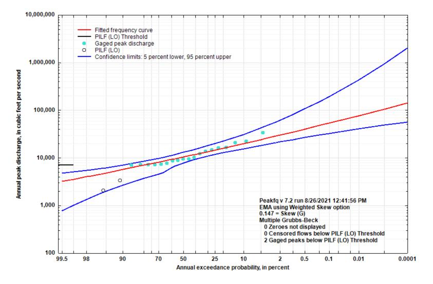
Figure 5-32. Flood Flow Frequency Curve for Bear Creek near Silver Hill, AR
