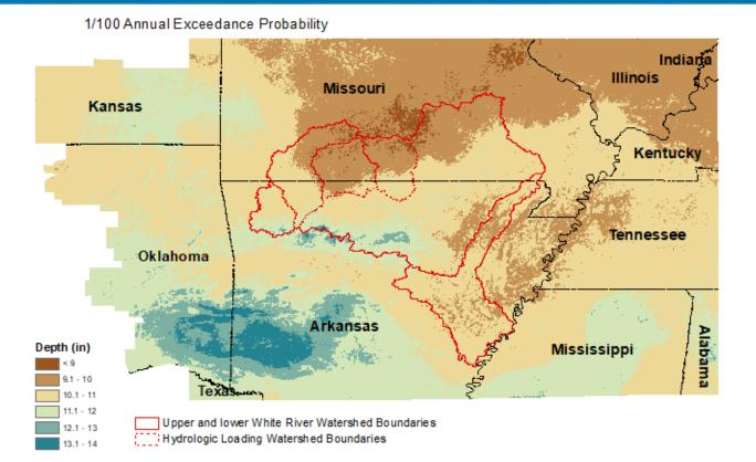
Figure 7-6. 1/100 AEP, 72-hour precipitation depths for the White River basin in AR and MO from SWL precipitation frequency study
