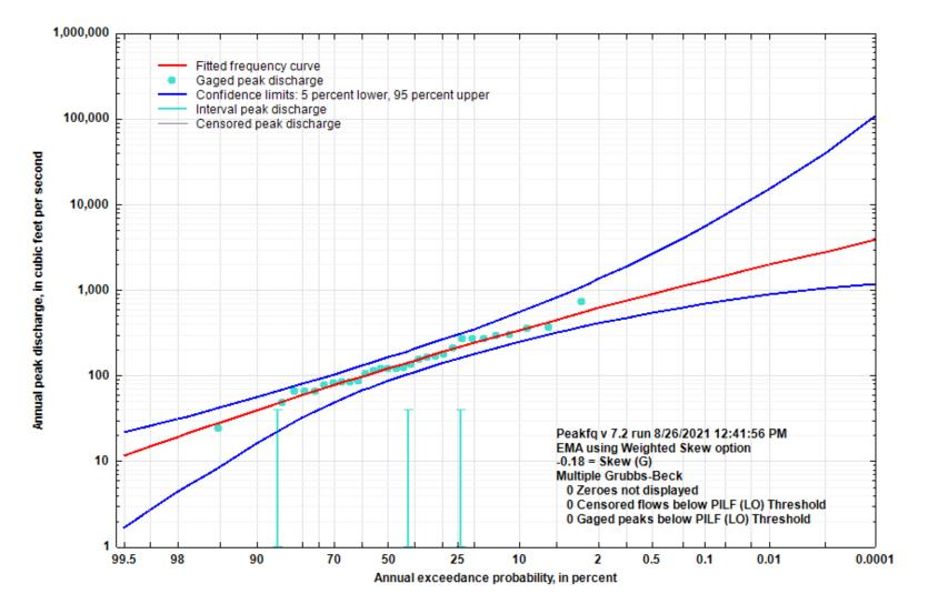
Figure 5-52. Flood Flow Frequency Curve for Sycamore Creek near Winona, MO
