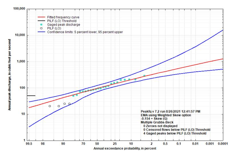
Figure 5-70. Flood Flow Frequency Curve for Trace C Trib nr Marshall, Ark
