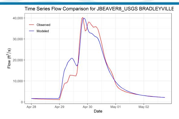
Figure 6-60. Calibration Results for JBEAVER8\_USGS BRADLEYVILLE HEC-HMS Junction – Beaver Creek at Bradleyville, MO Gage (07054080, 2017 Event)
