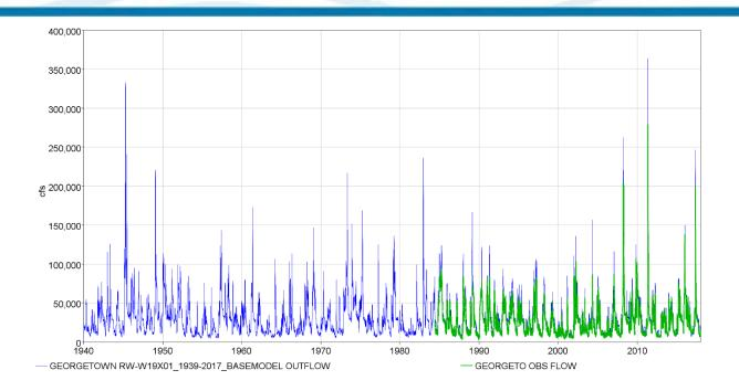
Figure 8-24. Observed and modeled flow at Georgetown from 1940-2017.
