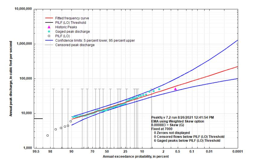
Figure 5-5. Flood Flow Frequency Curve for War Eagle Creek near Hindsville, AR
