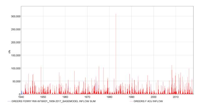
Figure 8-21. Observed and modeled inflow for Greers Ferry Dam from 1940-2017.
