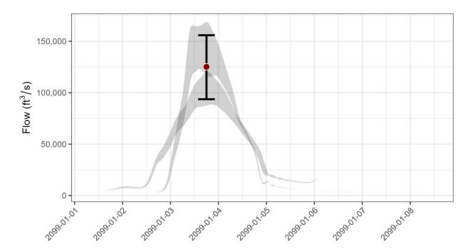
Figure 10-8 Results from stochastic precipitation frequency for USGS 07052500
