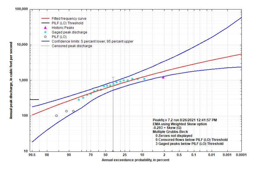
Figure 5-68. Flood Flow Frequency Curve for Dry Branch Tributary near Sidney, AR
