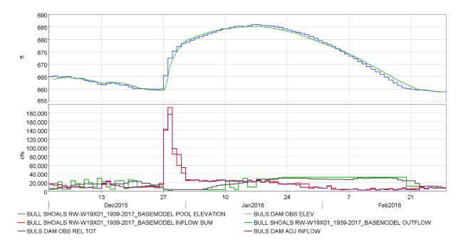
*Figure 8-4. Observed and modeled pool elevation for Bull Shoals Dam for Dec 2015 storm event.*
