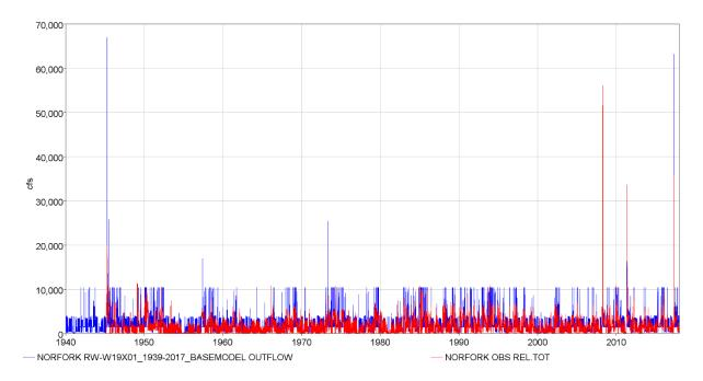
Figure 8-19. Observed and modeled releases for Norfork Dam from 1940-2017.
