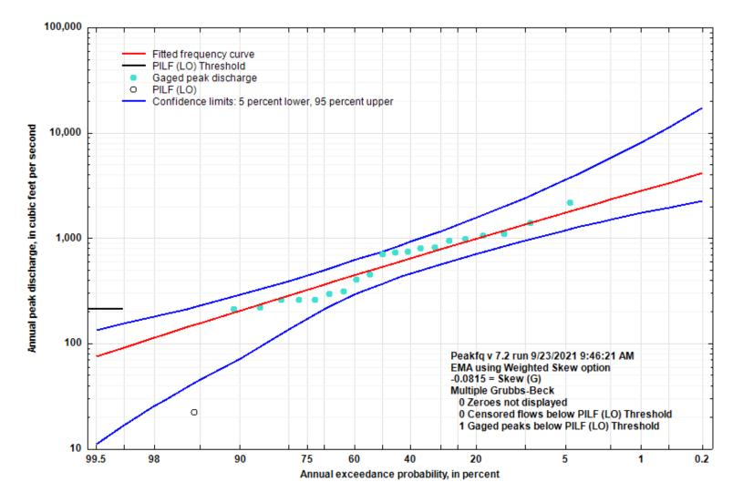
Figure 5-60. Flood Flow Frequency Curve for Miller Creek near Salem, AR
