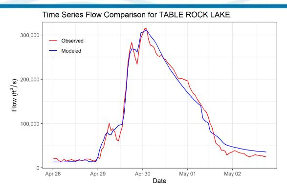
Figure 6-58. Calibration Results for TABLE ROCK LAKE HEC-HMS Junction – Flow at Table Rock Lake (2017 Event)
