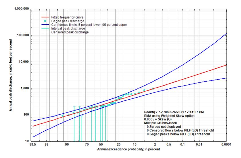
Figure 5-59. Flood Flow Frequency Curve for Brush Creek near Mammoth Spring, AR
