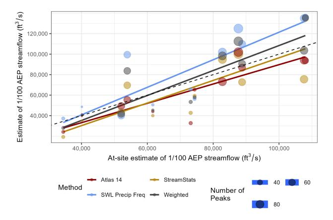
Figure 11-1 Comparison of at-site estimates of 1/100 AEP peak streamflows vs other methods of computing 1/100 AEP peak streamflows for selected gaged locations within the White River basin
