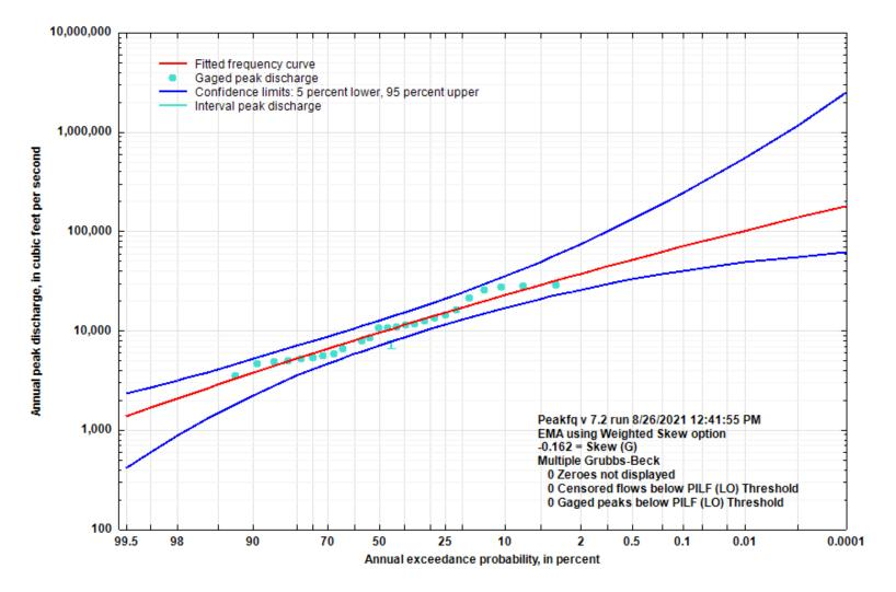
Figure 5-27. Flood Flow Frequency Curve for Buffalo River near Boxley, AR
