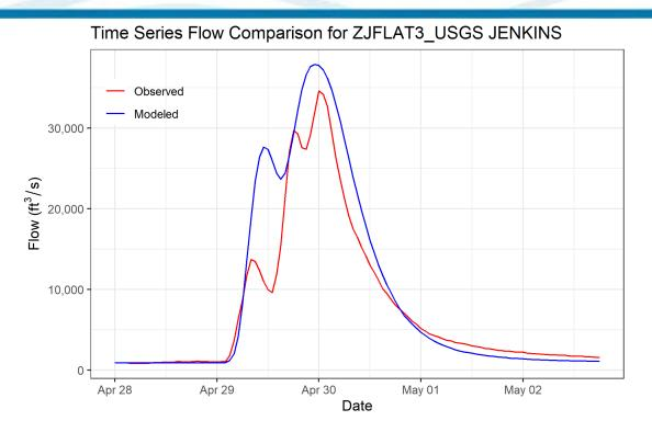
Figure 6-52. Calibration Results for ZJFLAT3\_USGS JENKINS HEC-HMS Junction – Flat Creek below Jenkins, MO Gage (07052820, 2017 Event)
