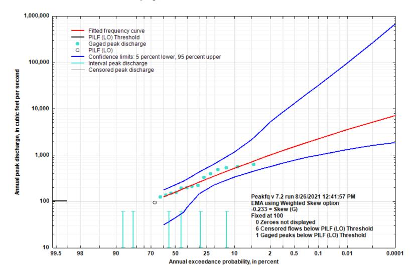
Figure 5-62. Flood Flow Frequency Curve for Burnham Branch near Willow Springs, MO
