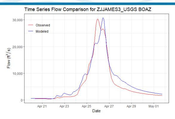
Figure 6-98. Calibration Results for ZJJAMES3\_USGS BOAZ HEC-HMS Junction – James River near Boaz, MO Gage (07052250, 2011 Event)
