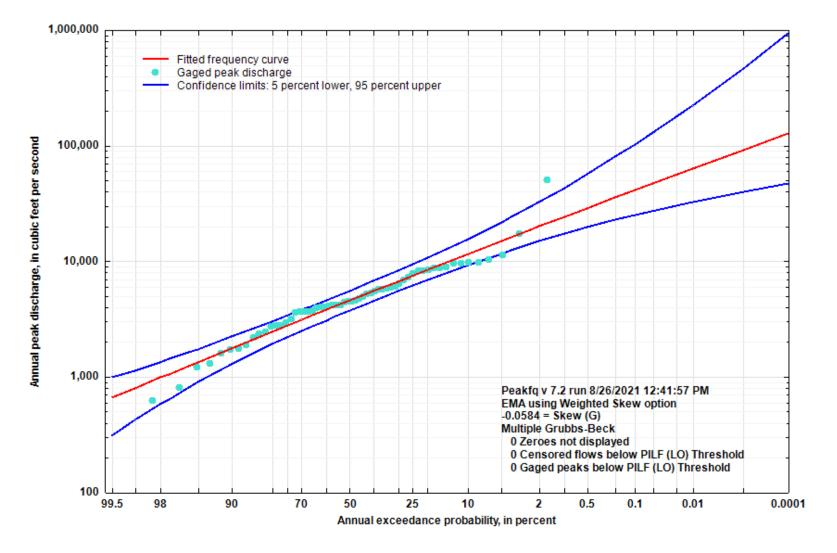
Figure 5-66. Flood Flow Frequency Curve for Piney Fork at Evening Shade
