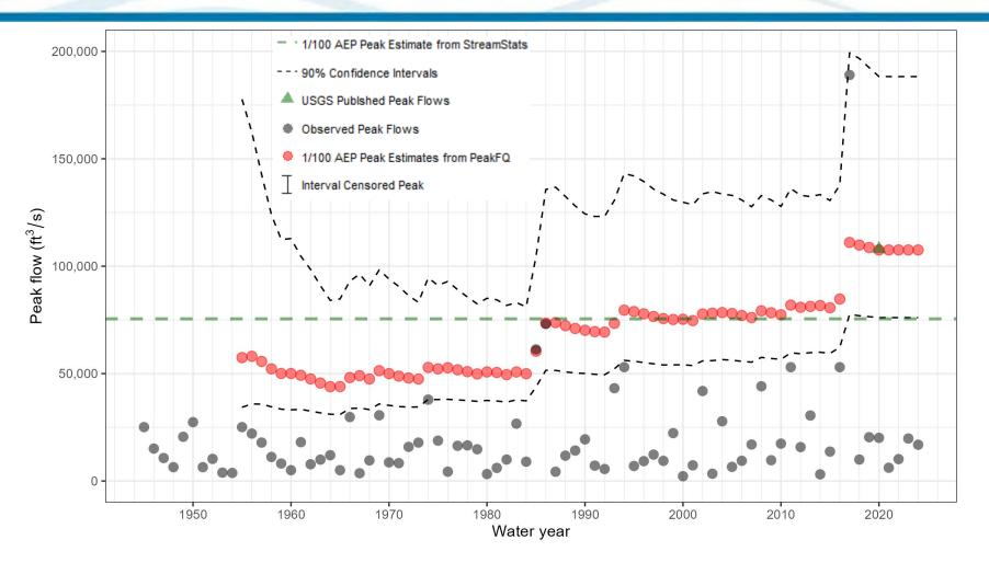
Figure 5-83. Change in 100-Year Flow over Time for North Fork River near Tecumseh, MO (07057500)
