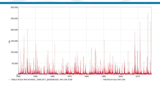
Figure 8-12. Observed and modeled inflow for Table Rock Dam from 1940-2017.
