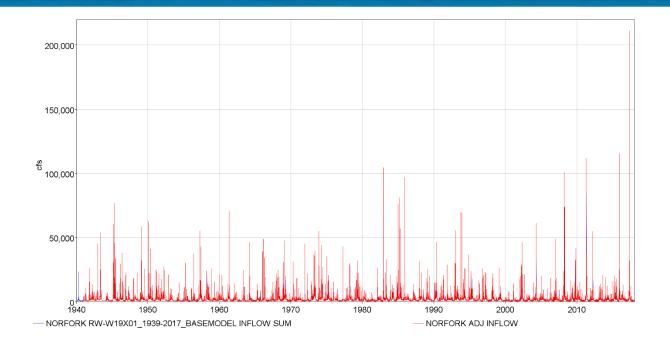
Figure 8-18. Observed and modeled inflow for Norfork Dam from 1940-2017.
