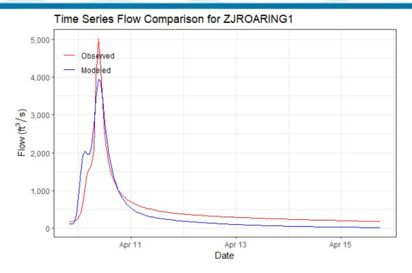
Figure 6-124. Validation Results for ZJROARING1 HEC-HMS Junction – Roaring River at Roaring River State Park Gage (2008 Event)
