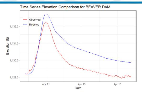
Figure 6-118. Validation Results for BEAVER DAM HEC-HMS Junction – Flow at Beaver Dam (2008 Event)
