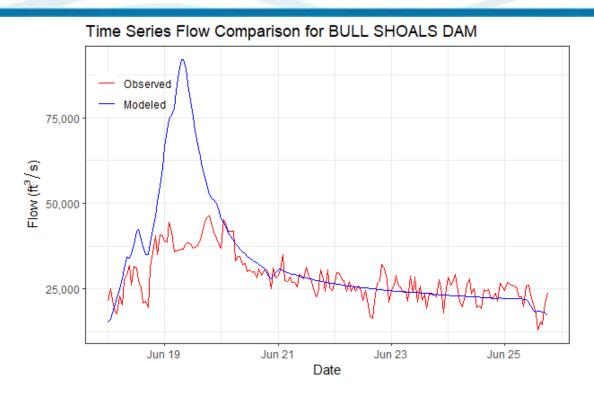
Figure 6-159. Validation Results for BULL SHOALS DAM HEC-HMS Junction – Flow at Bull Shoals Lake Gage (2015 Event)
