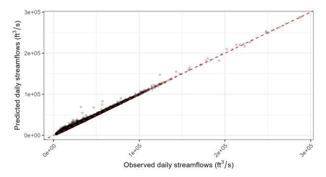
*Figure 5-90. Observed and bias corrected predicted daily streamflows for the regulated period of record for White River at Newport*
