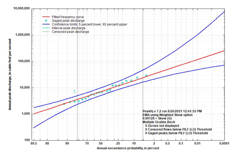
Figure 5-16. Flood Flow Frequency Curve for Long Creek at Denver, AR
