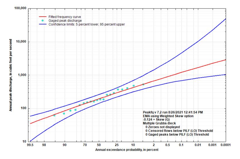
Figure 5-7. Flood Flow Frequency Curve for Freeman Branch at Berryville, AR
