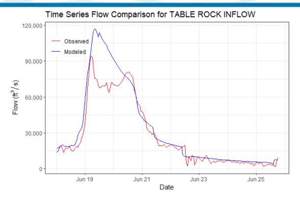
Figure 6-151. Validation Results for TABLE ROCK INFLOW HEC-HMS Junction – Inflow to Table Rock Lake (2015 Event)
