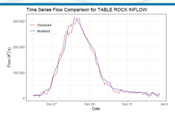
Figure 6-80. Calibration Results for TABLE ROCK INFLOW HEC-HMS Junction – Inflow to Table Rock Lake (2015 Event)
