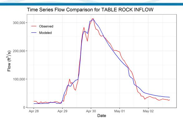
Figure 6-56. Calibration Results for TABLE ROCK INFLOW HEC-HMS Junction – Inflow to Table Rock Lake (2017 Event)
