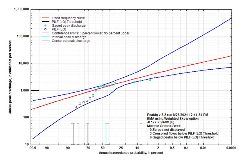
Figure 5-9. Flood Flow Frequency Curve for North Carolina Creek near Marshfield, MO
