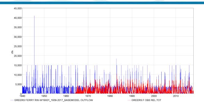
Figure 8-22. Observed and modeled releases for Greers Ferry Dam from 1940-2017.
