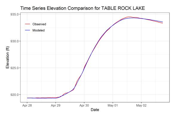
Figure 6-57. Calibration Results for TABLE ROCK LAKE HEC-HMS Junction – Elevation at Table Rock Lake (2017 Event)
