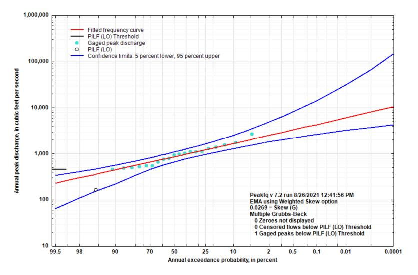
Figure 5-39. Flood Flow Frequency Curve for Hughes Creek near Mountain View, AR
