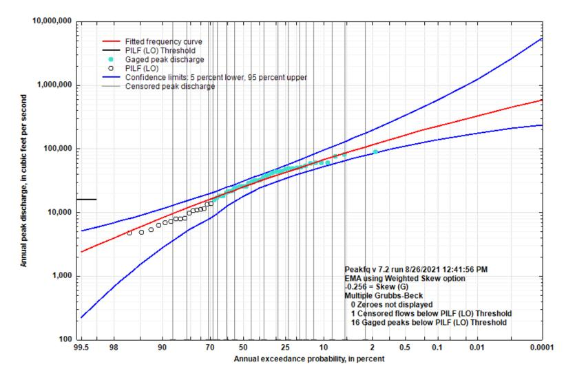
Figure 5-51. Flood Flow Frequency Curve for Current River at Eminence, MO
