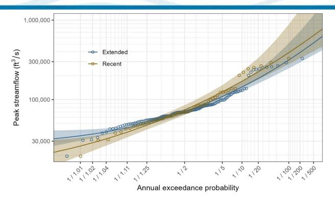
Figure 11-5 Comparison of regulated to extended period of record AEP streamflows for USGS 07074500 White River at Newport AR
