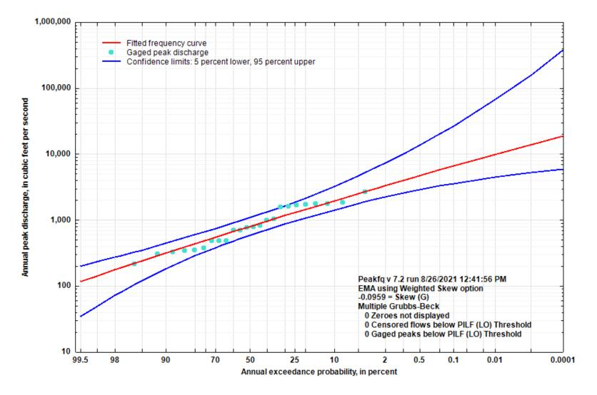
Figure 5-42. Flood Flow Frequency Curve for Gibbs Creek at Sulphur Rock, AR
