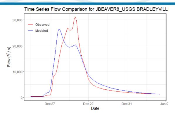
Figure 6-84. Calibration Results for JBEAVER8\_USGS BRADLEYVILLE HEC-HMS Junction – Beaver Creek at Bradleyville, MO Gage (07054080, 2015 Event)
