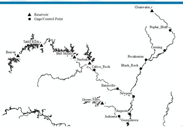
Figure 8-1. Norfork, White, and Black Rivers showing reservoir (triangles) and important gages (circles) used in hydrology update of the White River RiverWare period of record model.
