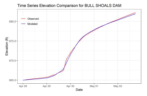
Figure 6-63. Calibration Results for BULL SHOALS DAM HEC-HMS Junction – Elevation at Bull Shoals Lake (2017 Event)
