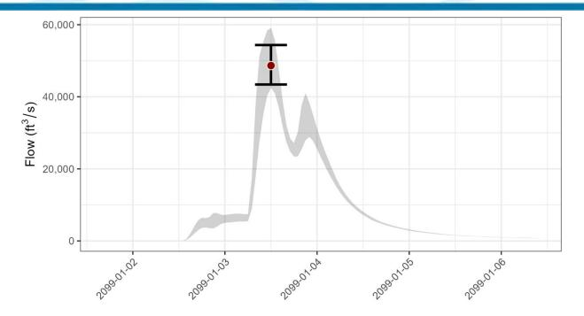
*Figure 10-9 Results from stochastic precipitation frequency for USGS 07053207*
