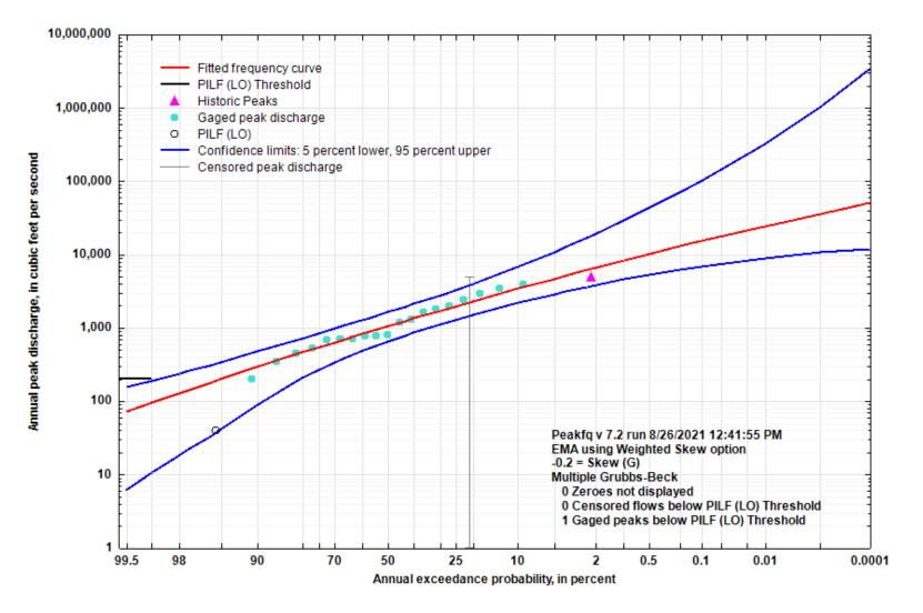
Figure 5-29. Flood Flow Frequency Curve for Dry Branch near Vendor, AR
