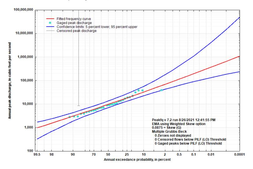
Figure 5-26. Flood Flow Frequency Curve for Crooked Creek at Kelly Crossing at Yellville, AR
