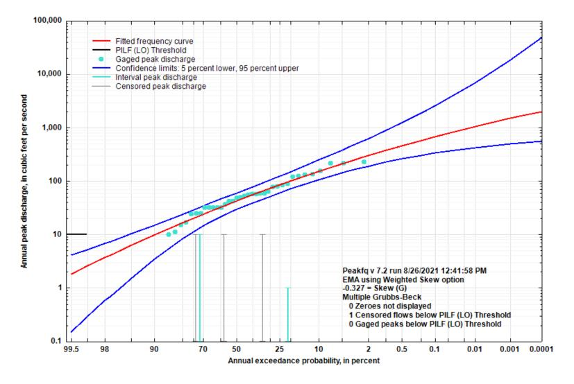
Figure 5-75. Flood Flow Frequency Curve for Dill Branch Tributary near Ida, AR
