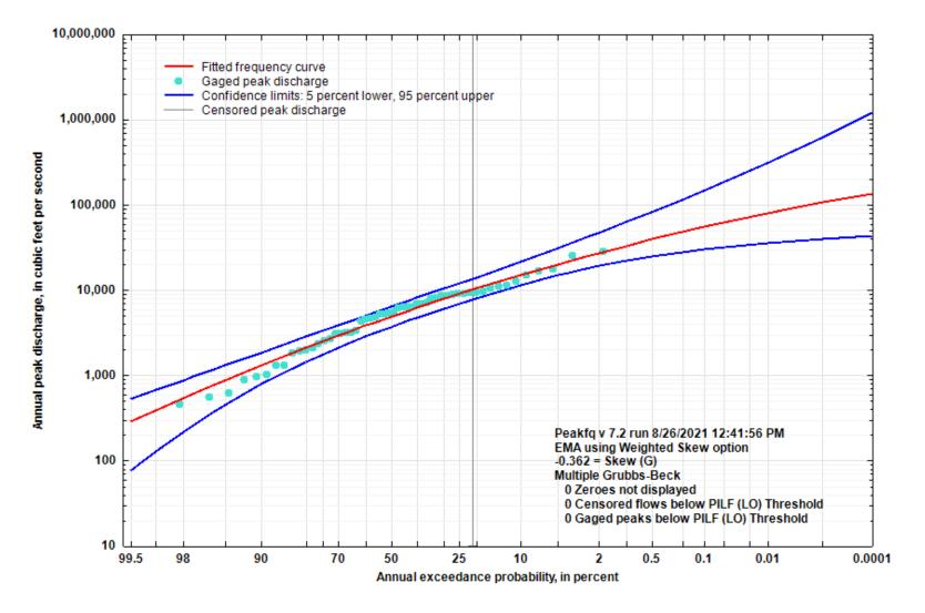
Figure 5-40. Flood Flow Frequency Curve for North Sylamore Creek near Fifty Six, AR
