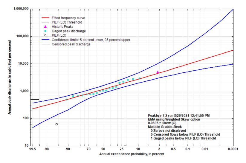
Figure 5-23. Flood Flow Frequency Curve for Charley Creek near Omaha, AR
