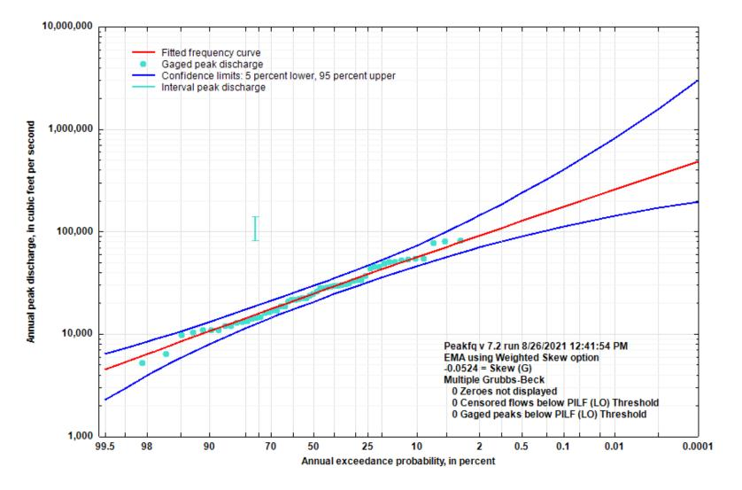
Figure 5-3. Flood Flow Frequency Curve for White River near Fayetteville, AR
