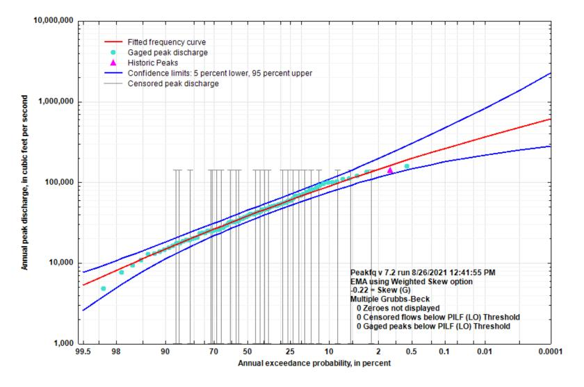
Figure 5-31. Flood Flow Frequency Curve for Buffalo River near St. Joe, AR
