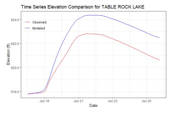
Figure 6-152. Validation Results for TABLE ROCK LAKE HEC-HMS Junction – Elevation at Table Rock Lake (2015 Event)
