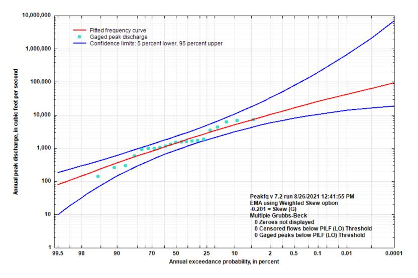
Figure 5-28. Flood Flow Frequency Curve for Smith Creek near Boxley, AR
