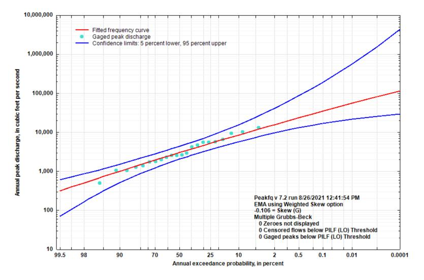
Figure 5-4. Flood Flow Frequency Curve for War Eagle Creek near Witter, AR
