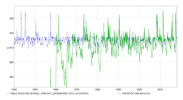
Figure 8-11. Observed and modeled pool elevation for Table Rock Dam from 1940-2017.
