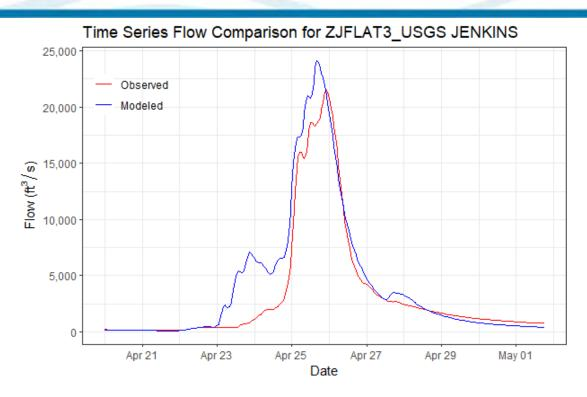
Figure 6-100. Calibration Results for ZJFLAT3\_USGS JENKINS HEC-HMS Junction – Flat Creek below Jenkins, MO Gage (07052820, 2011 Event)
