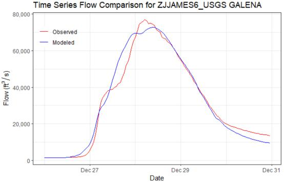
Figure 6-75. Calibration Results for ZJJAMES6\_USGS GALENA HEC-HMS Junction – James River near Galena, MO Gage (07052500, 2015 Event)
