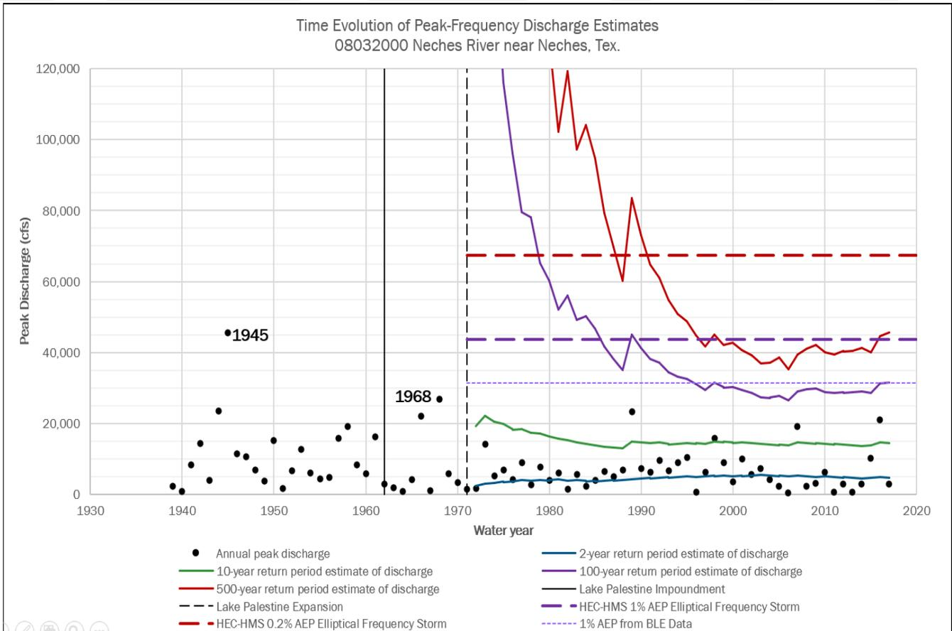
Figure 11.1b: Statistical Change Over Time Comparison for the Neches River nr Neches, TX
