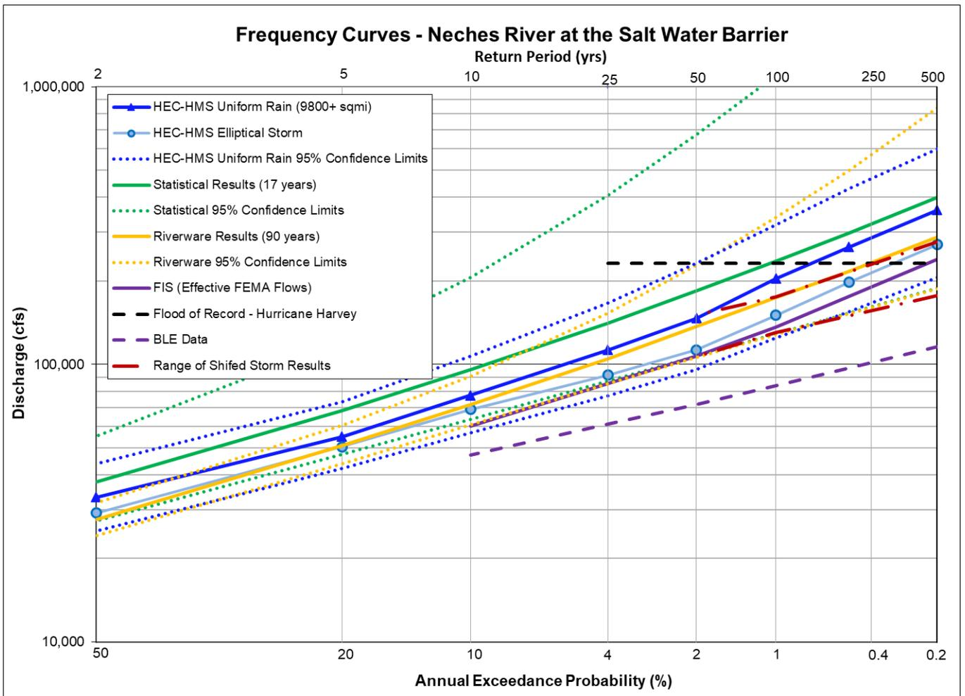
**Figure 11.16a: Flow Frequency Curve Comparison for the Neches River at the Saltwater Barrier, TX**
