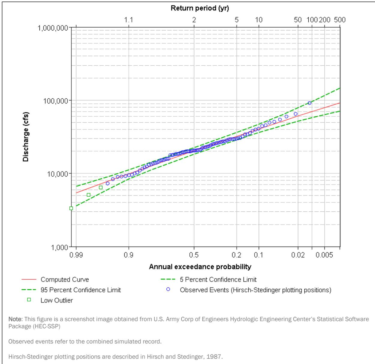
**Figure 8.16: Simulated Flood Flow Frequency using log-Pearson Type III Distribution for USGS Streamgaging Station 08040600 Neches River near Town Bluff, Tex.**
