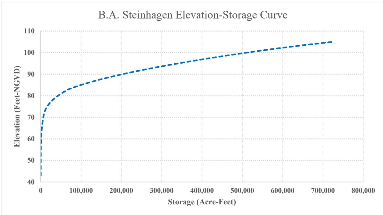
Figure 9.17: B.A. Steinhagen Lake Storage-Elevation Curve
