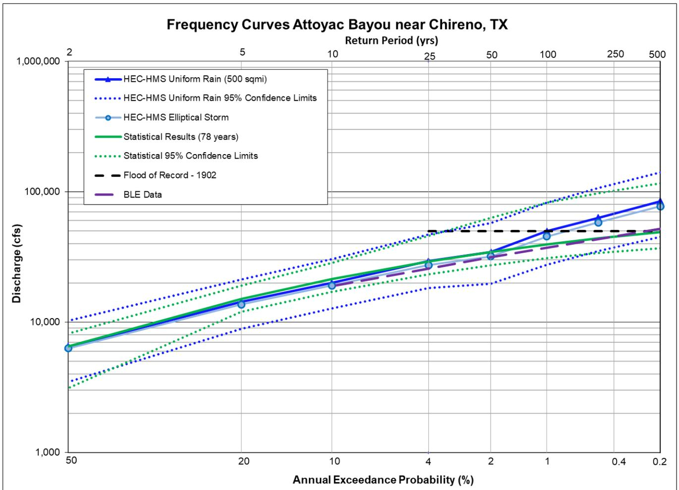
**Figure 11.8a: Flow Frequency Curve Comparison for Attoyac Bayou near Chireno, TX**
