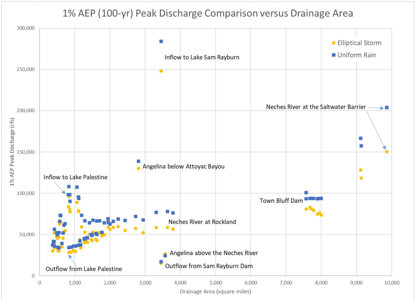
Figure 7.22: Elliptical Storm versus Uniform Rain HEC-HMS Peak Flow Results for the 1% ACE (100-yr)
