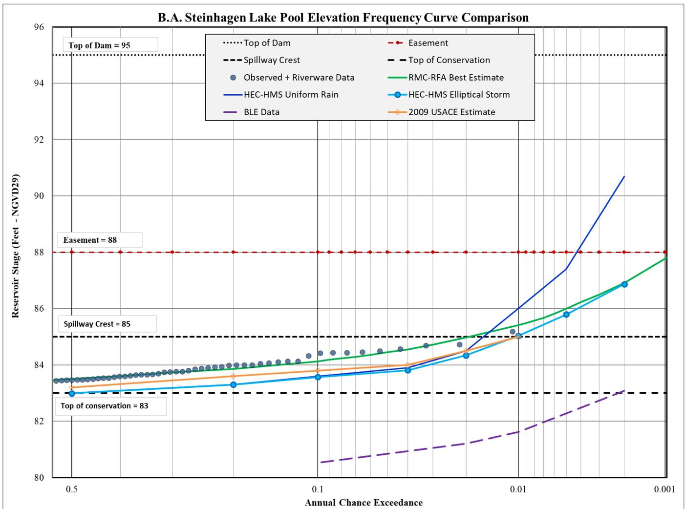
**Figure 11.18: Pool Elevation Frequency Curve Comparison for B.A. Steinhagen Lake**
