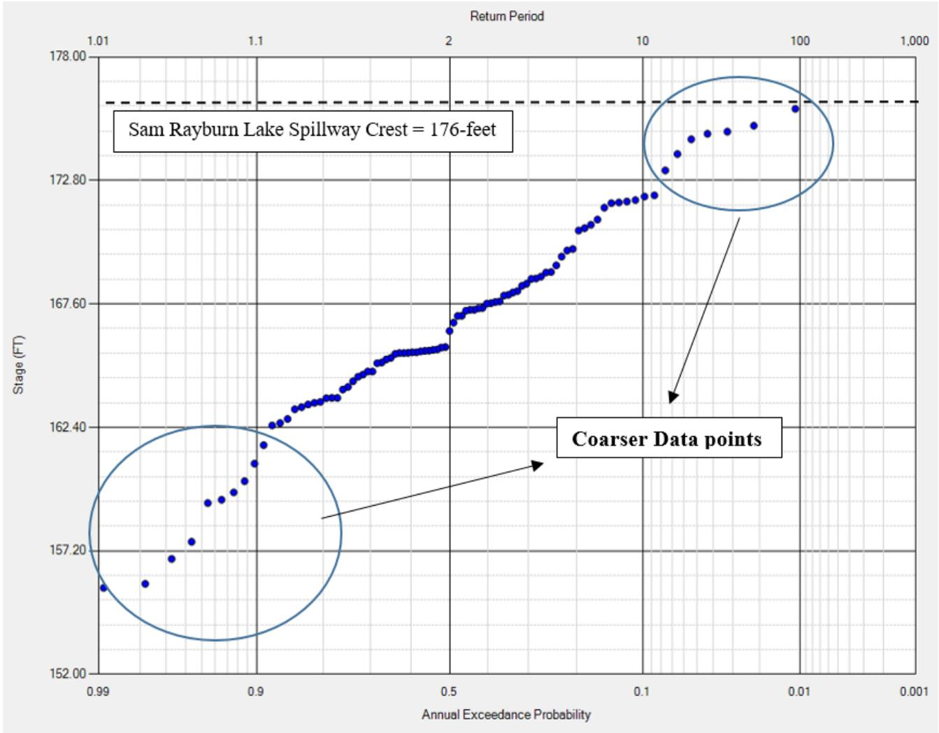
Figure 9.12: Empirical Stage Frequency for Sam Rayburn Reservoir
