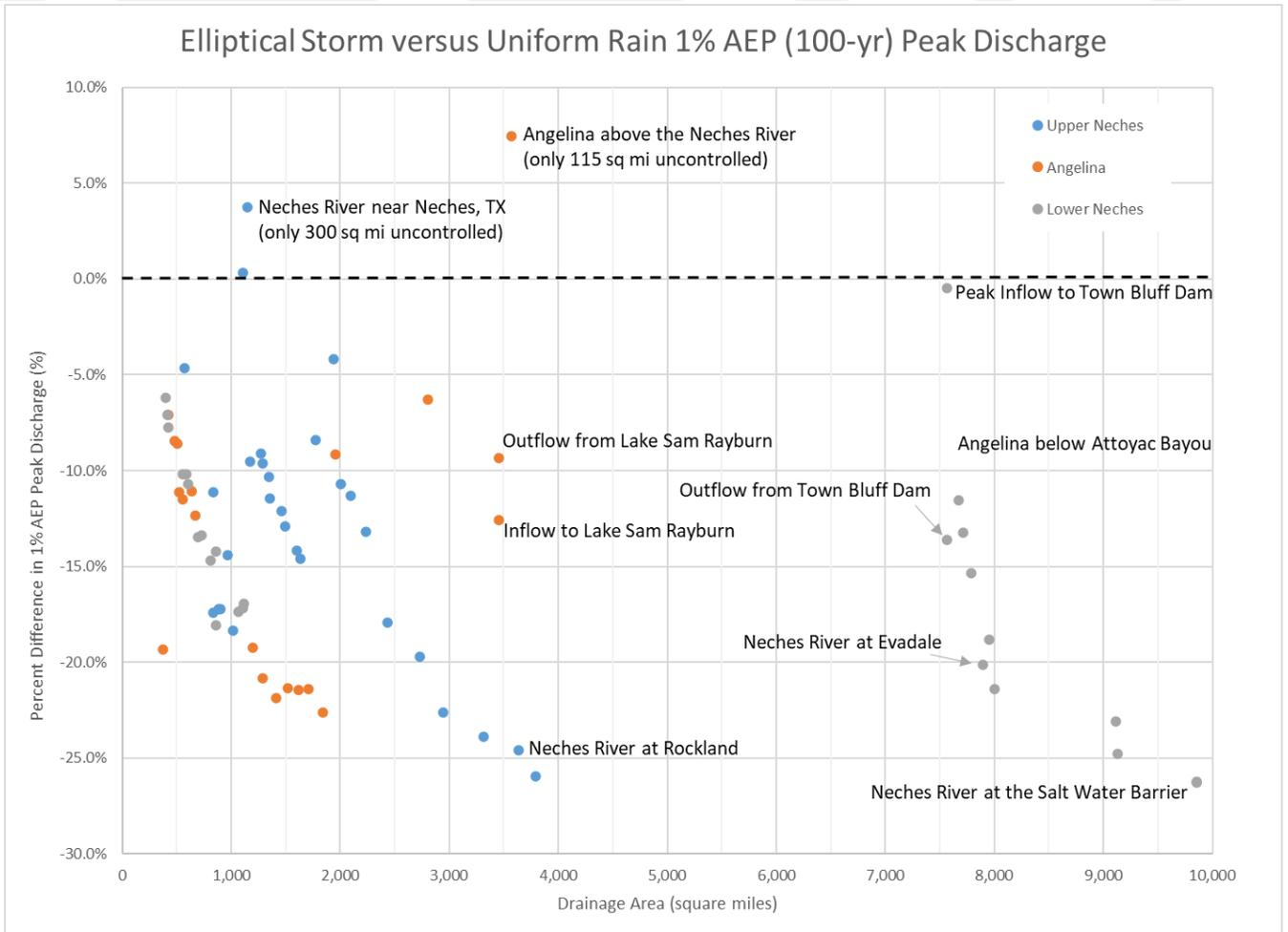
Figure 7.21: Elliptical Storm versus Uniform Rain HEC-HMS Difference in Peak Flow for the 1% ACE (100-yr)
