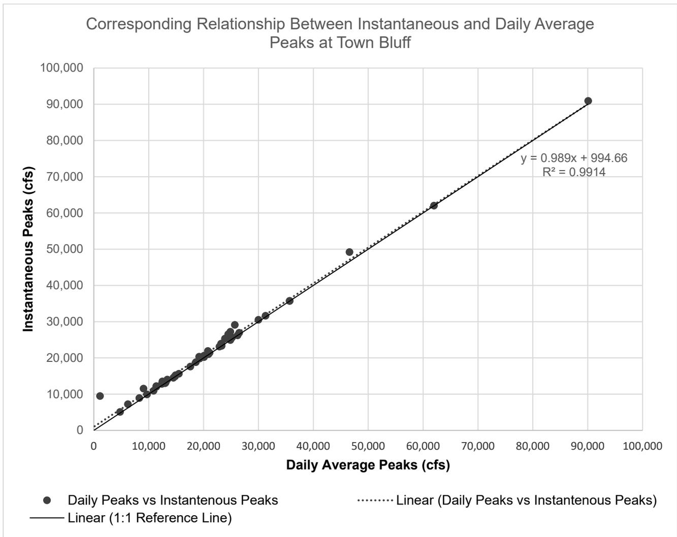
Figure 8.11: Instantaneous vs. Daily Average Peak Discharges for USGS Streamgaging Station 08040600 Neches River near Town Bluff, Tex.
