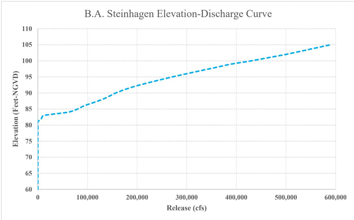
Figure 9.16: B.A. Steinhagen Lake Outflow Elevation-Discharge Curve
