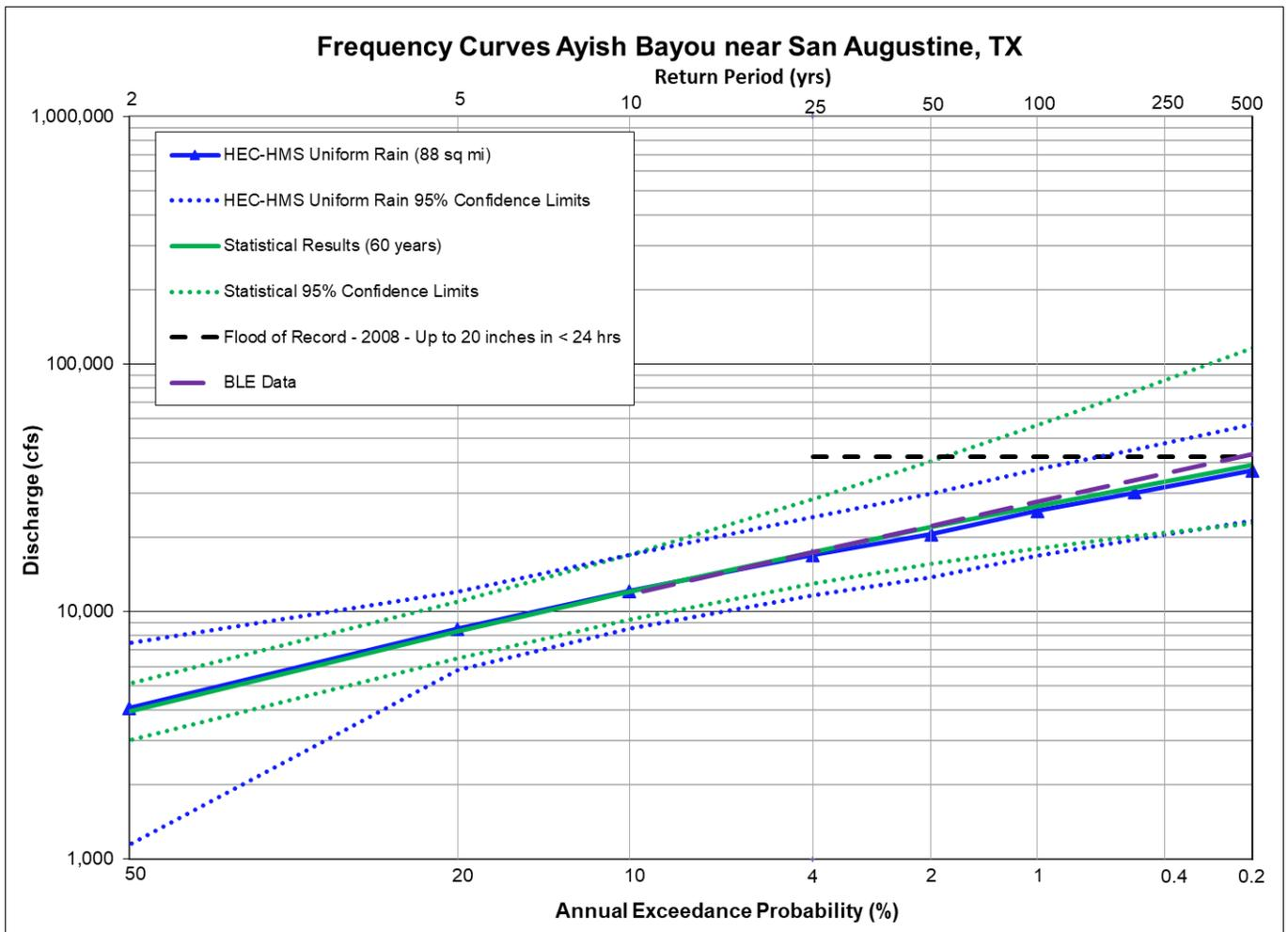
**Figure 11.9: Flow Frequency Curve Comparison for the Ayish Bayou nr San Augustine, TX**
