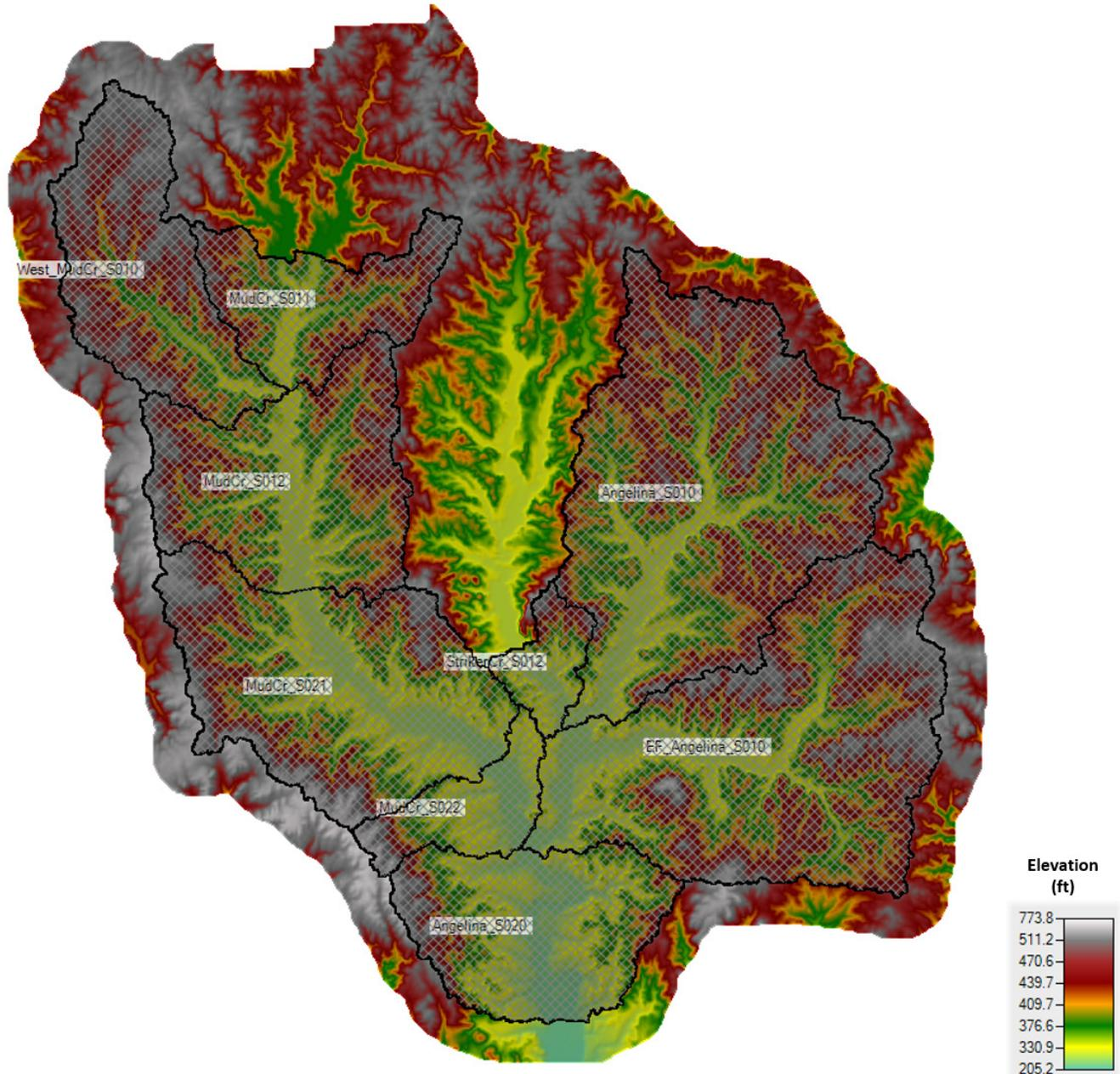
Figure 10.3: Overall Terrain Model and 2D Computational Mesh with Nine Flow Areas
