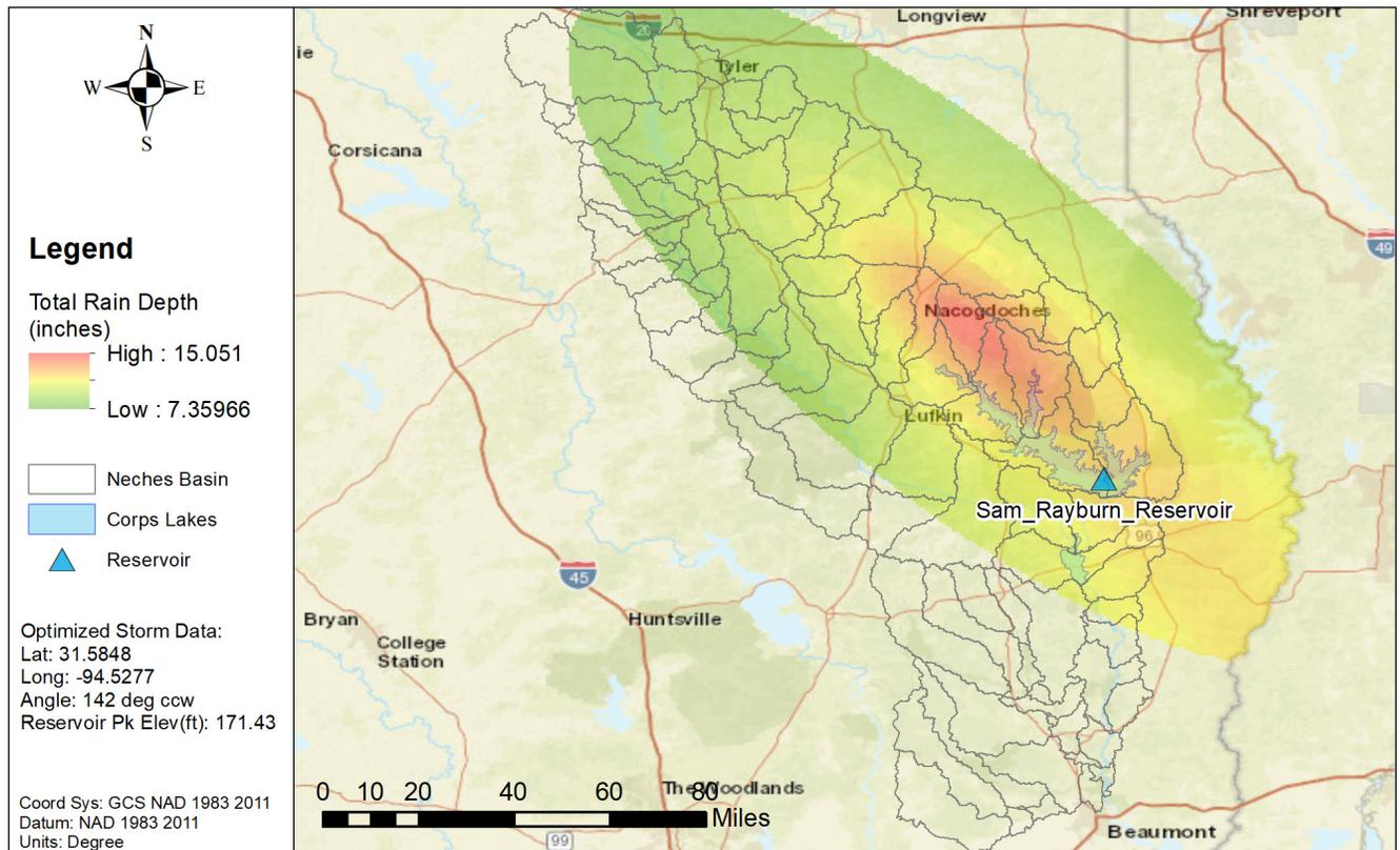
Figure 7.18b: NA14 1% AEP Elliptical Storm for Sam Rayburn Reservoir
