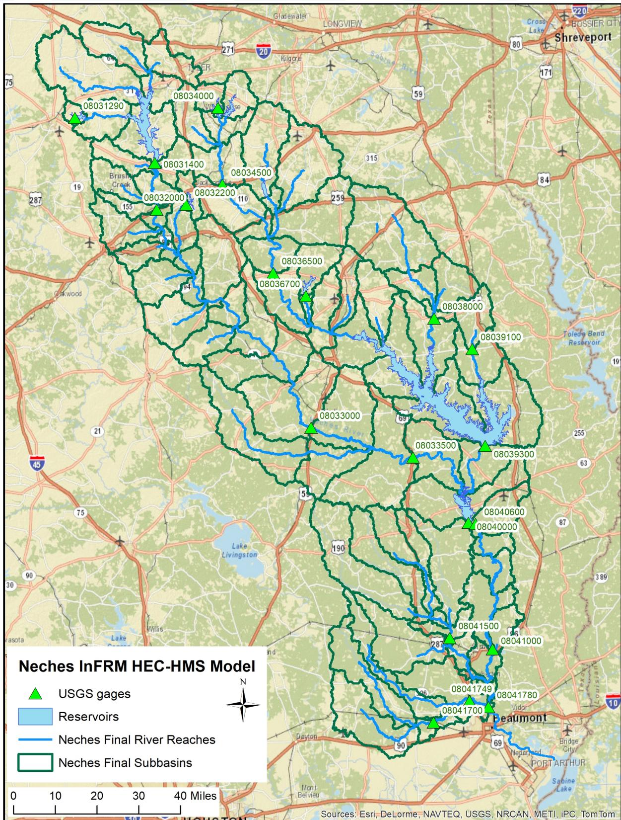
Figure 6.2: Final InFRM HEC-HMS Subbasins for the Neches River Basin
