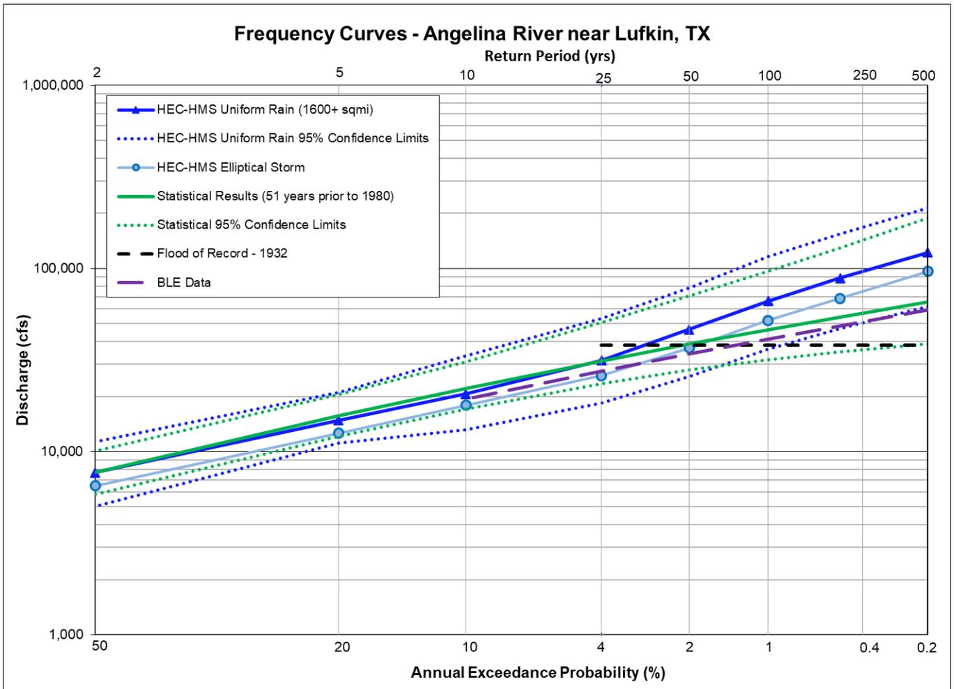
**Figure 11.7: Flow Frequency Curve Comparison for the Angelina River nr Lufkin, TX**
