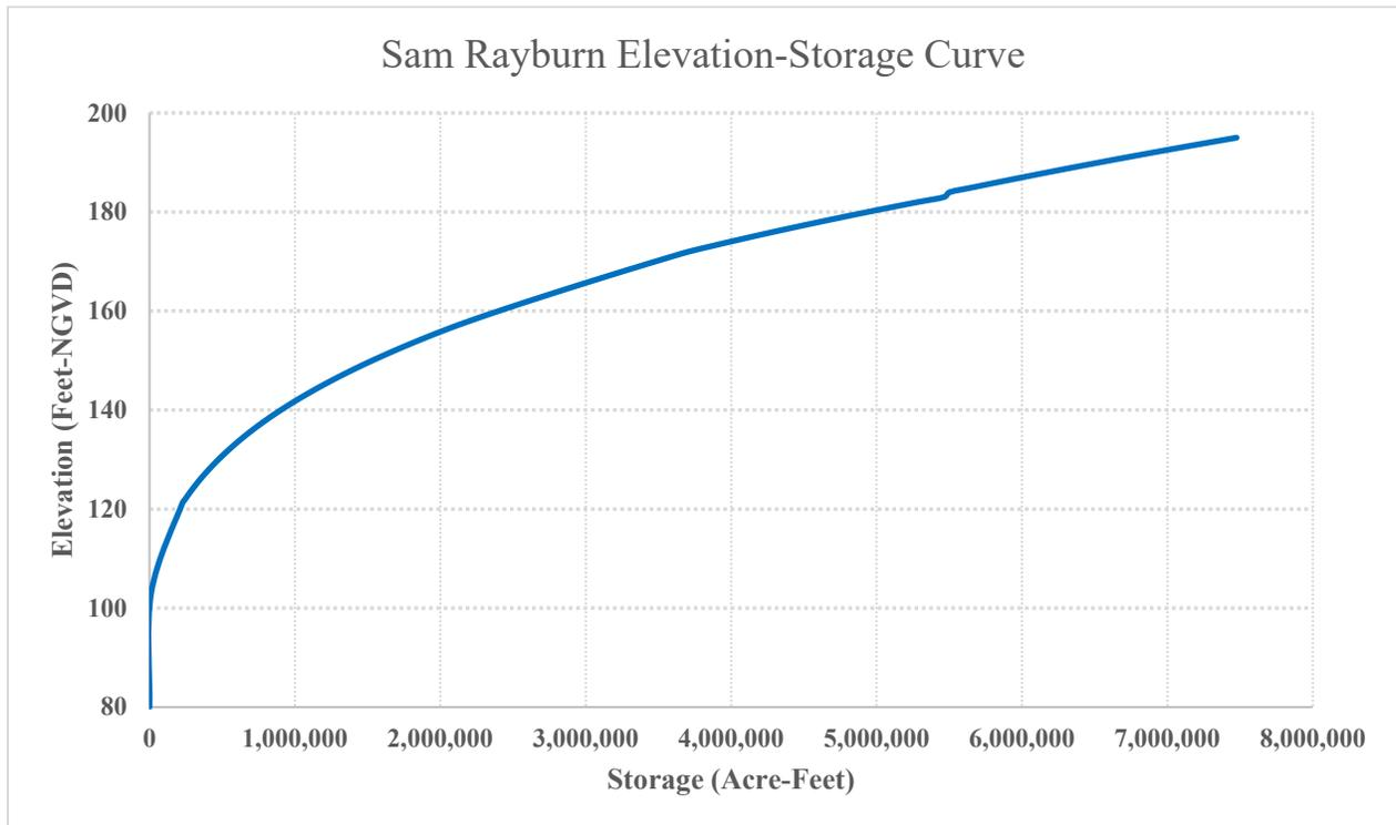
Figure 9.15: Sam Rayburn Storage-Elevation Curve
