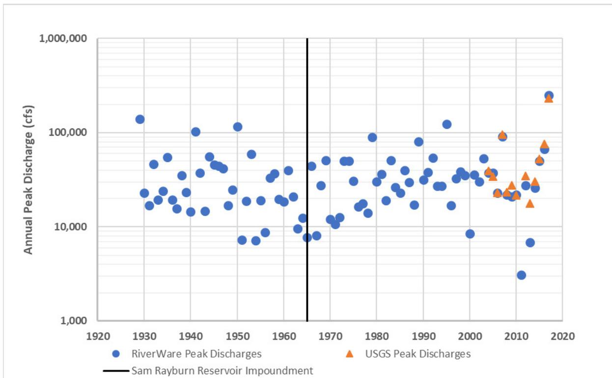
**Figure 8.21: RiverWare and USGS Annual Peak Discharges for Streamgaging Station 08041780 Neches River Saltwater Barrier at Beaumont, Tex.**
