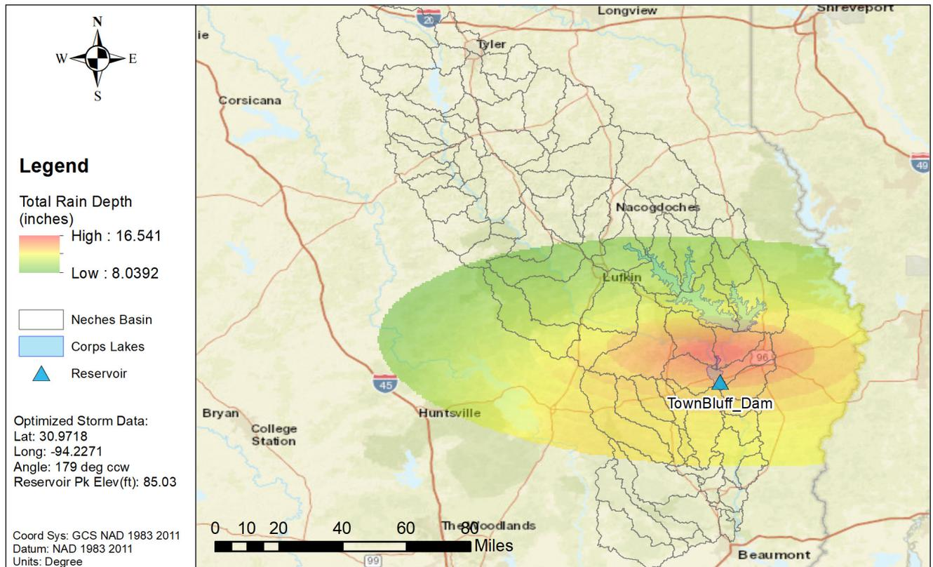
Figure 7.19b: NA14 1% AEP Elliptical Storm for B.A. Steinhagen Lake
