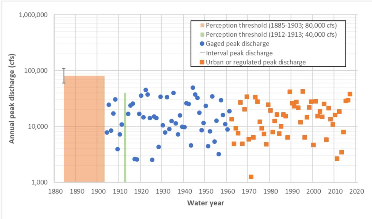
Figure 5.4: Annual Peak Discharge Data for USGS Station 08033500 Neches River nr Rockland, Tex.
