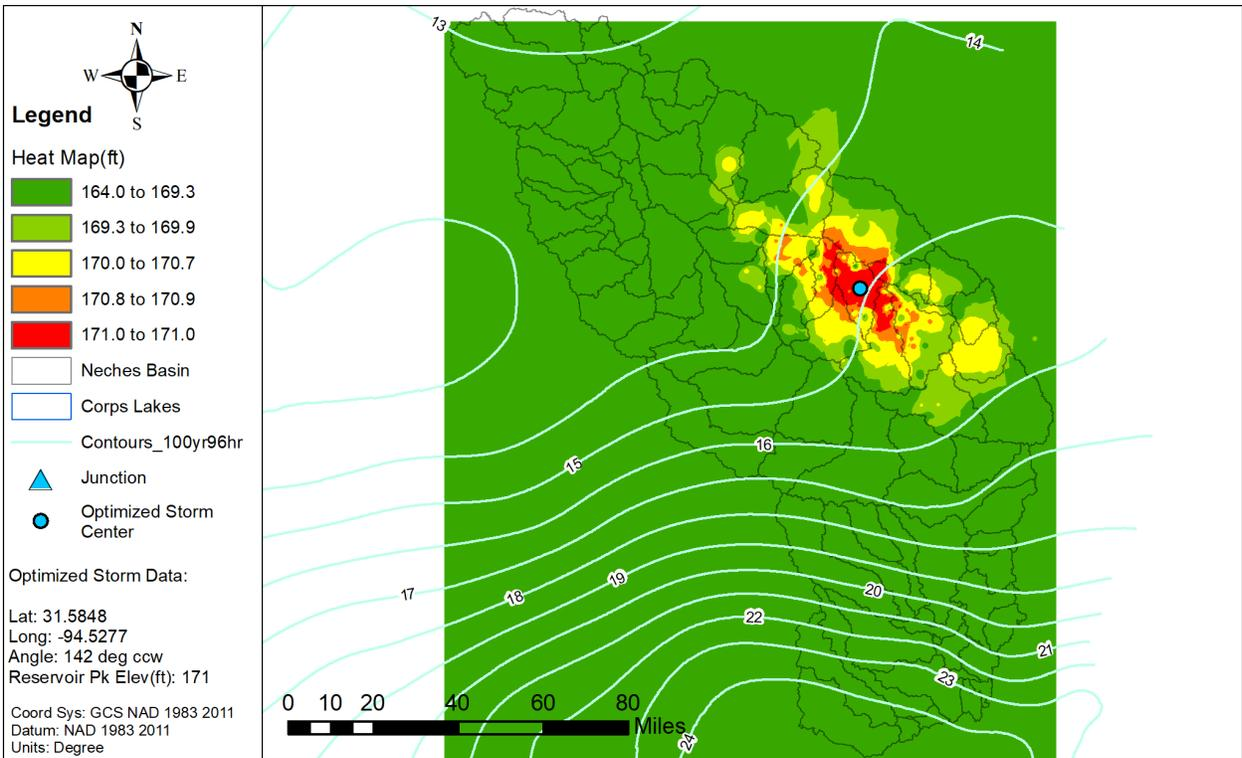
Figure 7.18a: Elliptical Storm Optimization Heat Map for Sam Rayburn Reservoir
