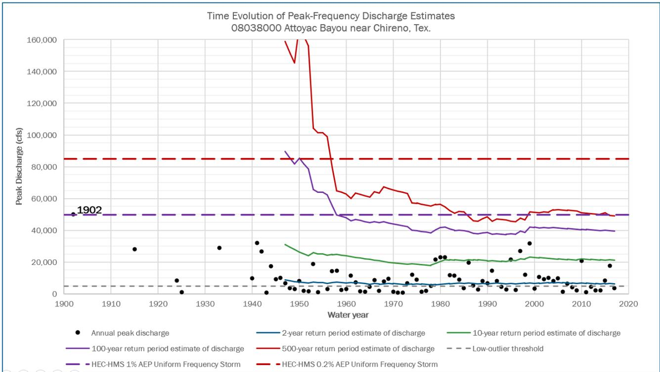
**Figure 11.8b: Statistical Change Over Time Comparison for Attoyac Bayou near Chireno, TX**
