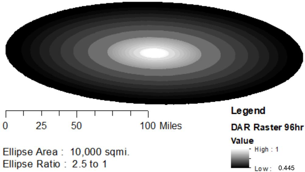
**Figure 7.6: Adopted Depth-Area-Reduction Rasterized Ellipse for the 96-hr Duration**
