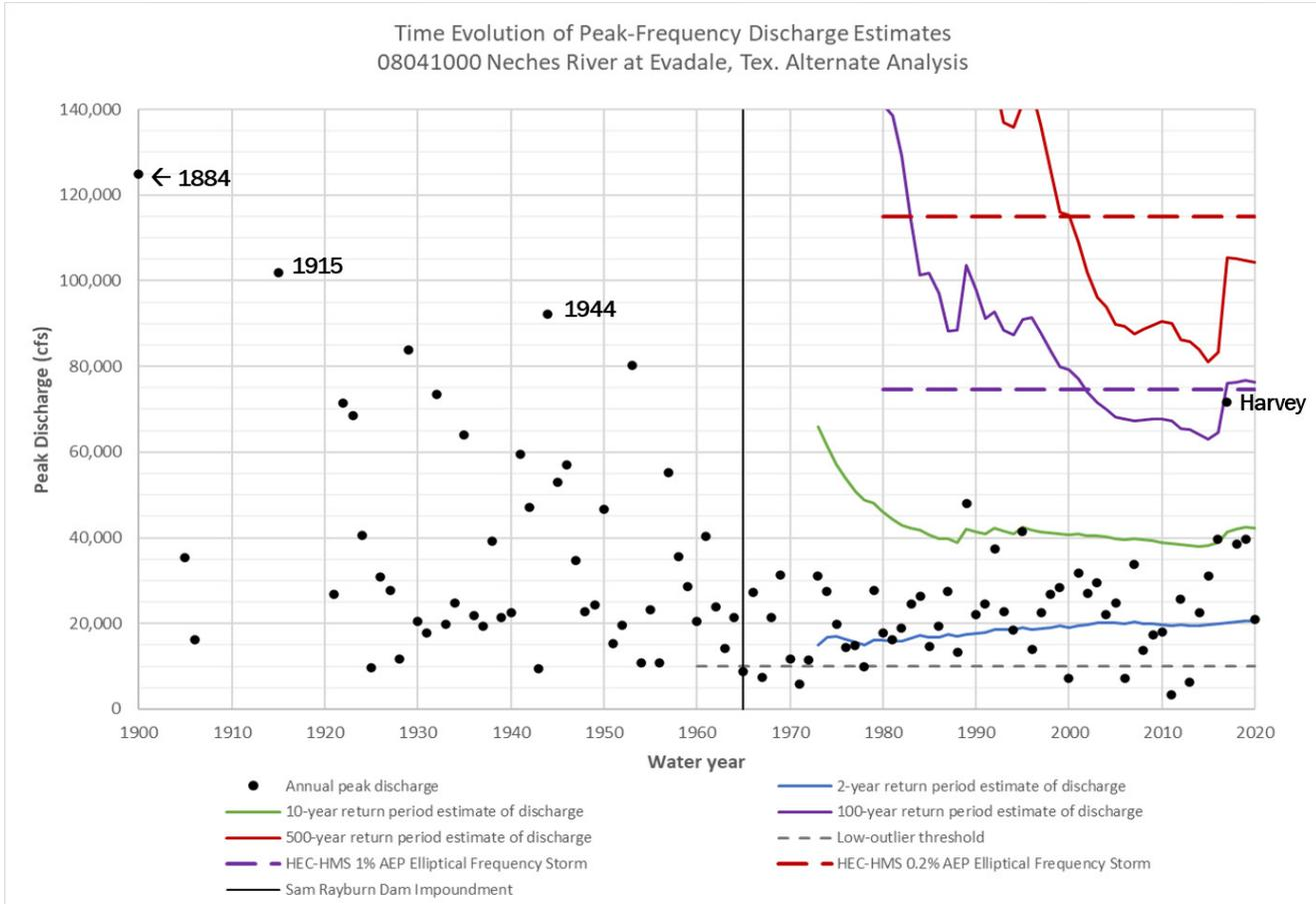
**Figure 11.12b: Statistical Change Over Time Comparison for the Neches River at Evadale, TX**
