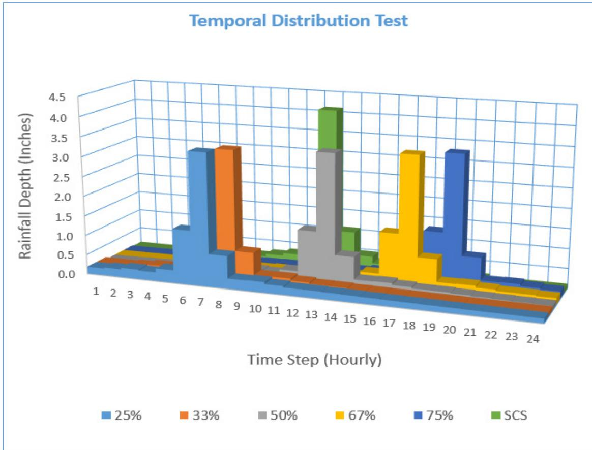
**Figure 7.7: Previously Tested Storm Temporal Distributions**
