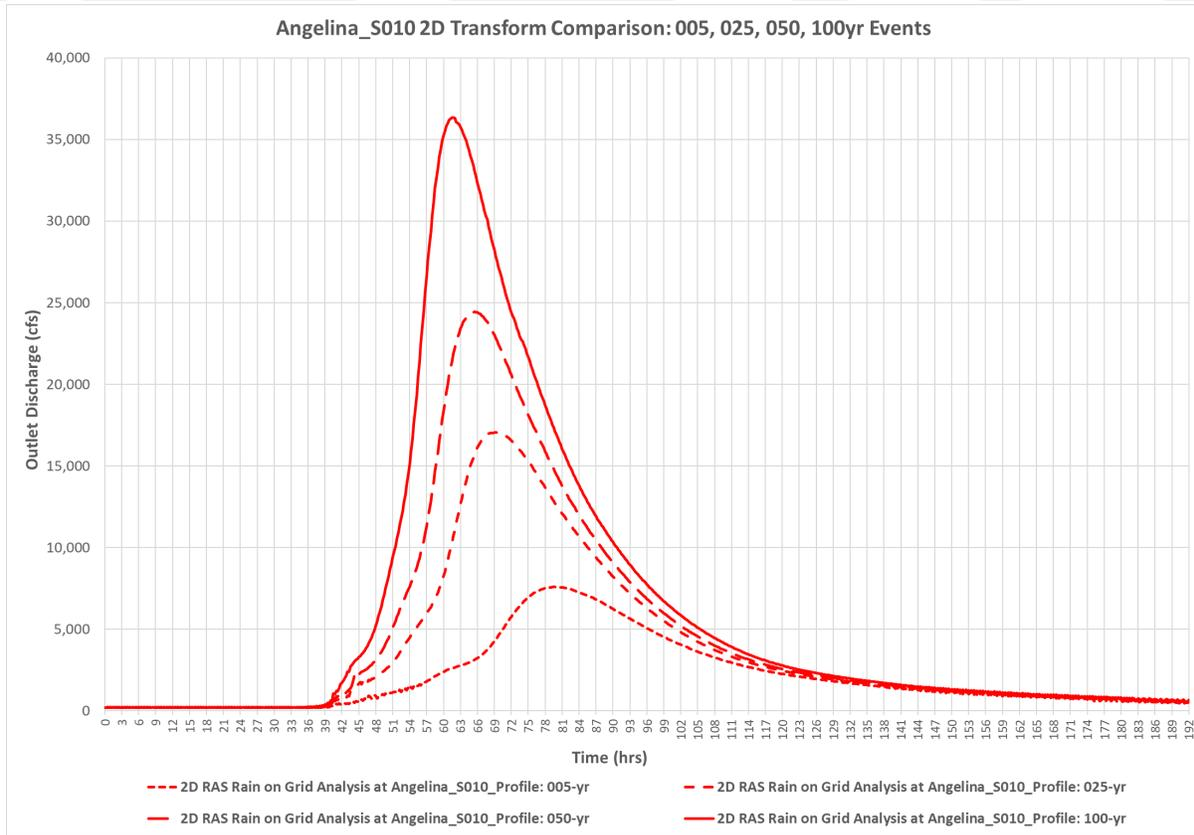
Figure 10.12: Example Subbasin 2D Frequency Results for Angelina\_S010
