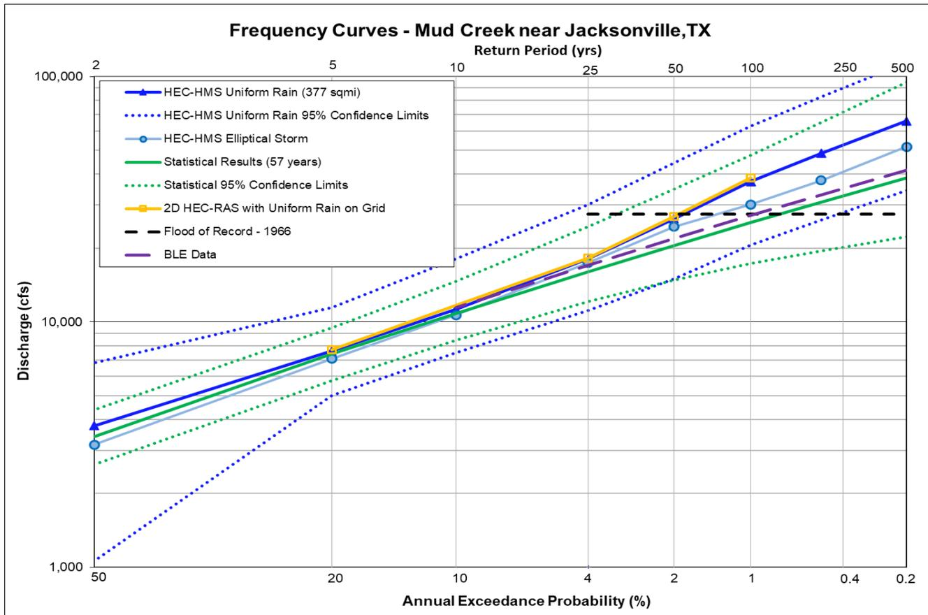
**Figure 11.5a: Flow Frequency Curve Comparison for Mud Creek near Jacksonville, TX**
