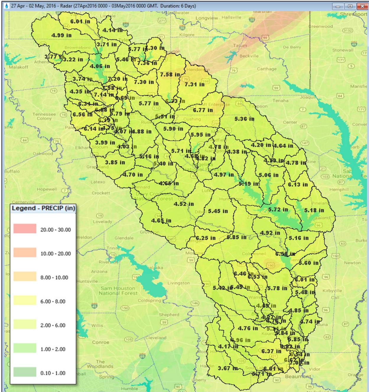
Figure 6.8: Total Rainfall Depths (inches) for the Apr-May 2016 Calibration Storm
