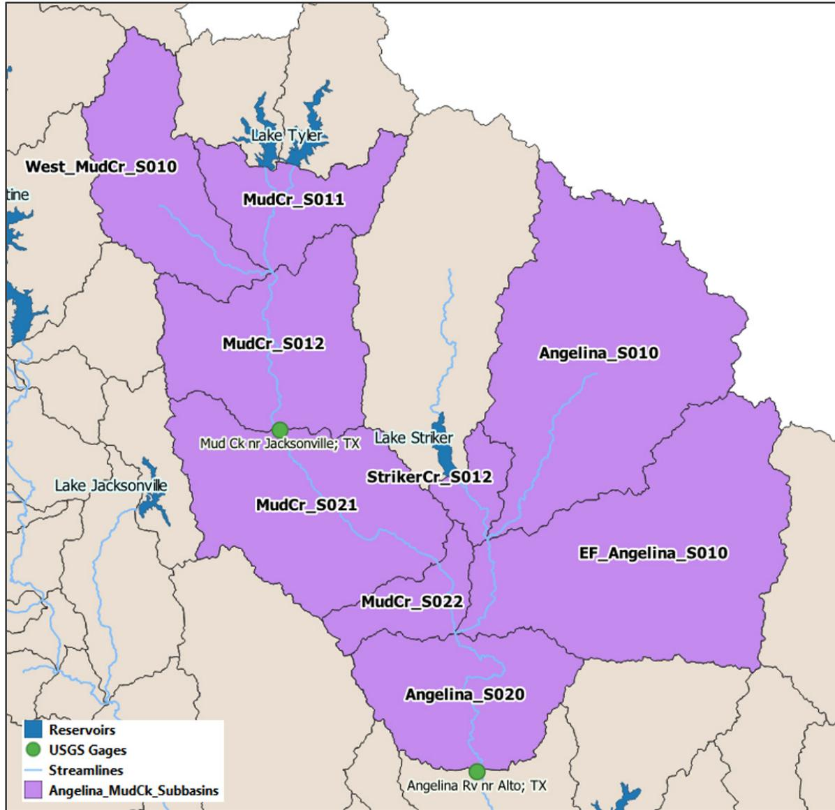
Figure 10.2: Neches InFRM HEC-HMS Model – Relevant Subbasins for the 2D Analysis
