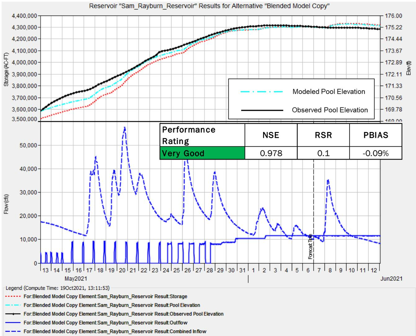
Figure 6.28: May 2021 Verification Results for Sam Rayburn Reservoir
