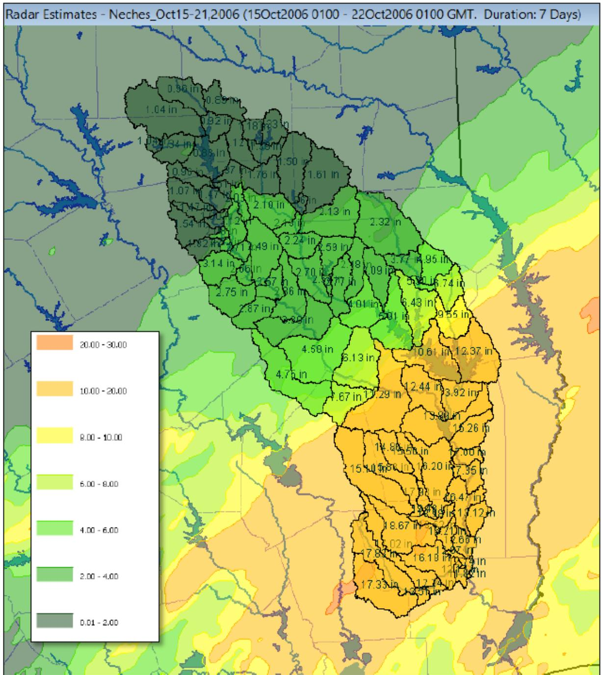
Figure 6.4: Total Rainfall Depths (inches) for the October 2006 Calibration Storm
