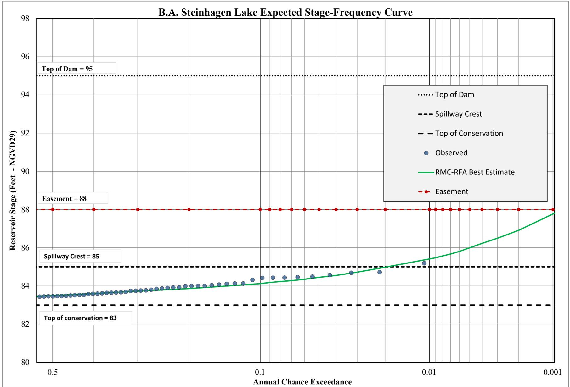
Figure 9.21: B.A. Steinhagen Lake RMC-RFA Final Stage-Frequency Curve
