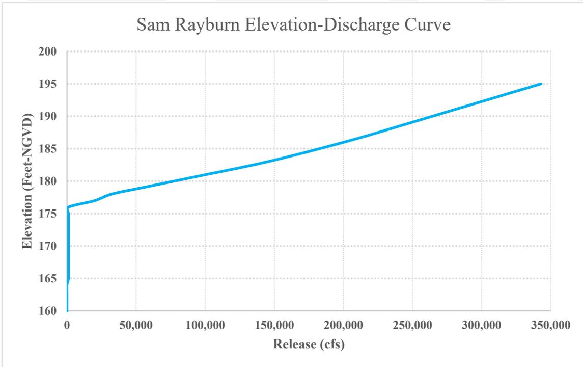
Figure 9.14: Sam Rayburn Outflow Elevation-Discharge Curve
