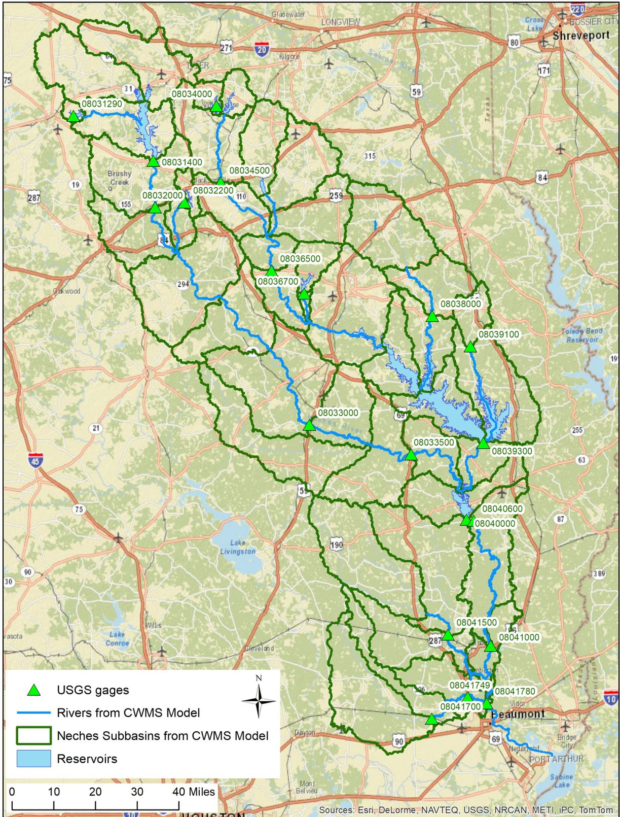
Figure 6.1: Existing CWMS Subbasins for the Neches River Basin
