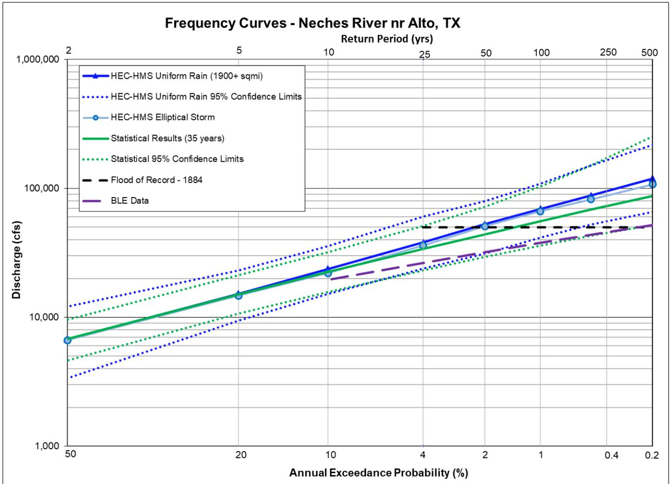
**Figure 11.2: Flow Frequency Curve Comparison for the Neches River nr Alto, TX (at the TX-21 Bridge)**
