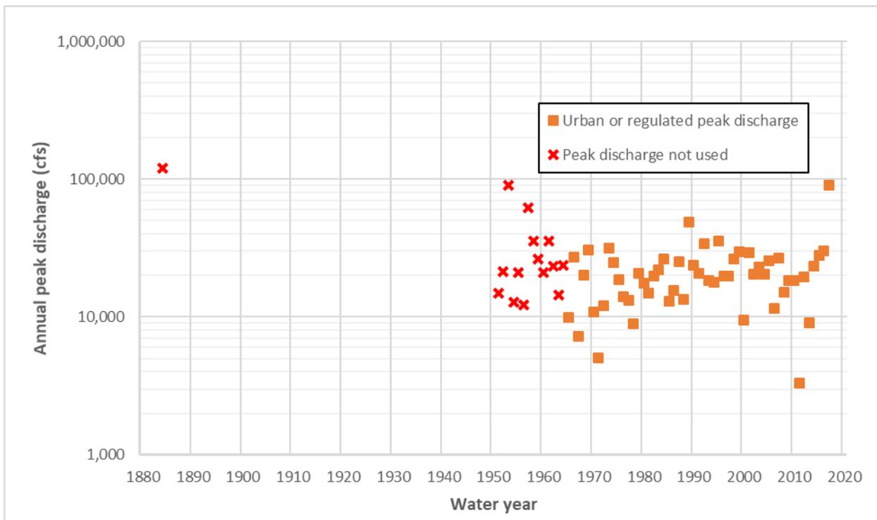
Figure 5.8: Annual Peak Discharge Data for USGS Station 08040600 Neches River near Town Bluff, Tex.
