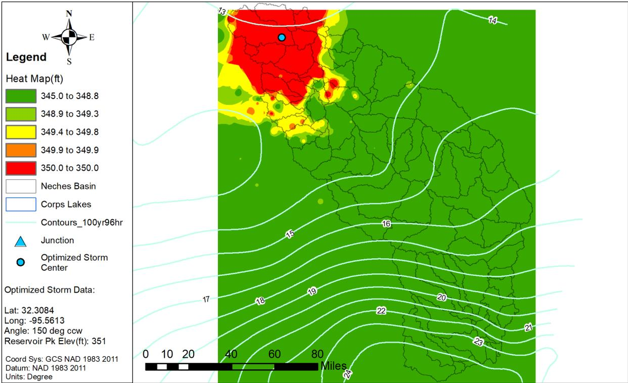
Figure 7.17a: Elliptical Storm Optimization Heat Map for Lake Palestine
