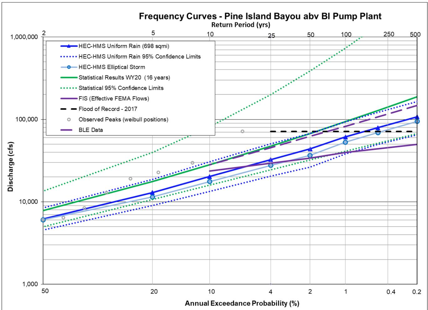
**Figure 11.15: Flow Frequency Curve Comparison for Pine Island Bayou above BI Pump Plant**
