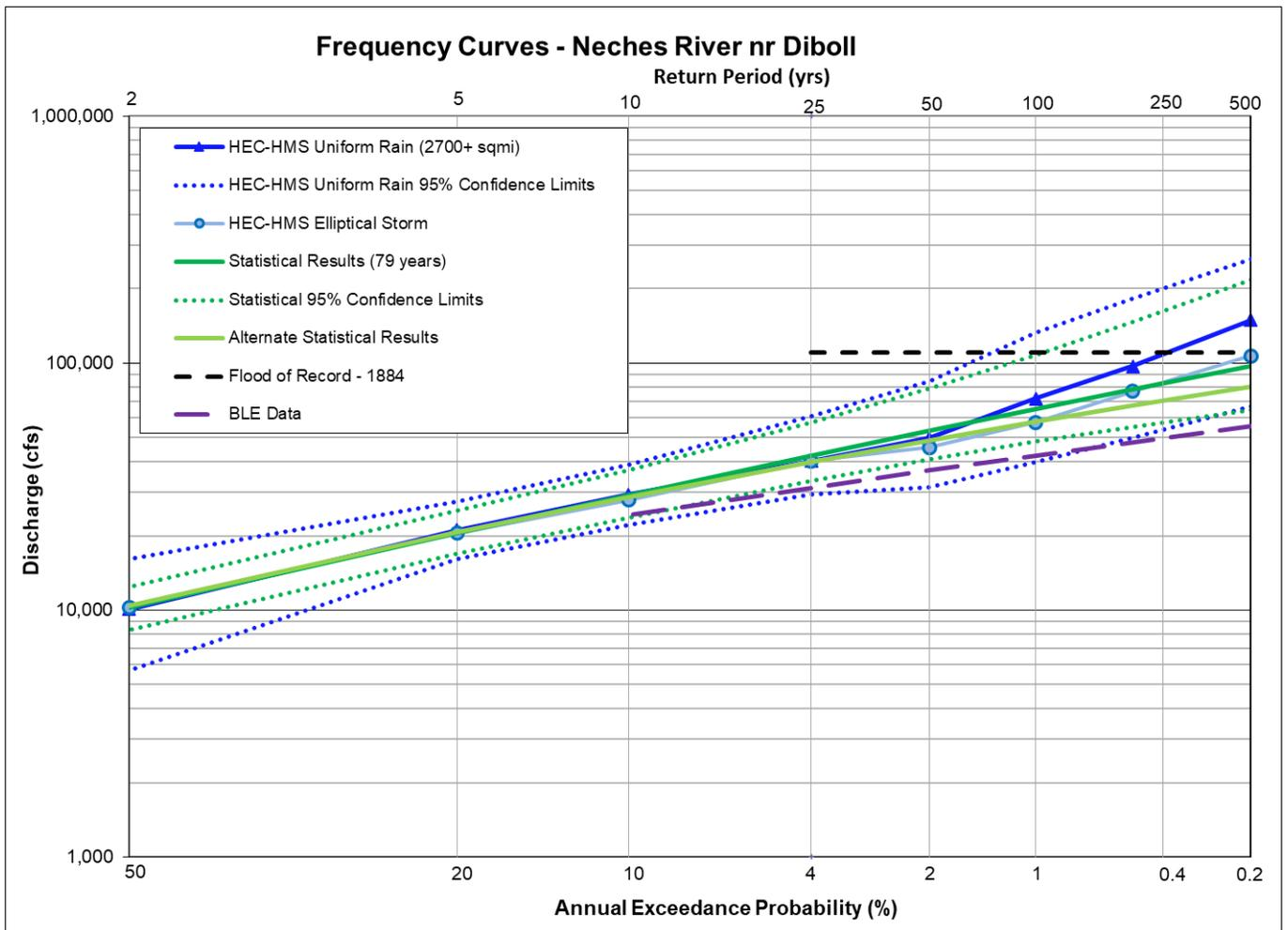
**Figure 11.3a: Flow Frequency Curve Comparison for the Neches River nr Diboll, TX**
