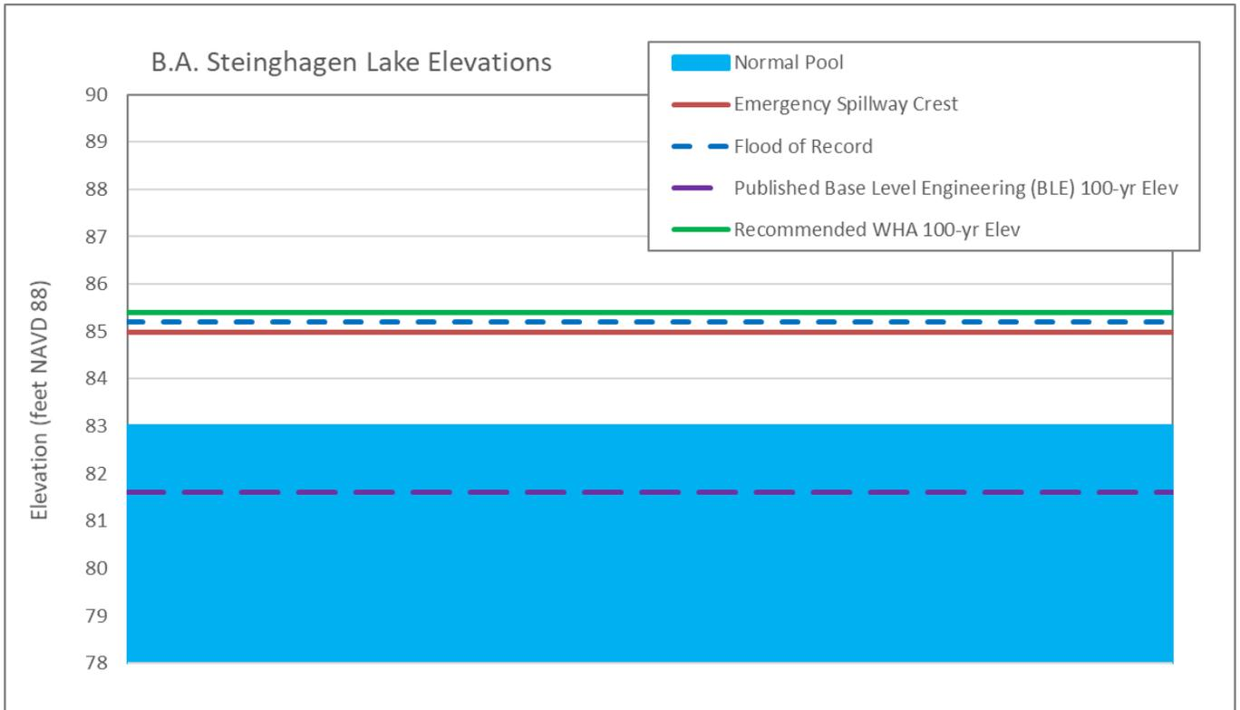
Figure ES.5: Comparison of 100-yr Pool Elevations for B.A. Steinghagen Lake
