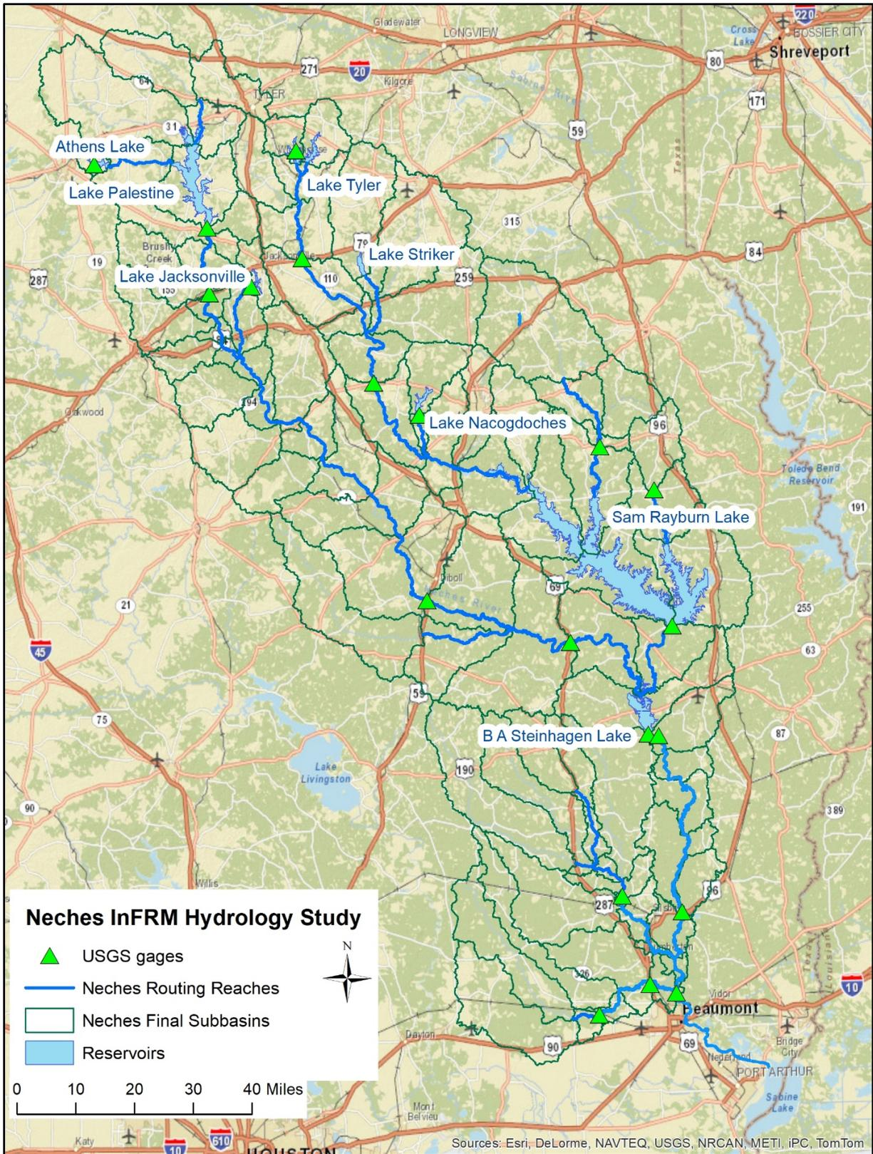
Figure 6.3: Locations of Reservoirs Modeled in HEC-HMS
