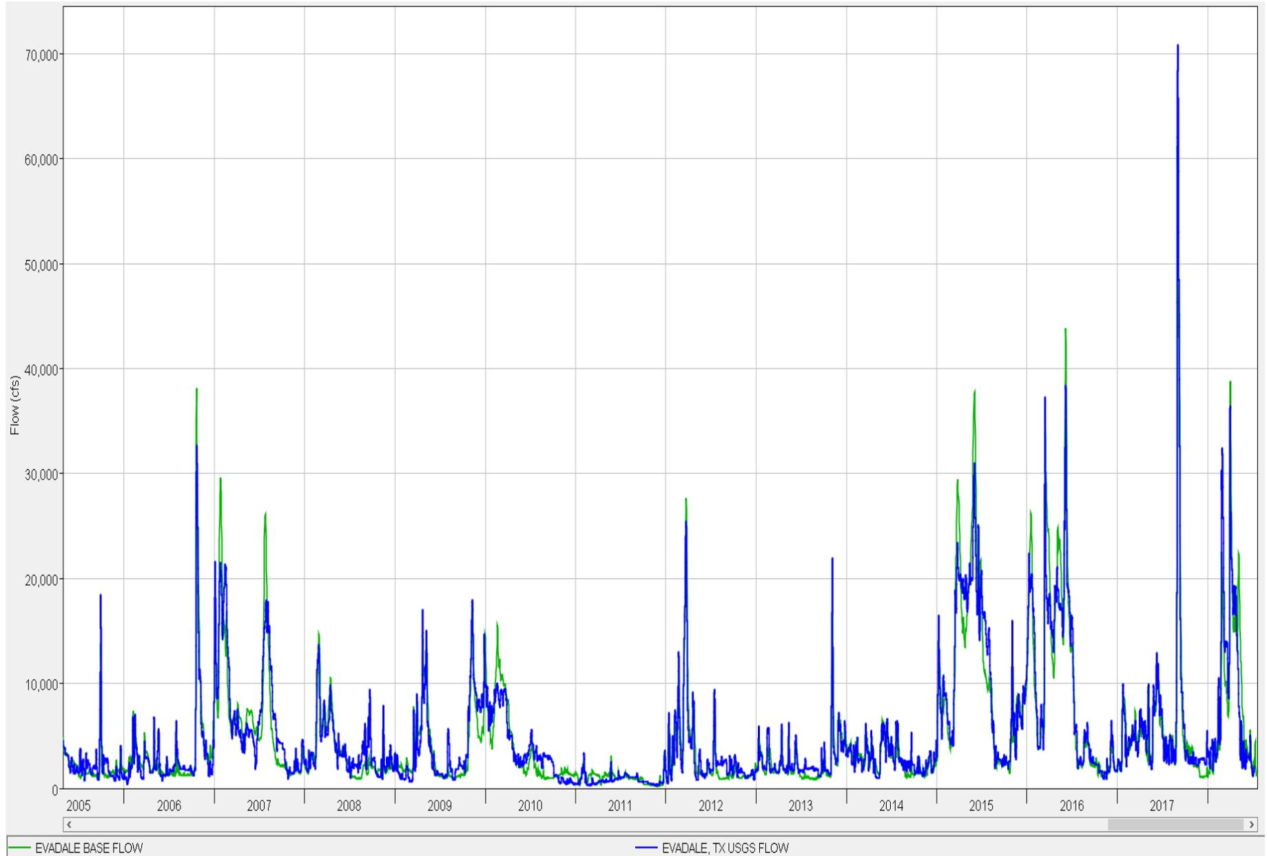
Figure 8.6: RiverWare Model Results Comparison for USGS Streamgauge Station 08041000 Neches River at Evadale, Tex.
