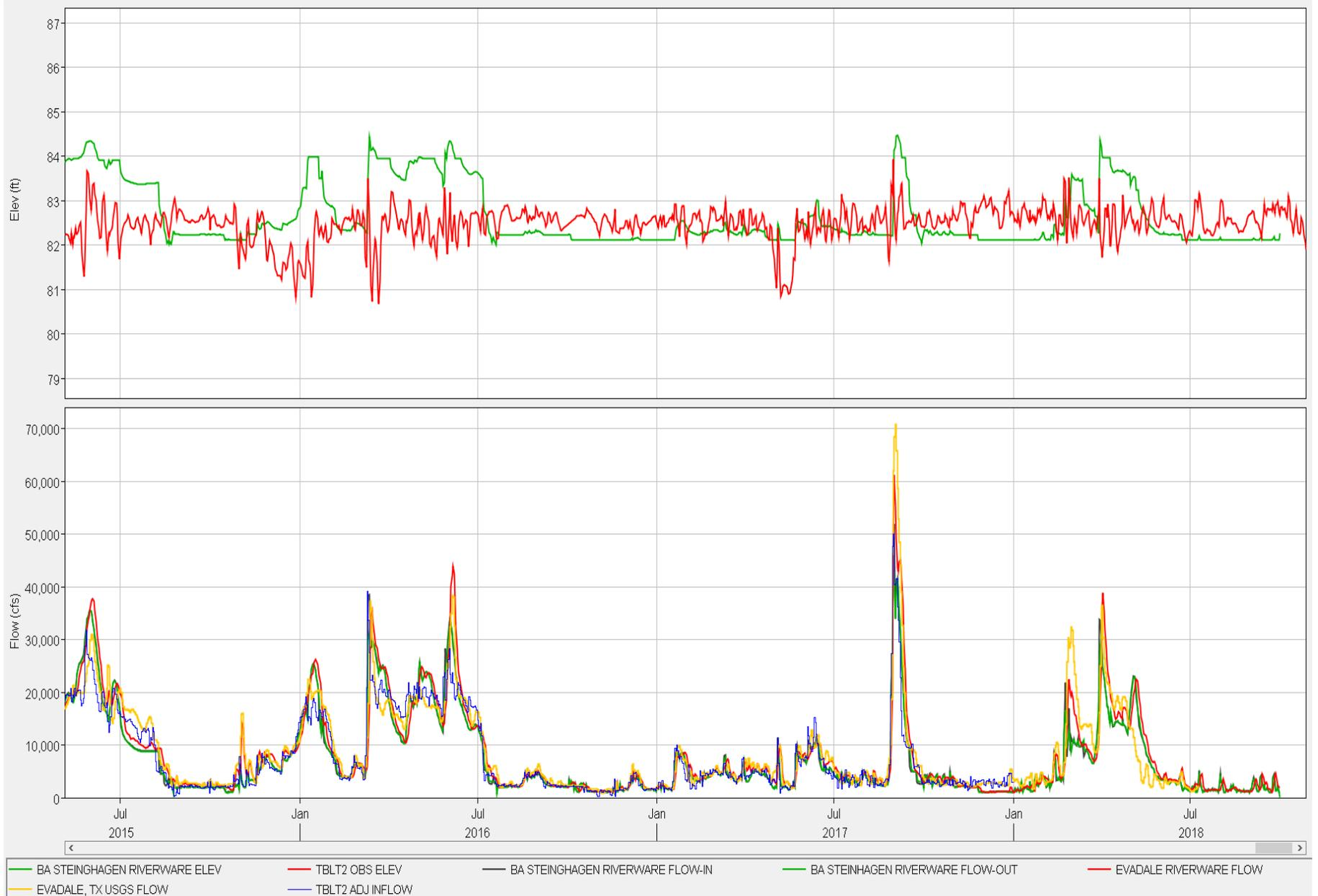
Figure 8.5: Model Simulation Results for Water Years 2015 Through 2018
