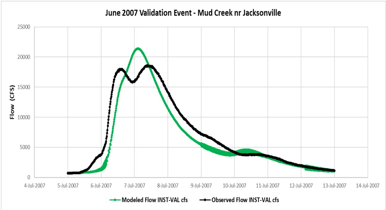
Figure 10.9: June 2007 Modeled vs Observed Flow – Mud Creek nr Jacksonville
