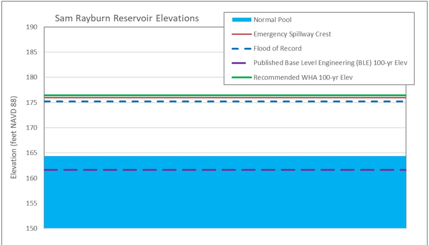
Figure ES.4: Comparison of 100-yr Pool Elevations for Sam Rayburn Reservoir
