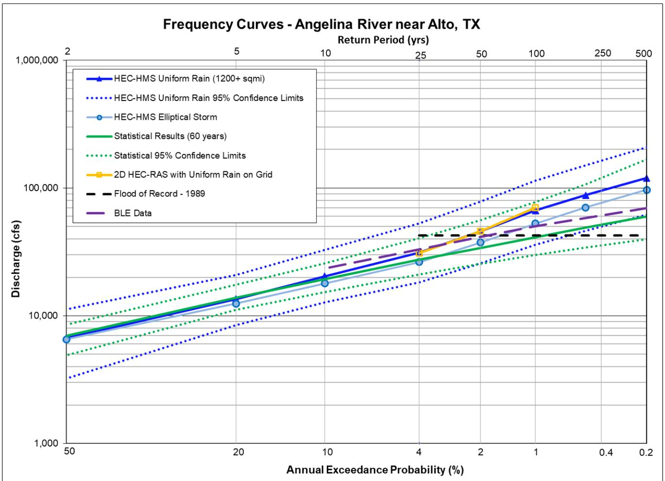
**Figure 11.6a: Flow Frequency Curve Comparison for the Angelina River nr Alto, TX**
