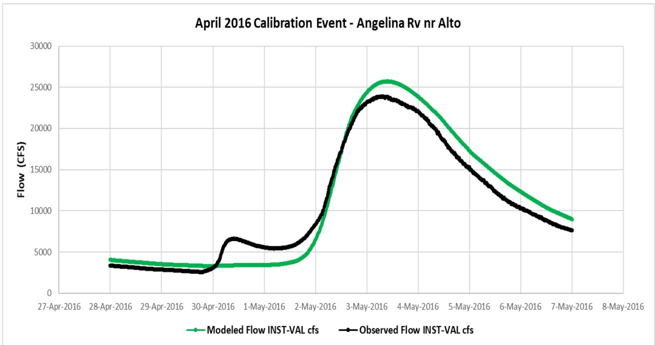
Figure 10.8: April 2016 Modeled vs Observed Flows – Angelina Rv nr Alto
