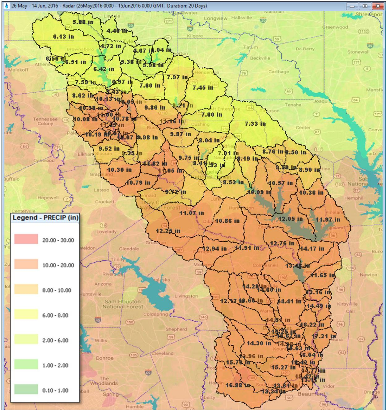
Figure 6.9: Total Rainfall Depths (inches) for the May-Jun 2016 Calibration Storm
