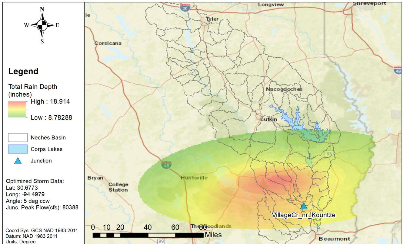
Figure 7.15b: NA14 1% AEP Elliptical Storm for VillageCr\_nr\_Kountze
