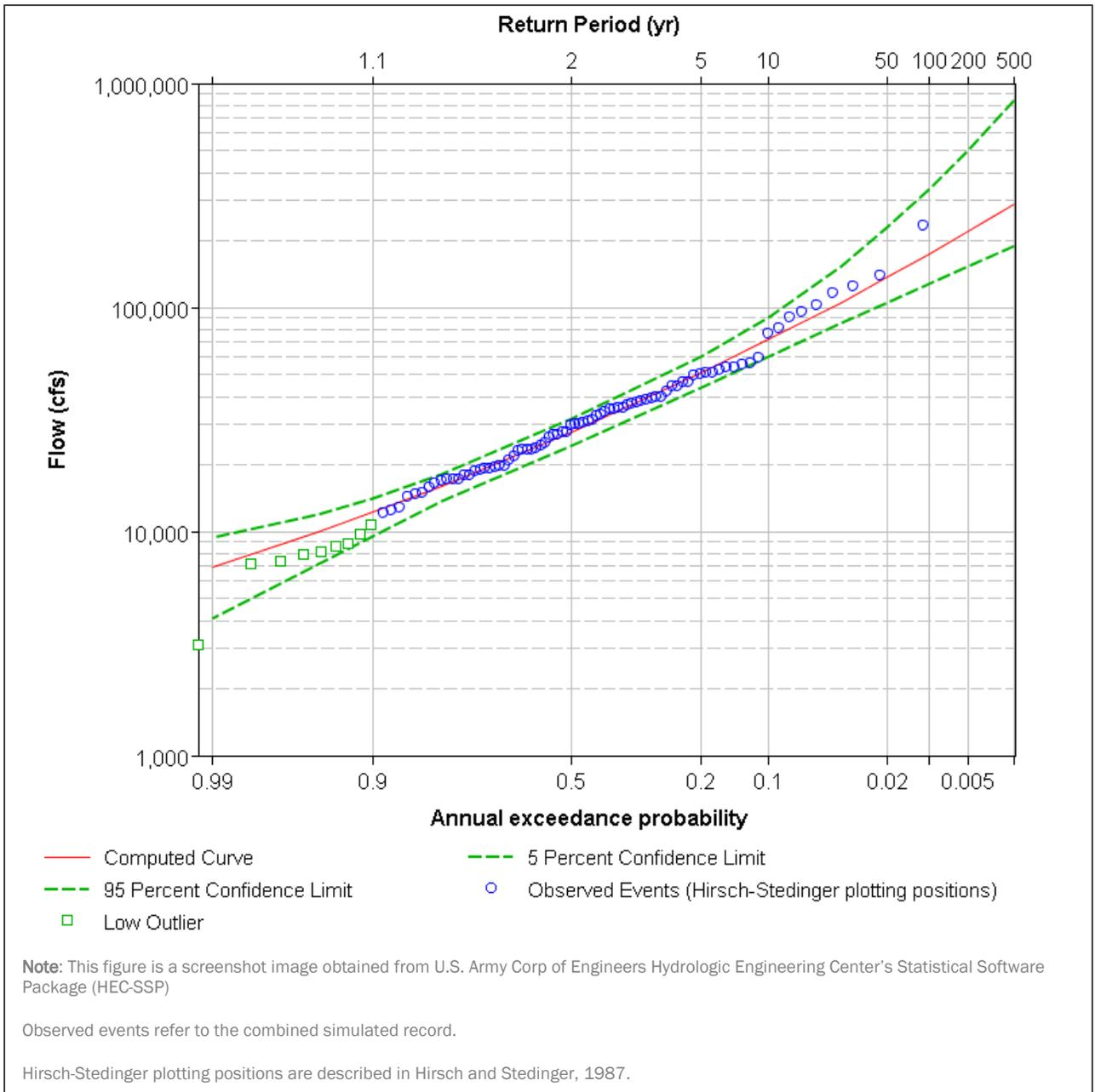
**Figure 8.22: Simulated Flood Flow Frequency Determined by using a log-Pearson Type III Distribution for USGS Streamgaging Station 08041780 Neches River Saltwater Barrier at Beaumont, Tex.**
