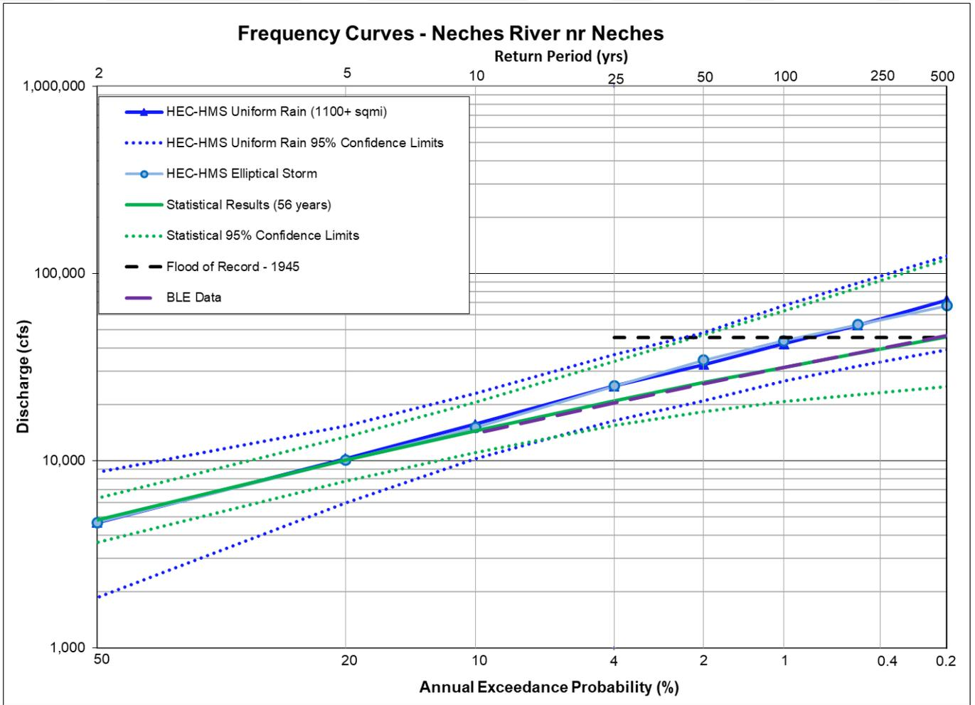
Figure 11.1a: Flow Frequency Curve Comparison for the Neches River nr Neches, TX
