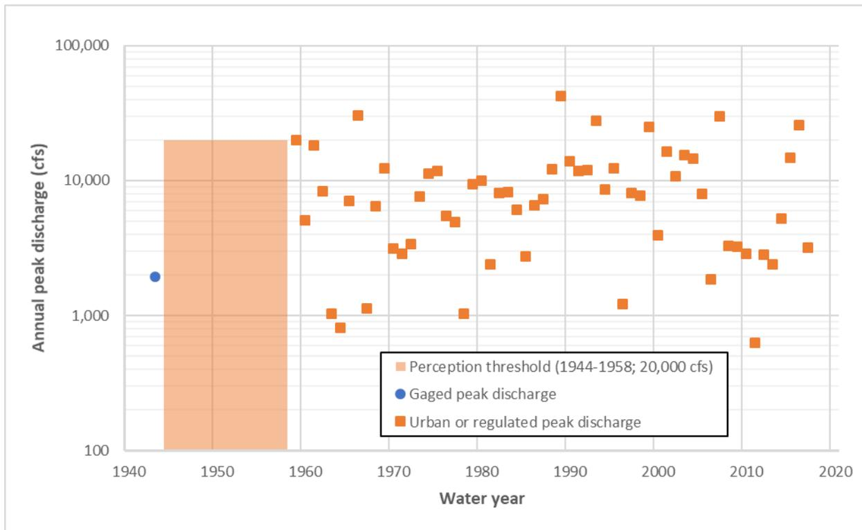
Figure 5.6: Annual Peak Discharge Data for USGS Station 08036500 Angelina River near Alto, Tex.
