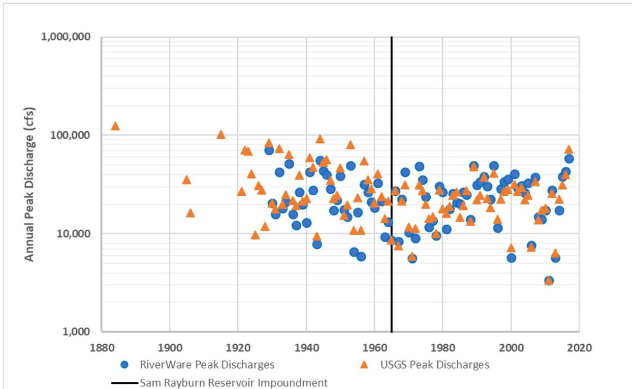
Figure 8.18: Simulated RiverWare and Observed USGS Annual Peak Discharges for USGS Streamgaging Station 08041000 Neches River at Evadale, Tex.
