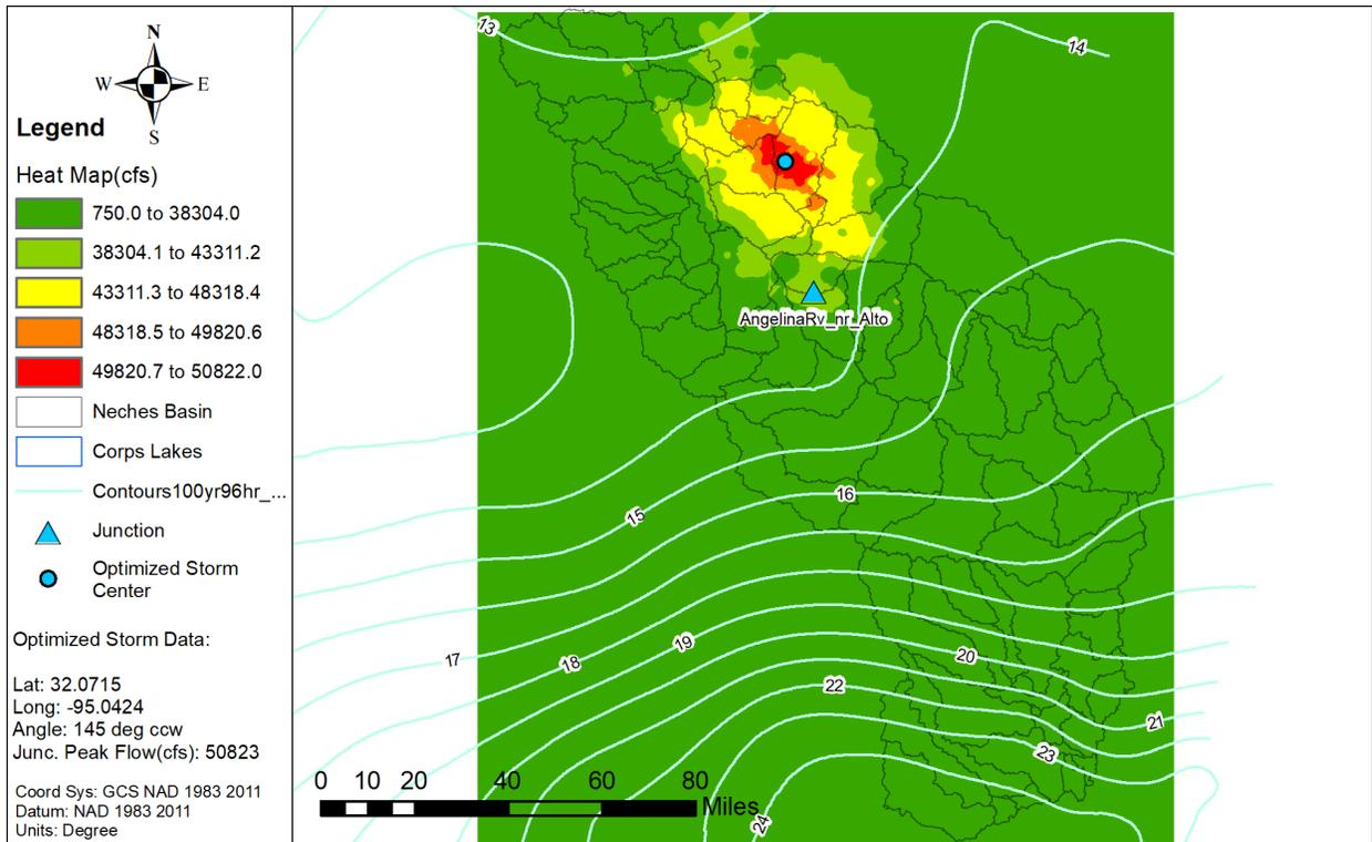
Figure 7.12a: Elliptical Storm Optimization Heat Map for AngelinaRv\_nr\_Alto
