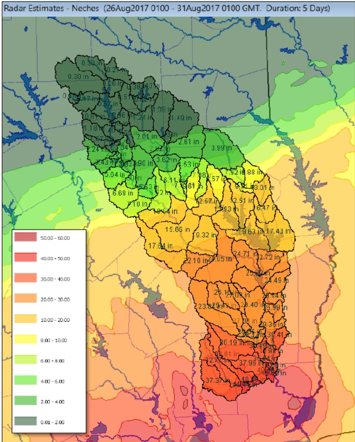
Figure 6.10: Total Rainfall Depths (inches) for Hurricane Harvey, Aug-Sep 2017, Calibration Storm
