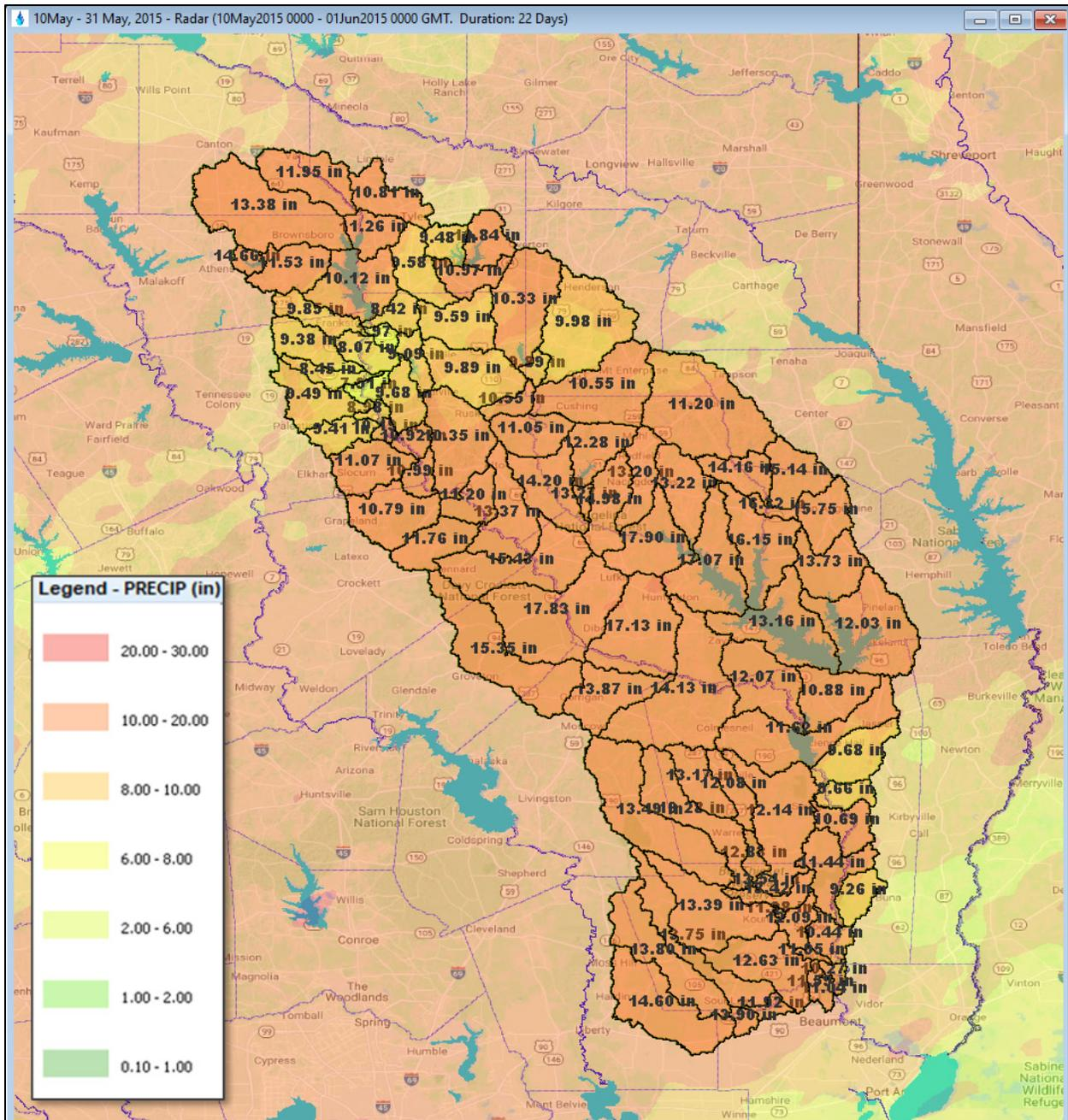
Figure 6.6: Total Rainfall Depths (inches) for the May-Jun 2015 Calibration Storm
