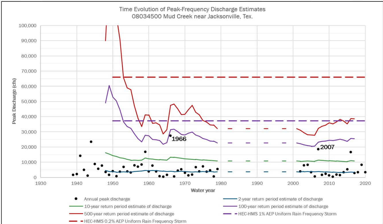
**Figure 11.5b: Statistical Change Over Time Comparison for the Mud Creek near Jacksonville, TX**
