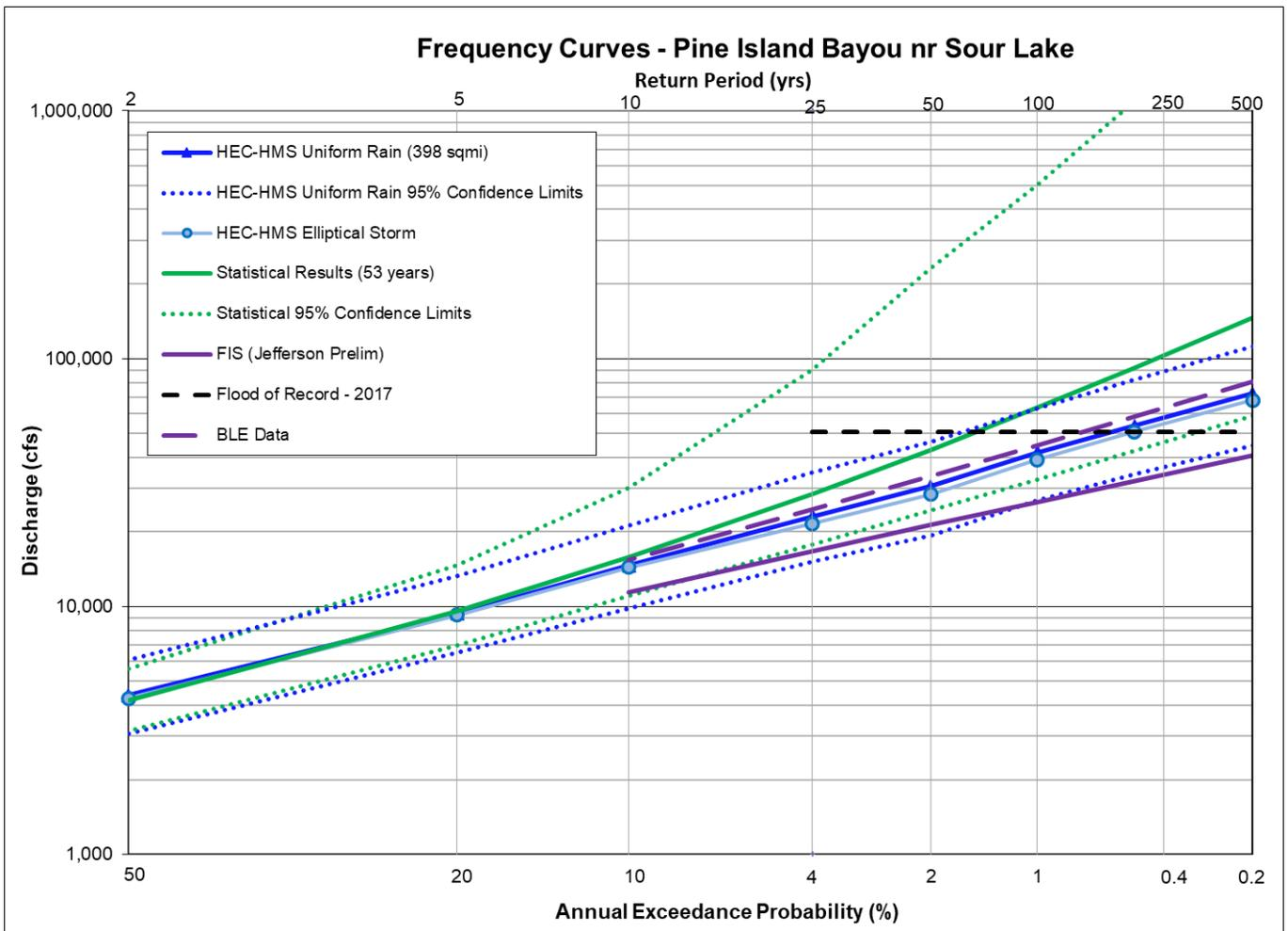
**Figure 11.14a: Flow Frequency Curve Comparison for Pine Island Bayou near Sour Lake, TX**
