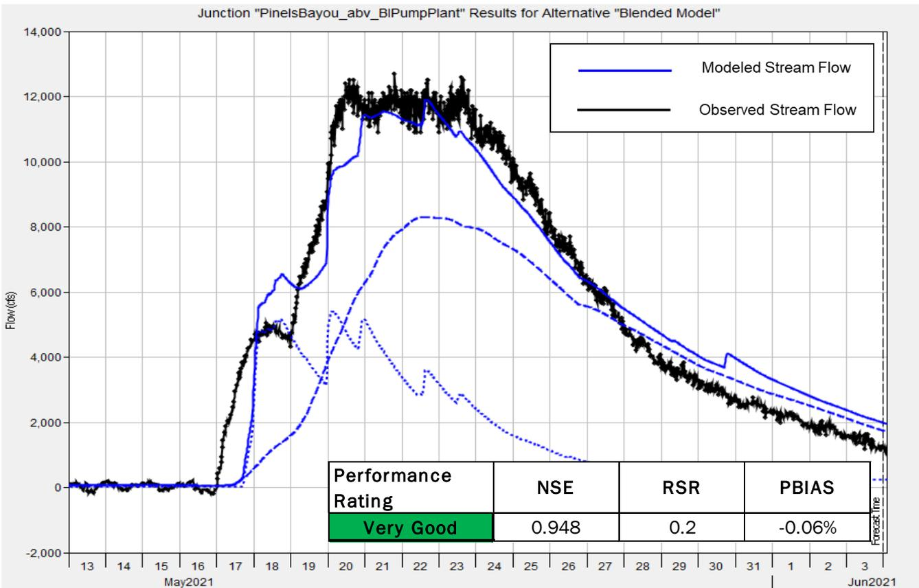
Figure 6.30: May 2021 Verification Results for Pine Island Bayou above BI Pump Plant
