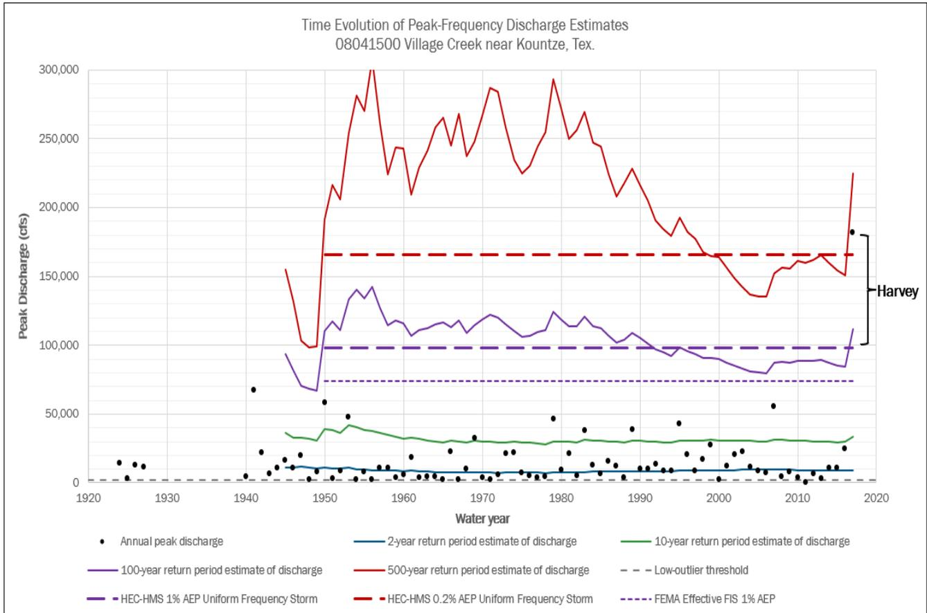
**Figure 11.13b: Statistical Change Over Time Comparison for Village Creek near Kountze, TX**
