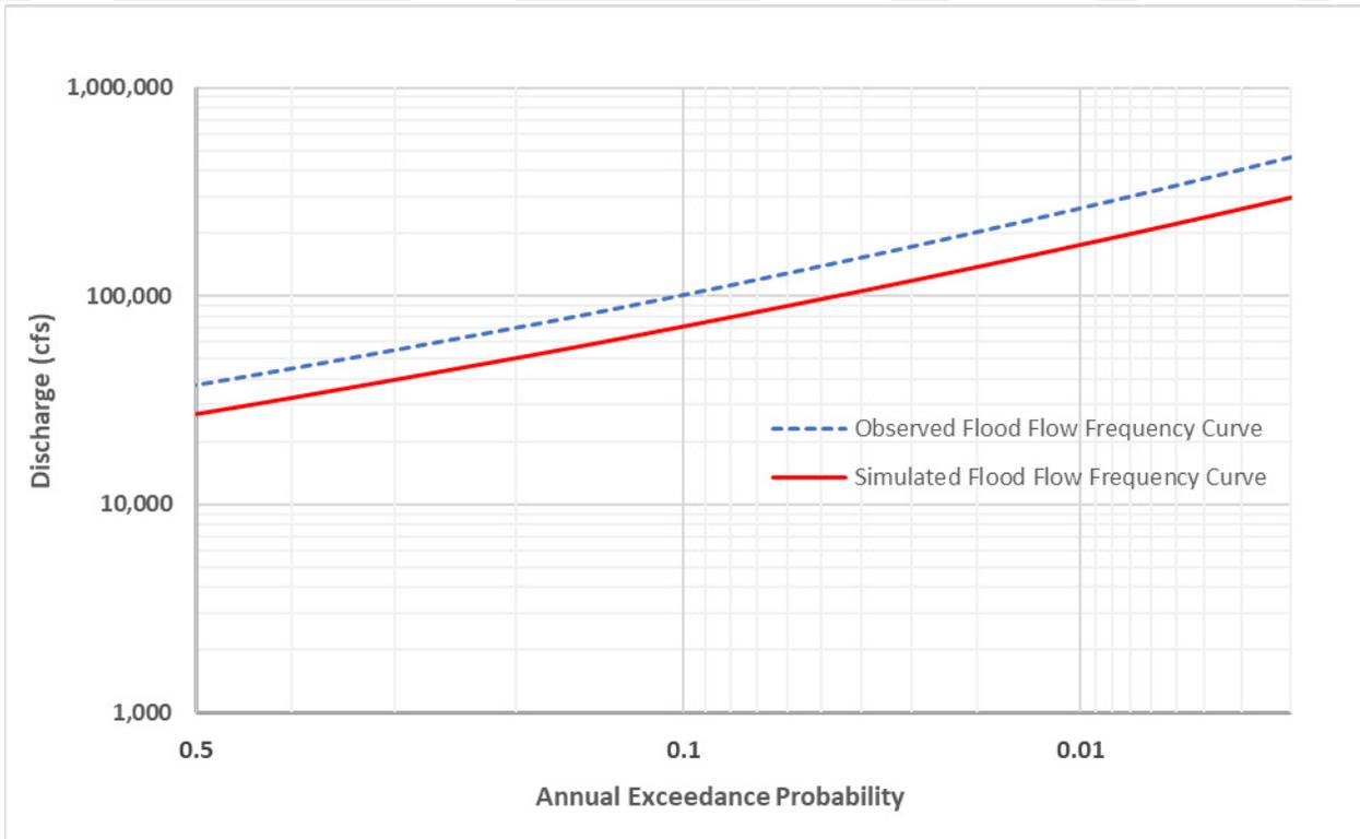
Figure 8.23: Comparison of Flood Flow Frequency Curves for the Observed and Simulated Datasets for USGS Streamgaging Station 08041780 Neches River Saltwater Barrier at Beaumont, Tex.
