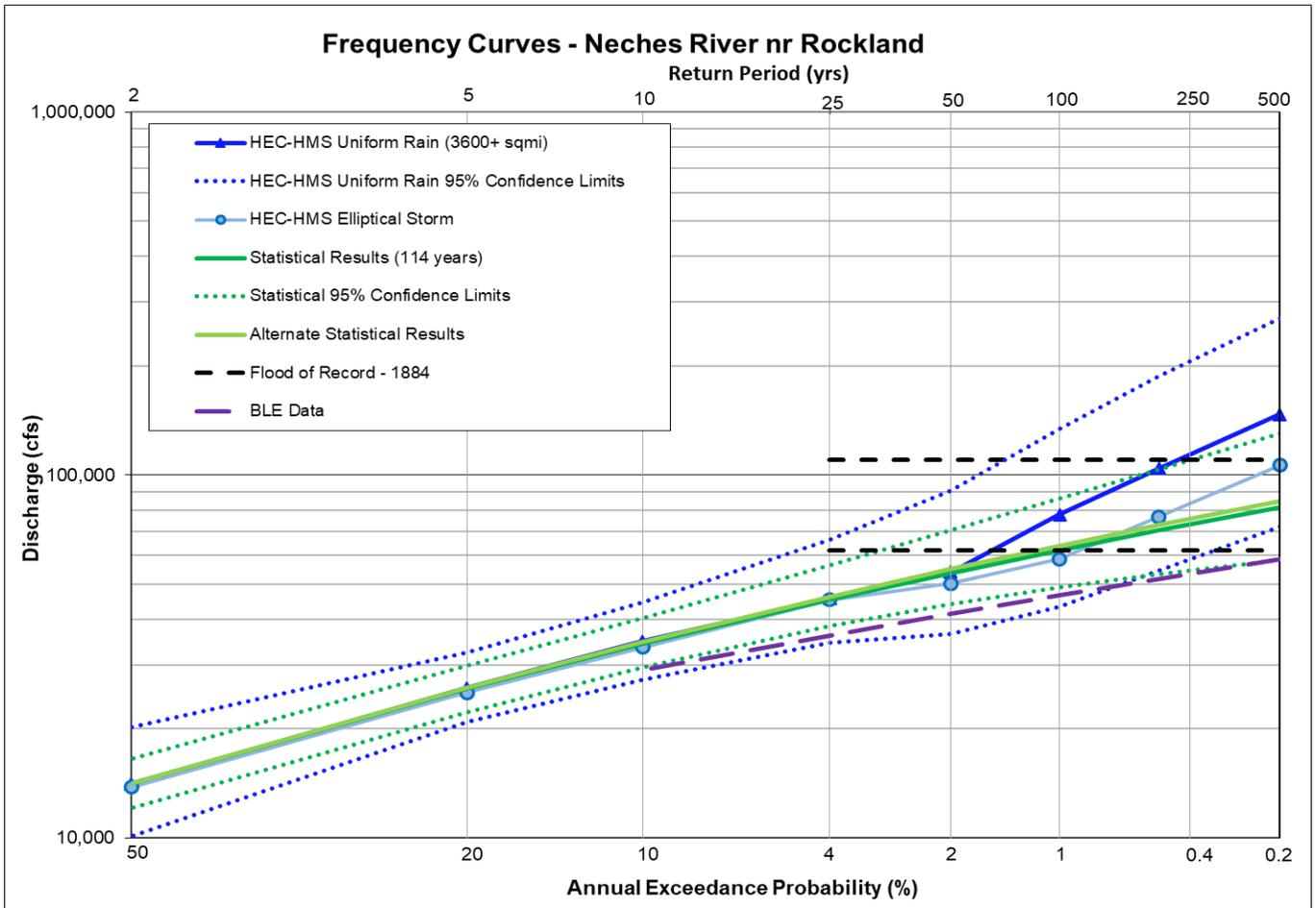
**Figure 11.4a: Flow Frequency Curve Comparison for the Neches River nr Rockland, TX**
