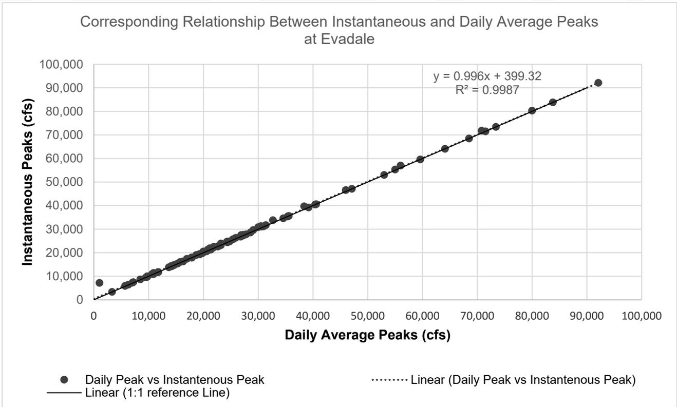
Figure 8.12: Instantaneous vs. Daily Average Peak Discharges for USGS Streamgaging Station 08041000 Neches River at Evadale, Tex.
