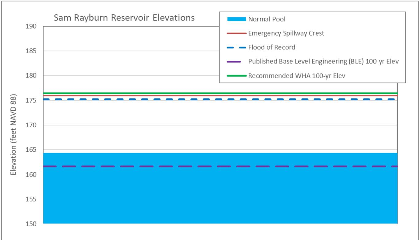
Figure 13.3: Comparison of Pool Elevations for Sam Rayburn Reservoir
