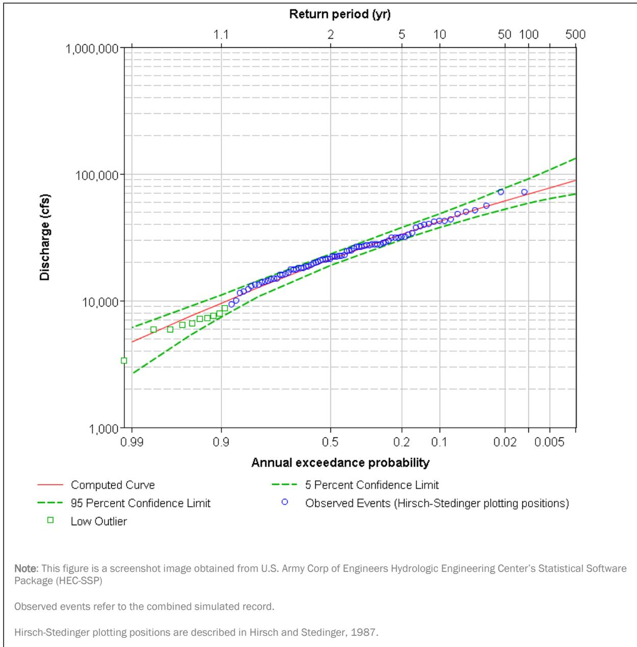
**Figure 8.19: Simulated Flood Flow Frequency using log-Pearson Type III Distribution for USGS Streamgaging Station 08041000 Neches River at Evadale, Tex.**
