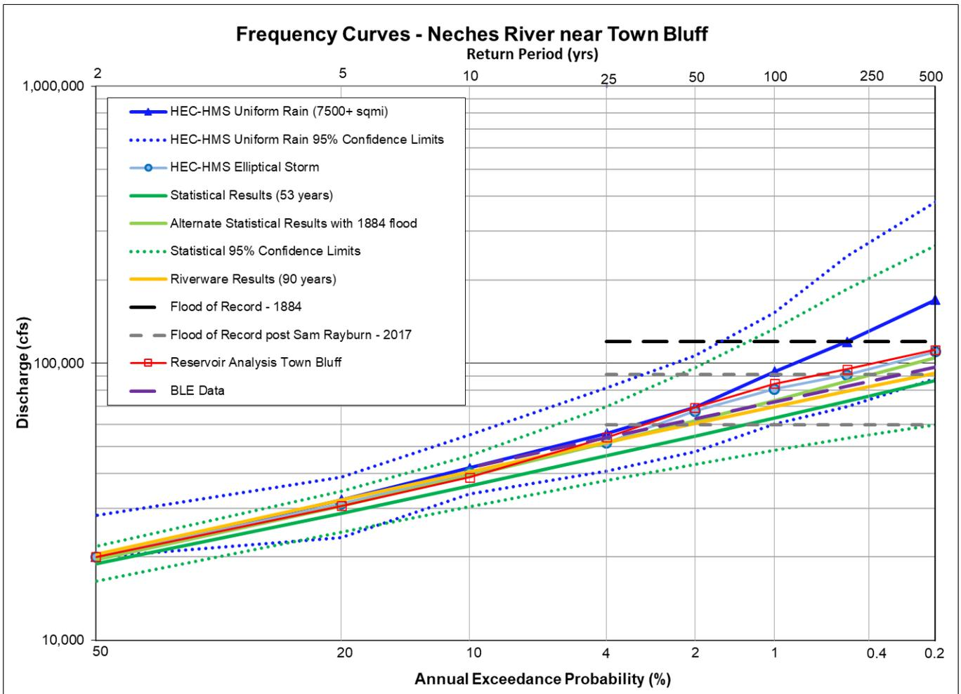
Figure 11.11a: Flow Frequency Curve Comparison for the Neches River nr Town Bluff, TX
