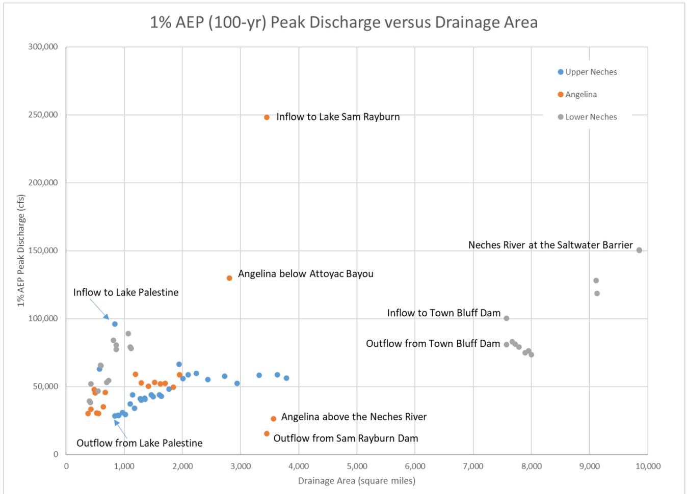
Figure 7.20: NA14 1% AEP Elliptical Storm Frequency Results versus Drainage Area
