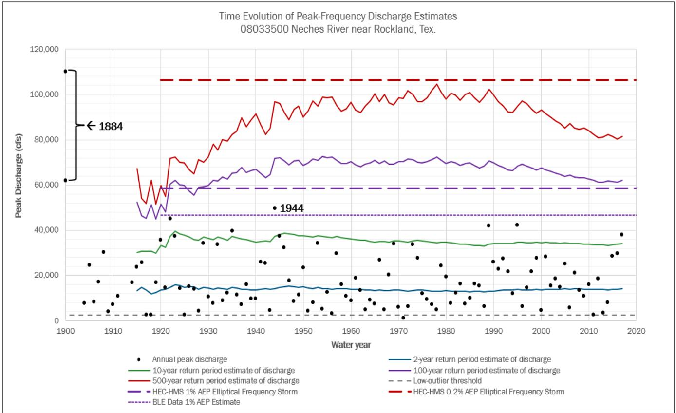
**Figure 11.4b: Statistical Change Over Time Comparison for the Neches River nr Rockland, TX**
