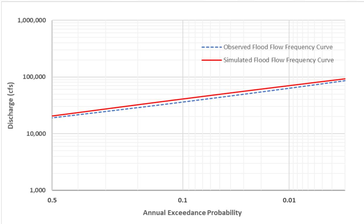
Figure 8.17: Comparison of Flood Flow Frequency Curves for the Observed and Simulated Datasets for USGS Streamgaging Station 08040600 Neches River near Town Bluff, Tex.
