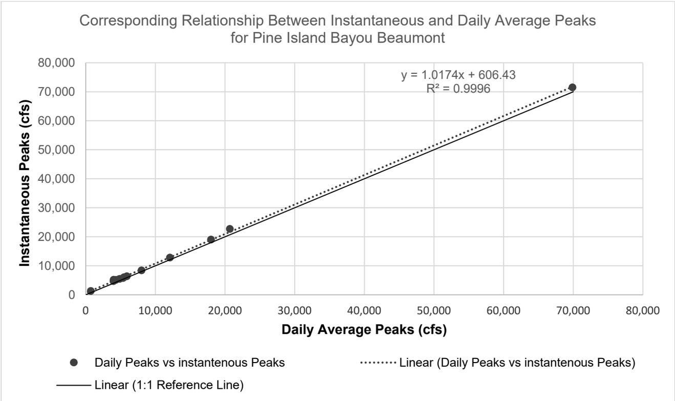
Figure 8.13: Instantaneous vs. Daily Average Peak Discharges for USGS Streamgaging Station 08041749 Pine Island Bayou above BI Pump at Beaumont, Tex.
