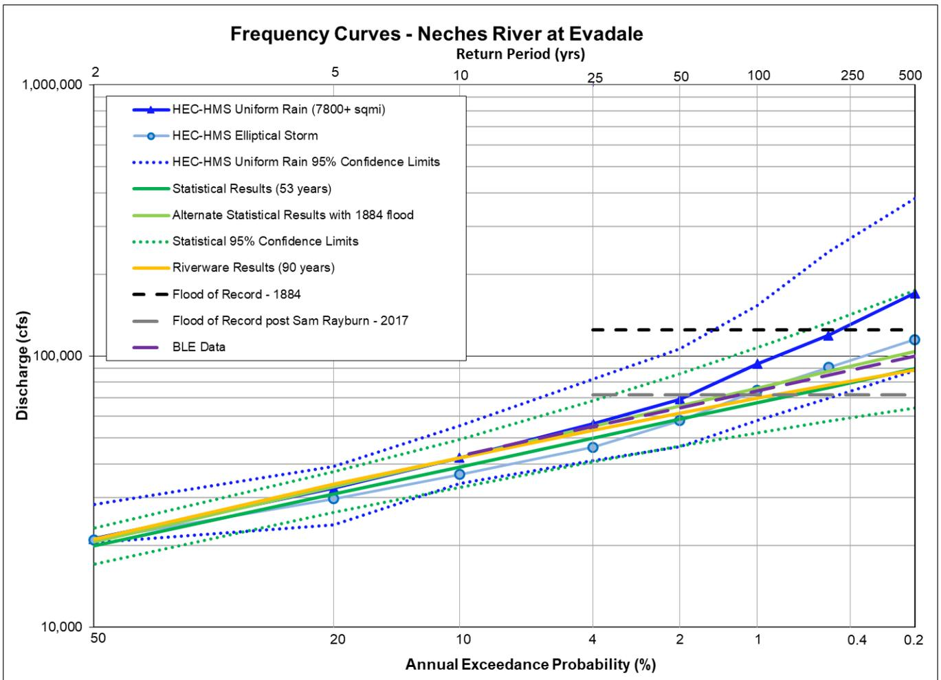
**Figure 11.12a: Flow Frequency Curve Comparison for the Neches River at Evadale, TX**
