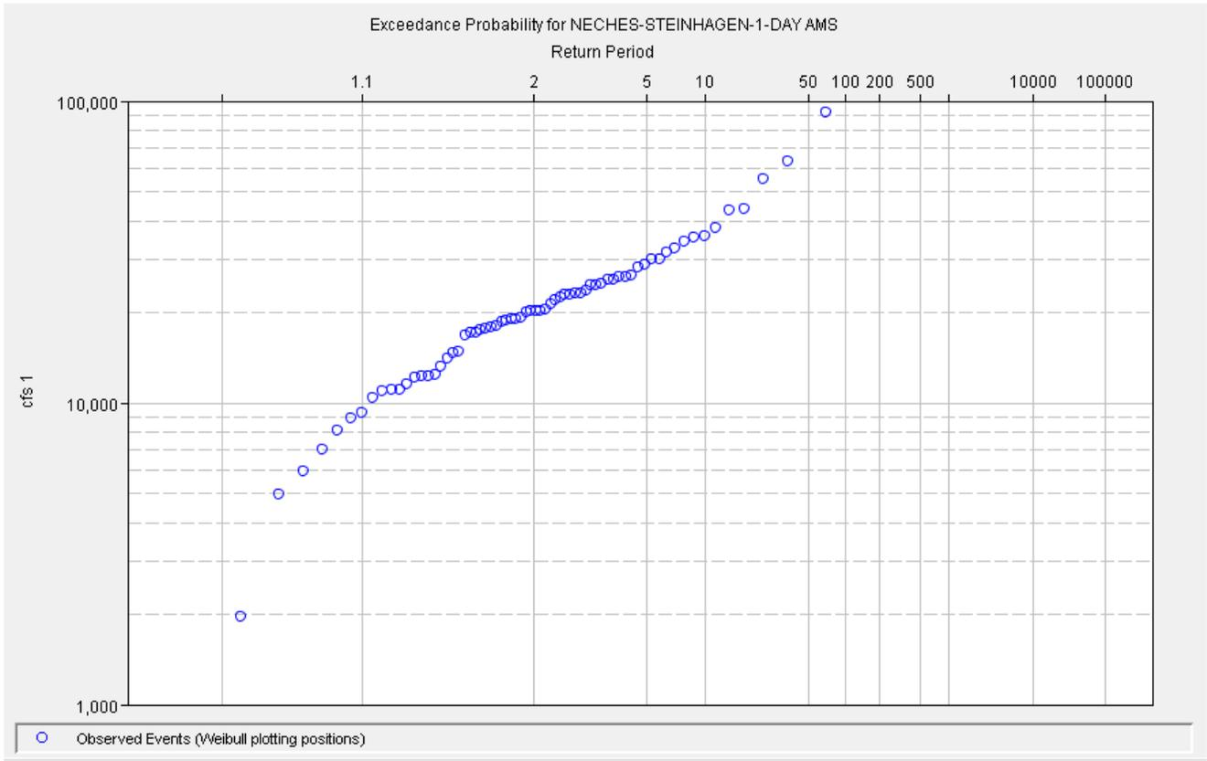
Figure 9.20: B.A. Steinhagen Observed Releases Following Weibull Plotting Distribution
