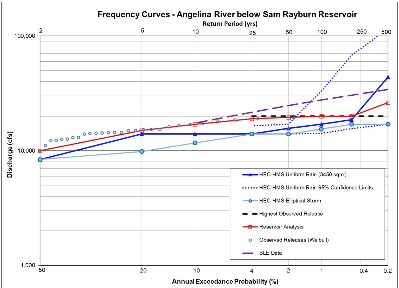
**Figure 11.10: Flow Frequency Curve Comparison for the Angelina River below Sam Rayburn Dam**
