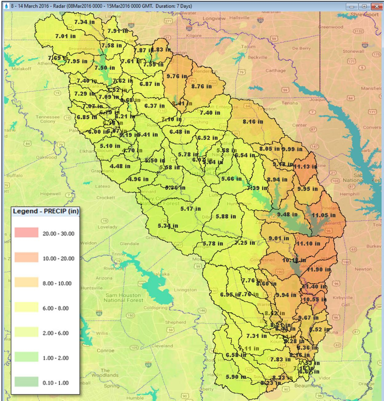
Figure 6.7: Total Rainfall Depths (inches) for the Mar 2016 Calibration Storm
