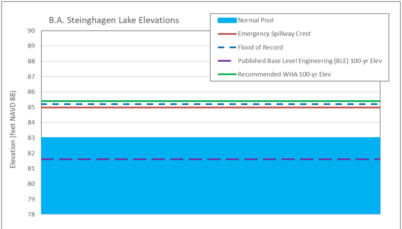
Figure 13.4: Comparison of Pool Elevations for B.A. Steinghagen Lake
