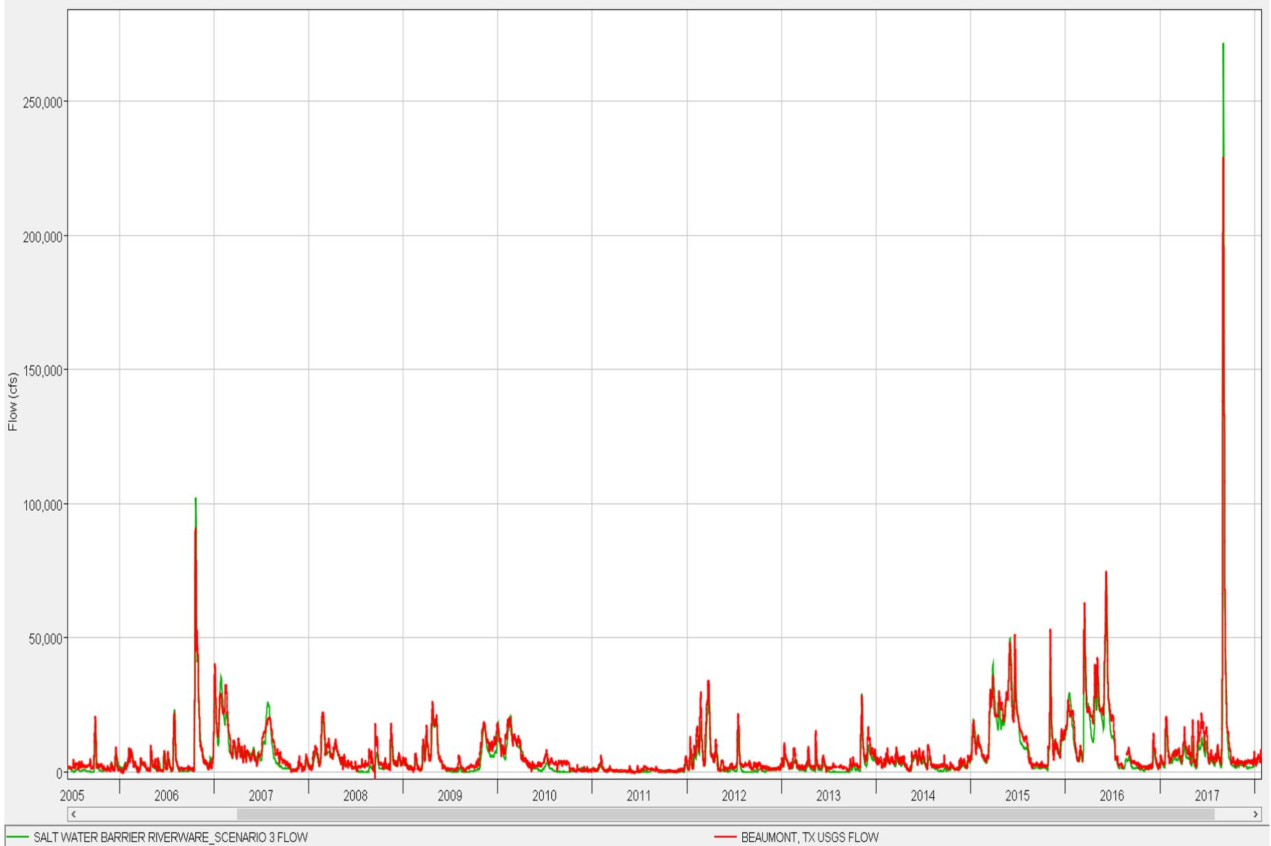
Figure 8.7: RiverWare Model Results Comparison for USGS Streamgauge Station 08041780 Neches River Saltwater Barrier at Beaumont, Tex.
