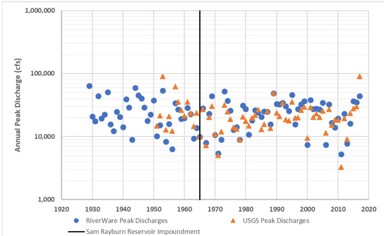
**Figure 8.15: Simulated RiverWare and Observed USGS Annual Peak Discharges for USGS Streamgaging Station 08040600 Neches River near Town Bluff, Tex.**
