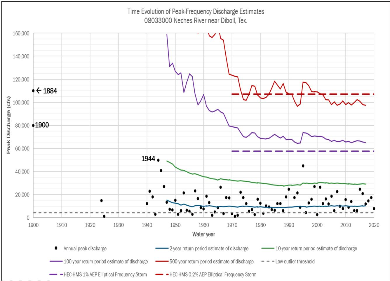
**Figure 11.3b: Statistical Change Over Time Comparison for the Neches River nr Diboll, TX**
