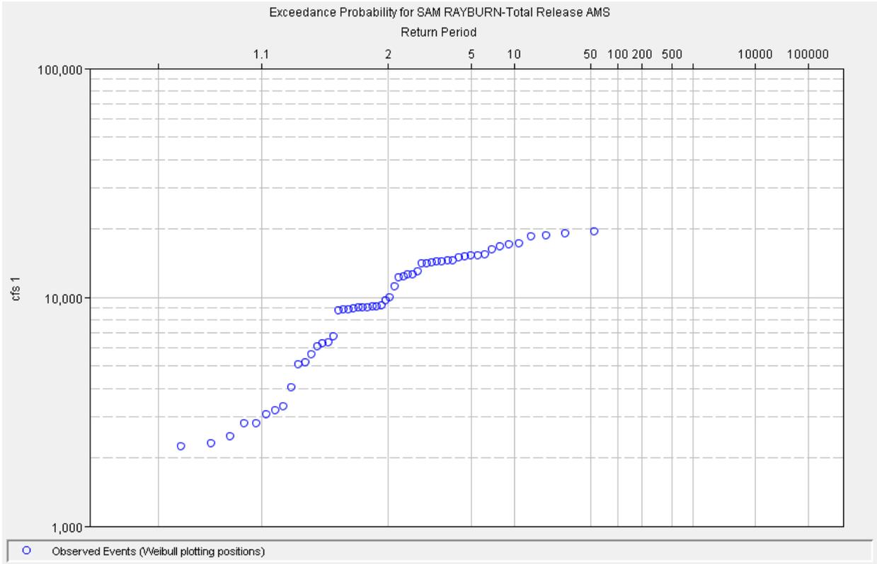
Figure 9.18: Sam Rayburn Observed Releases Following Weibull Plotting Distribution
