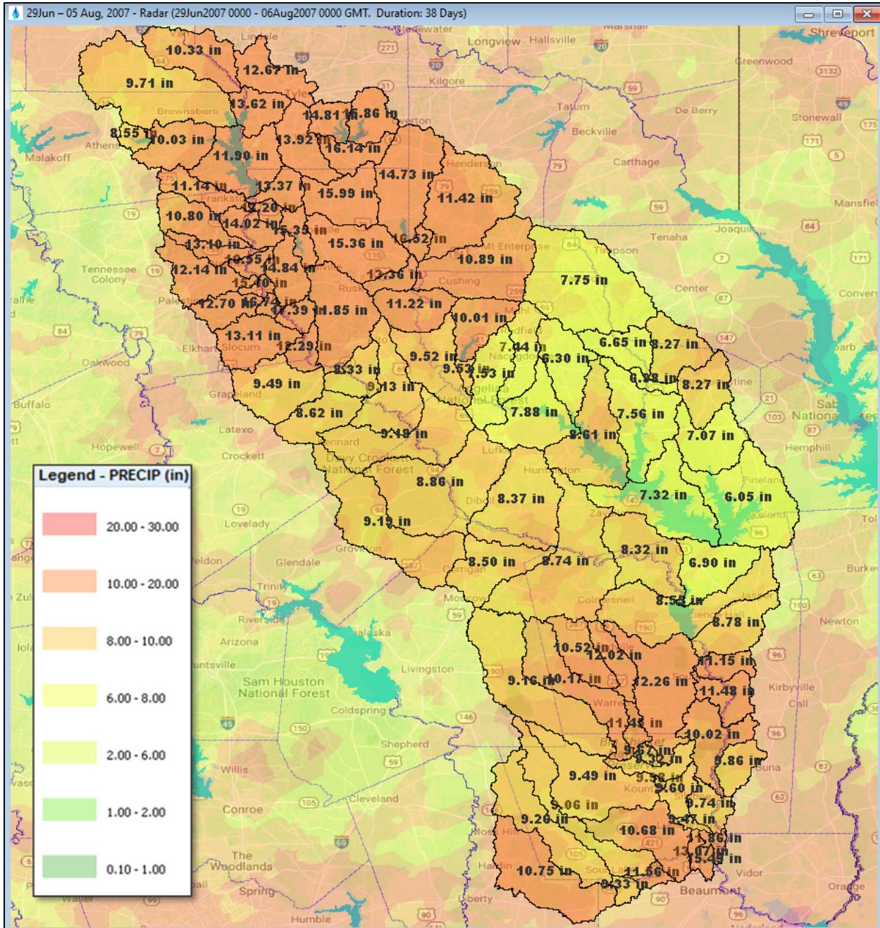
Figure 6.5: Total Rainfall Depths (inches) for the Jun-Jul 2007 Calibration Storm
