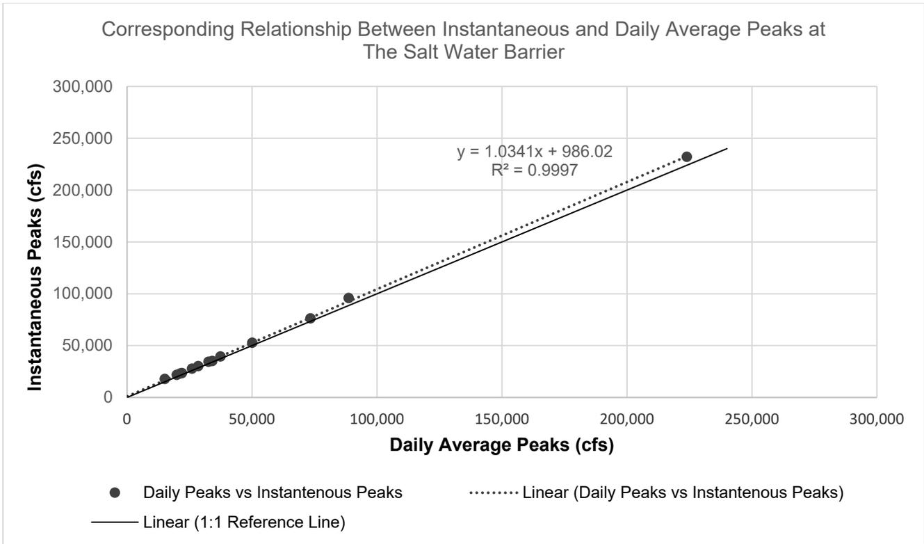
**Figure 8.14: Instantaneous vs. Daily Average Peak Discharges for USGS Streamgaging Station 08041780 Neches Rv Saltwater Barrier at Beaumont, Tex.**
