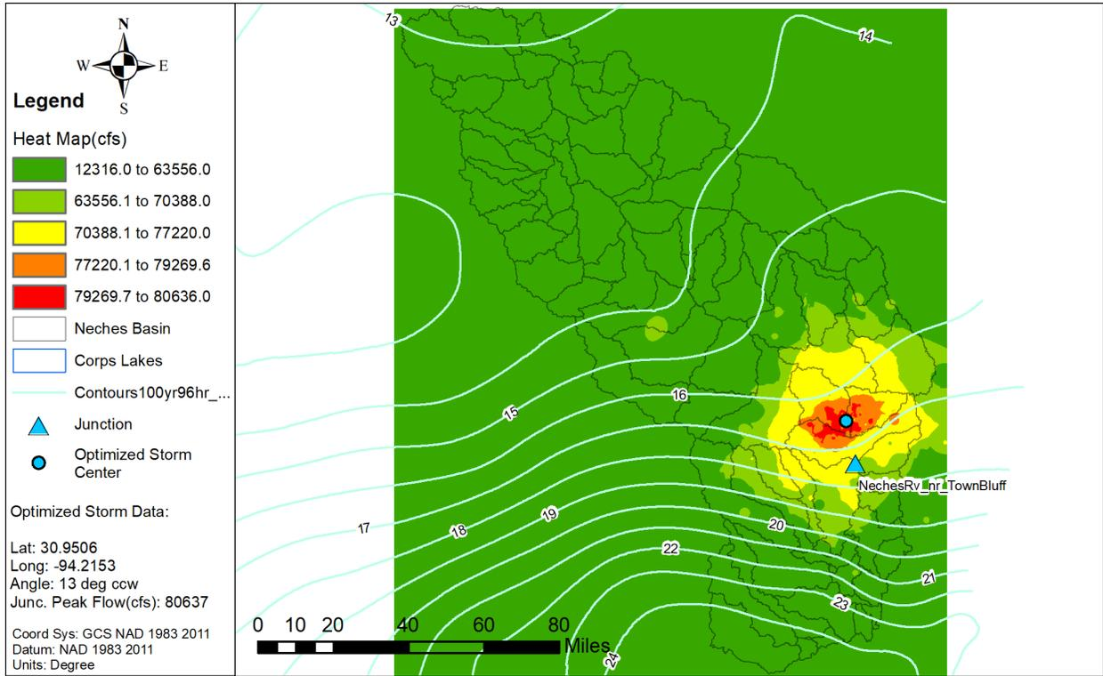
Figure 7.13a: Elliptical Storm Optimization Heat Map for NechesRv\_nr\_TownBluff
