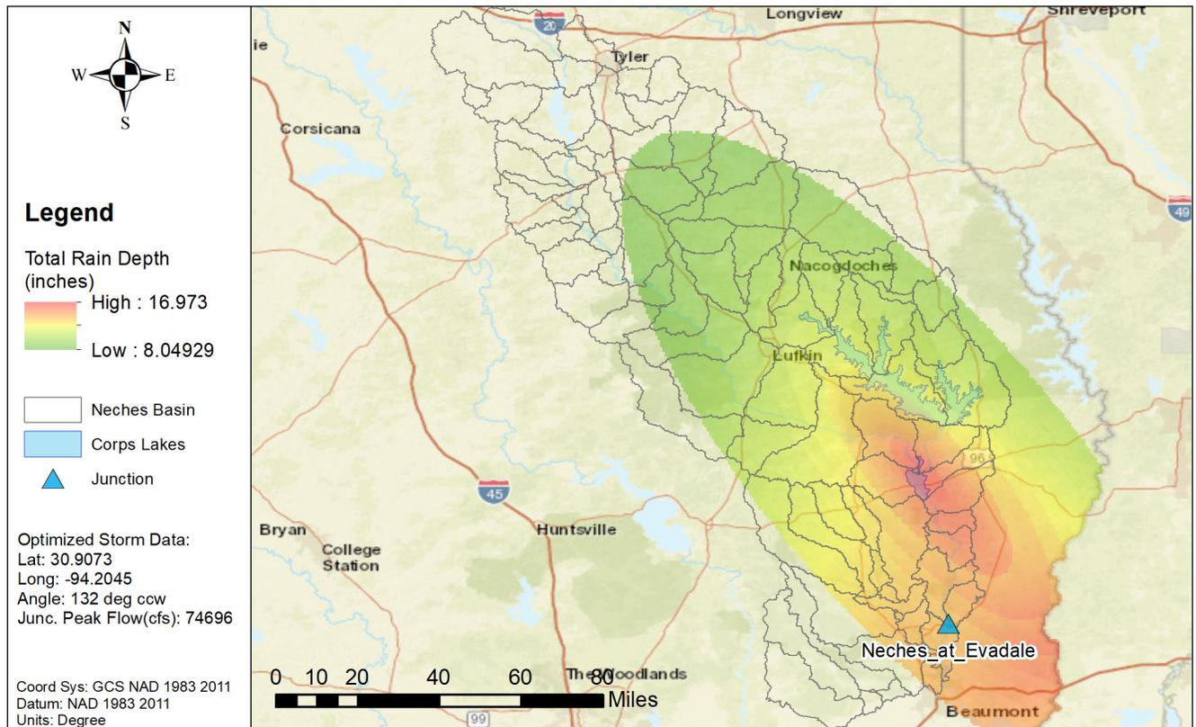
Figure 7.14b: NA14 1% AEP Elliptical Storm for Neches\_at\_Evadale
