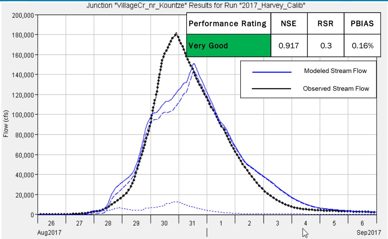
Figure 6.17: Aug 2017 Calibration Results for the Village Creek nr Kountze, TX USGS Gage
