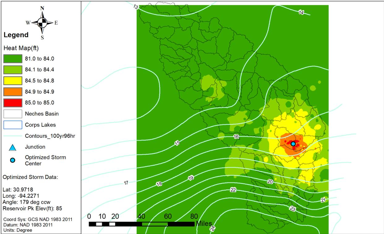
Figure 7.19a: Elliptical Storm Optimization Heat Map for B.A. Steinhagen Lake
