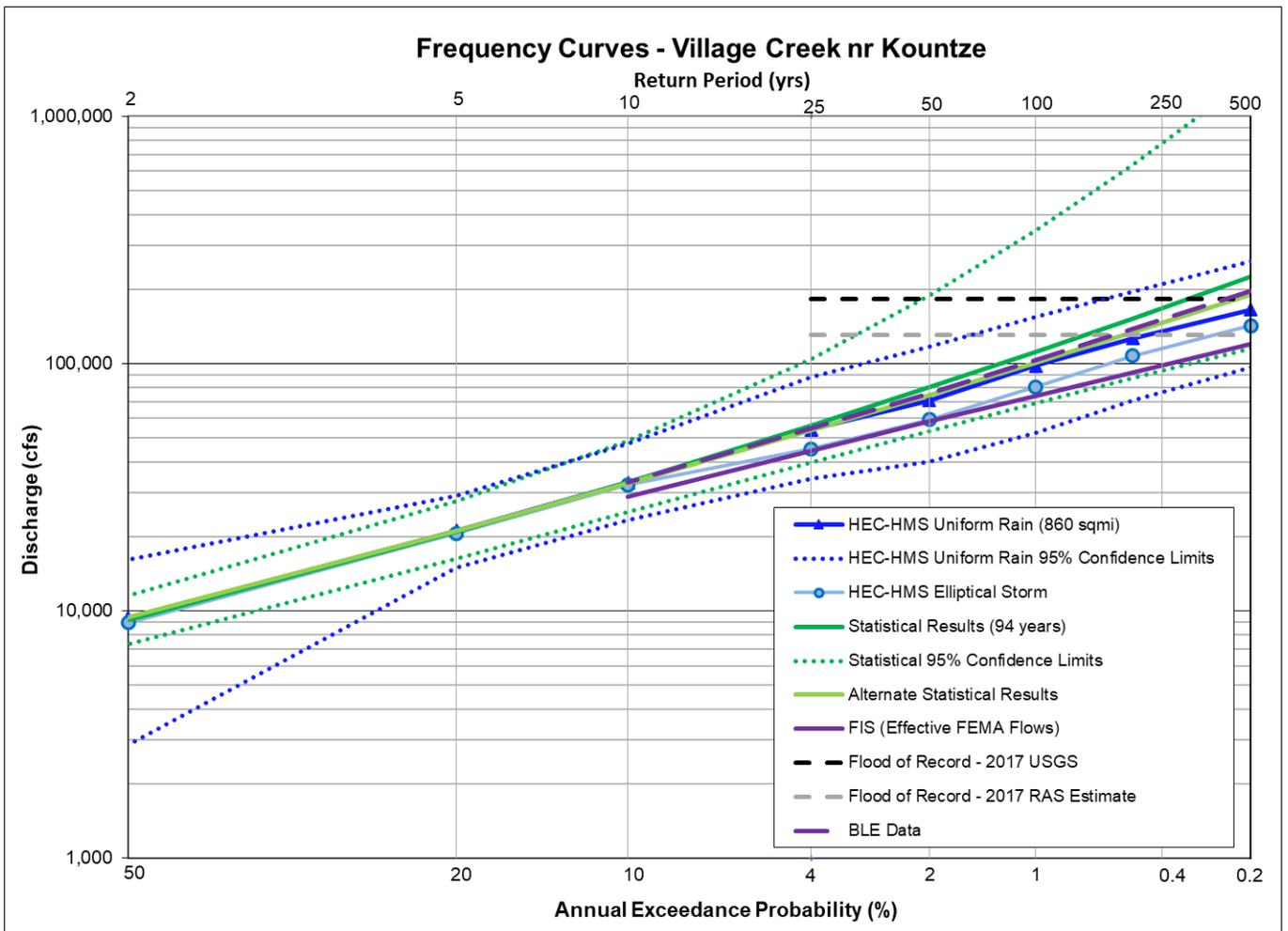
**Figure 11.13a: Flow Frequency Curve Comparison for Village Creek near Kountze, TX**
