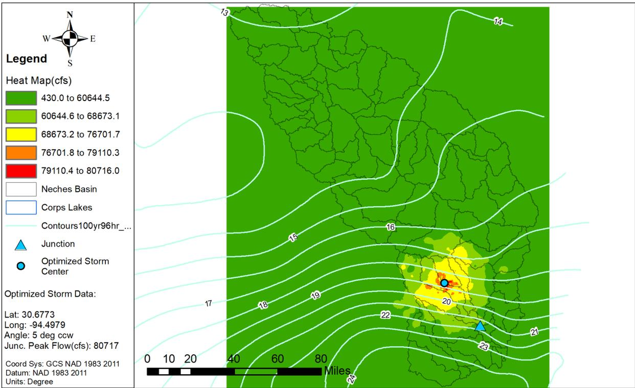
Figure 7.15a: Elliptical Storm Optimization Heat Map for VillageCr\_nr\_Kountze
