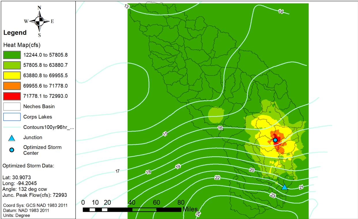
Figure 7.14a: Elliptical Storm Optimization Heat Map for Neches\_at\_Evadale
