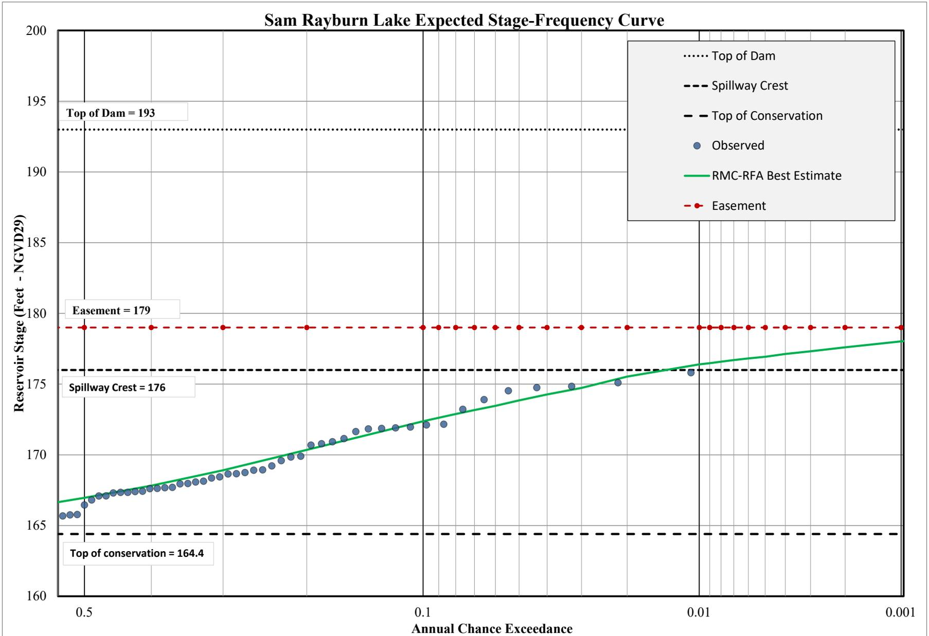
Figure 9.19: Sam Rayburn Reservoir RMC-RFA Final Stage-Frequency Curve
