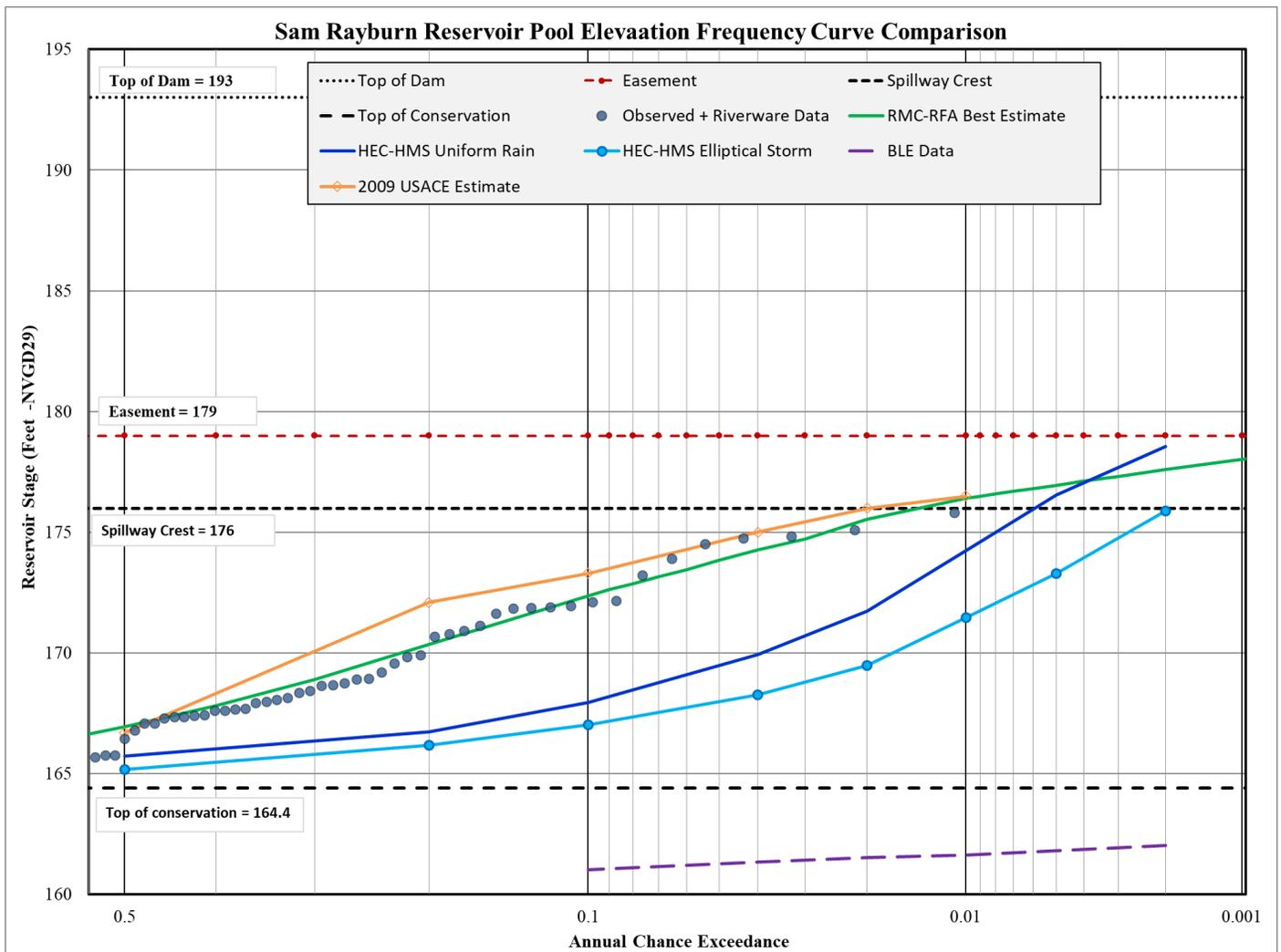
**Figure 11.17: Pool Elevation Frequency Curve Comparison for Sam Rayburn Reservoir**
