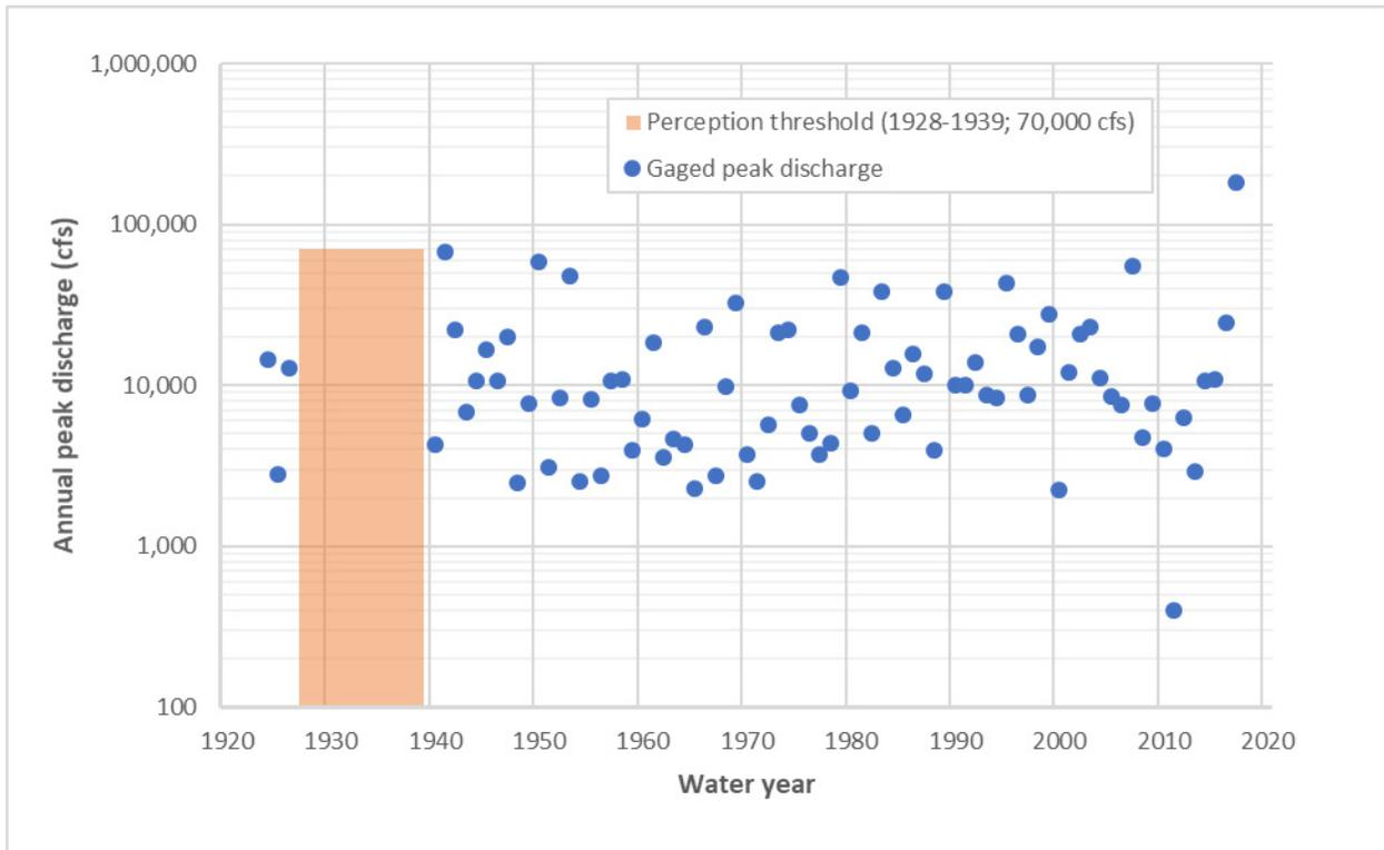
Figure 5.11: Annual Peak Discharge Data for USGS Station 08041500 Village Creek near Kountze, Tex.
