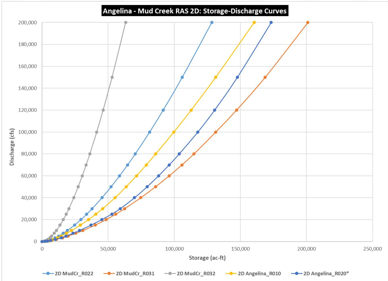
Figure 10.13: 2D HEC-RAS Storage-Discharge Curves
