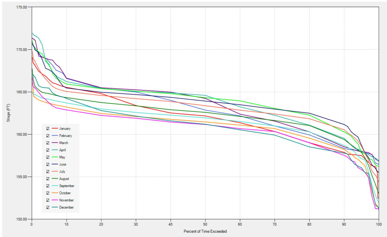
Figure 9.10: Sam Rayburn Reservoir Starting Stage Durations
