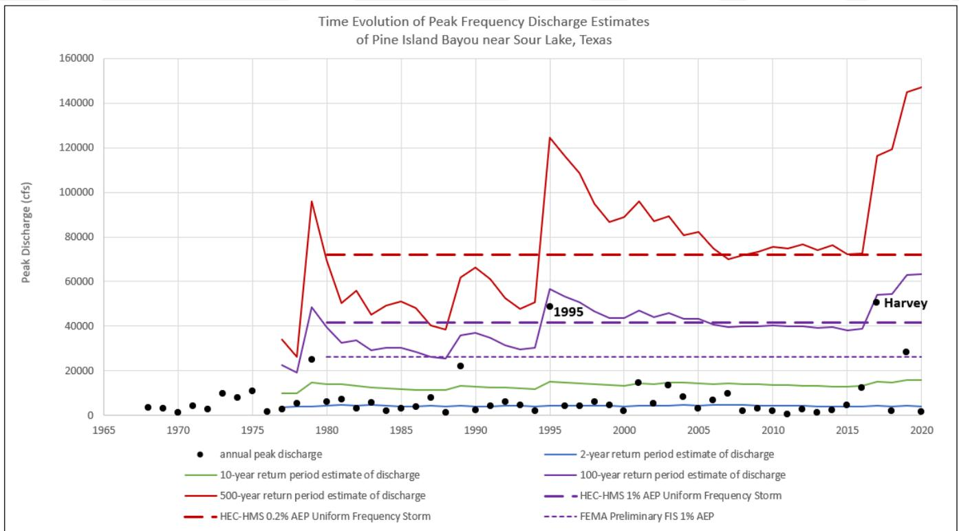
**Figure 11.14b: Statistical Change Over Time Comparison for Pine Island Bayou near Sour Lake, TX**
