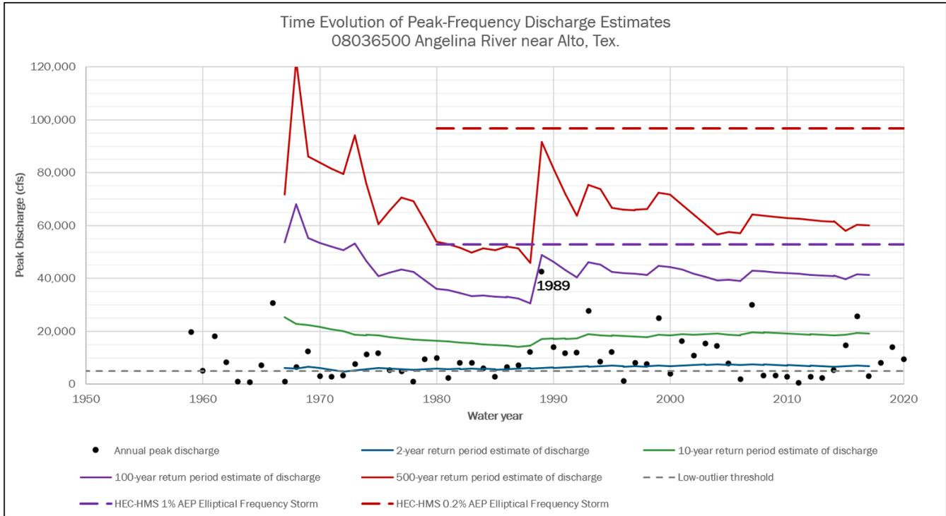
**Figure 11.6b: Statistical Change Over Time Comparison for the Angelina River nr Alto, TX**
