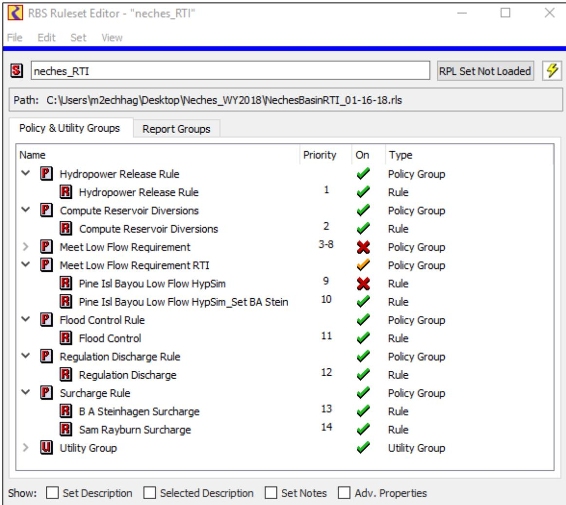
Figure 8.3: Neches River Basin Rule-based Simulation Groups
