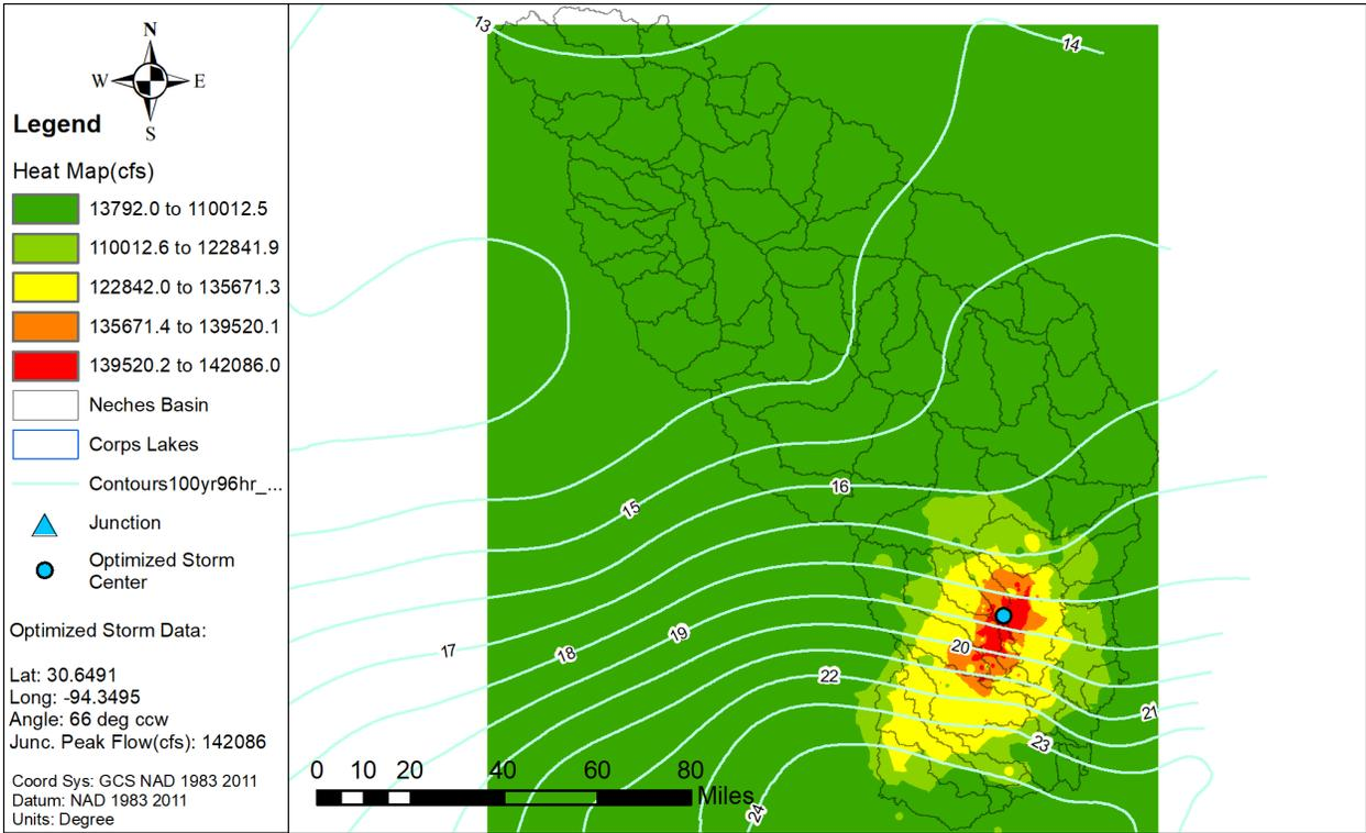
Figure 7.16a: Elliptical Storm Optimization Heat Map for Neches\_at\_SaltwaterBarrier
