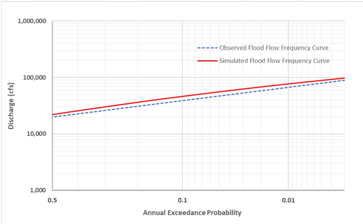
Figure 8.20: Comparison of Flood Flow Frequency Curves for the Observed and Simulated Datasets for USGS Streamgaging Station 08041000 Neches River at Evadale, Tex.
