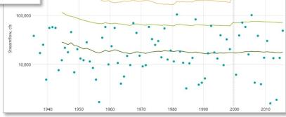
estimate is at a relative high point or low point. The change over time plots illustrate the relative instability of statistically based flood frequency estimates, especially for rare frequencies like the 100-yr flood, and demonstrate their susceptibility to new large flood events, climate variability, reservoir construction, or other physical changes to the basin. These plots also show that even with 100 years of gage record, the 100-yr flow estimate is still a moving target.
