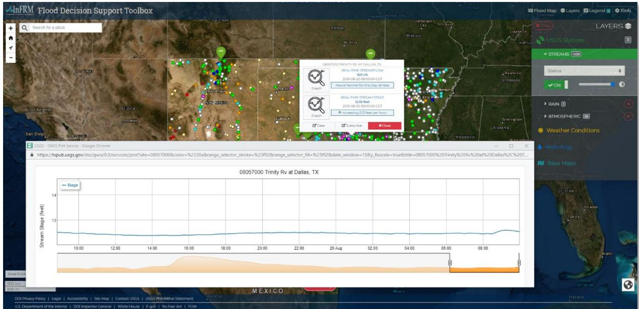
**Figure 12:** Example graph showing stage at USGS streamgage 08057000 Trinity River at Dallas, Texas.
