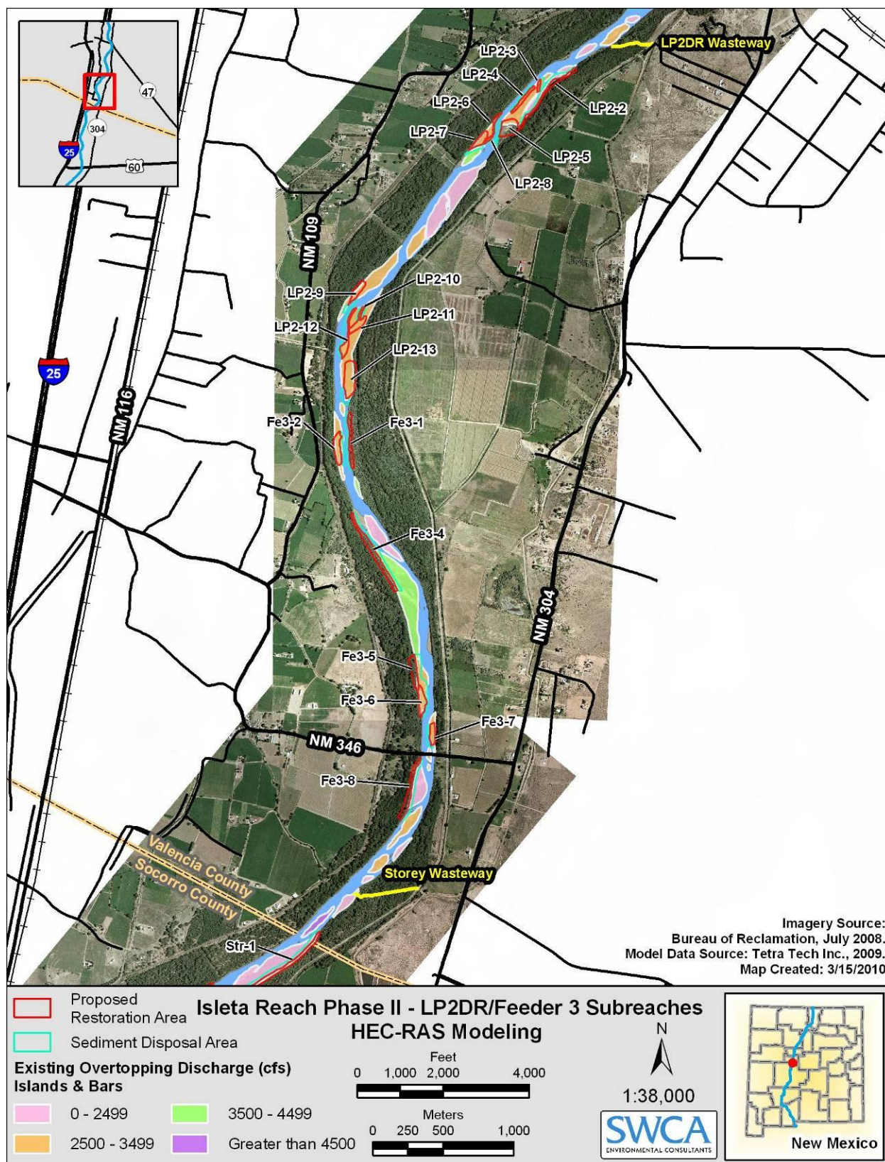
Figure B.2. LP2DR and Feeder 3 Subreaches HEC-RAS modeling with island/bar and restoration site delineation.
