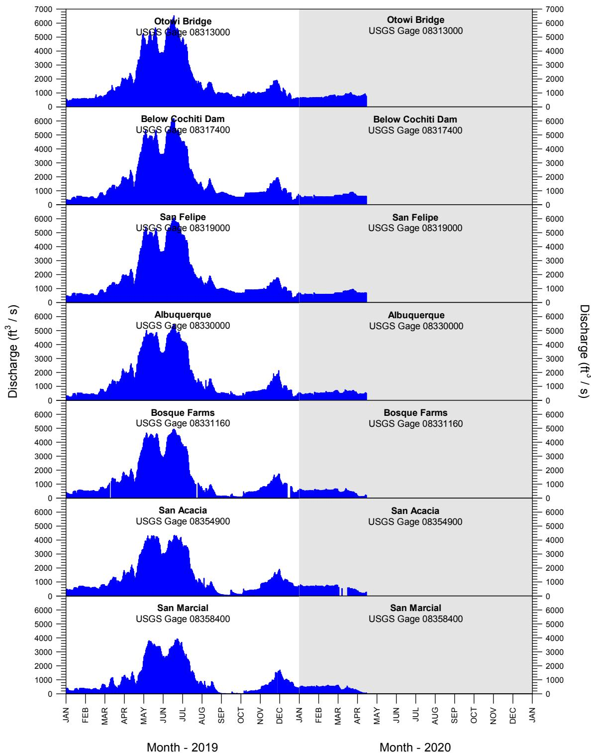
Figure 3. Rio Grande mean-daily discharge, by U.S. Geological Survey (USGS) gaging station, from 1 January 2019 to 15 April 2020. Discharge data are provisional and subject to change.
